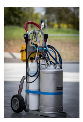
DA 2 is a mobile decontamination device designed for indoor and outdoor use, where access to the affected area is either restricted or where a robust rinse technique is avoided for subsequent damage. With a 4-fold decontaminant content in relation to DA 1, it allows to cope a larger contamination.
