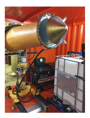
DA4 is a large-volume decontamination equipment designed to decontaminate the internal spaces of platforms and subway tunnels. It is a facility with sufficient decontaminant supply and allows rapid rinse and decontamination in the event of CBRN attack in the subway.
