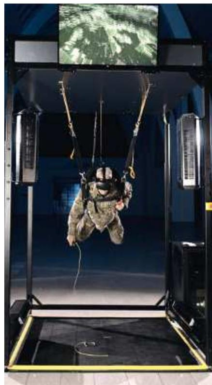
the experience of wind which is created by application of four wind modules, or the improved body tracking which allows tracking of hand movement to steer during the free fall phase more precisely. With the mounted Touch monitor, the instructor can change various exercise parameters during the running training.
