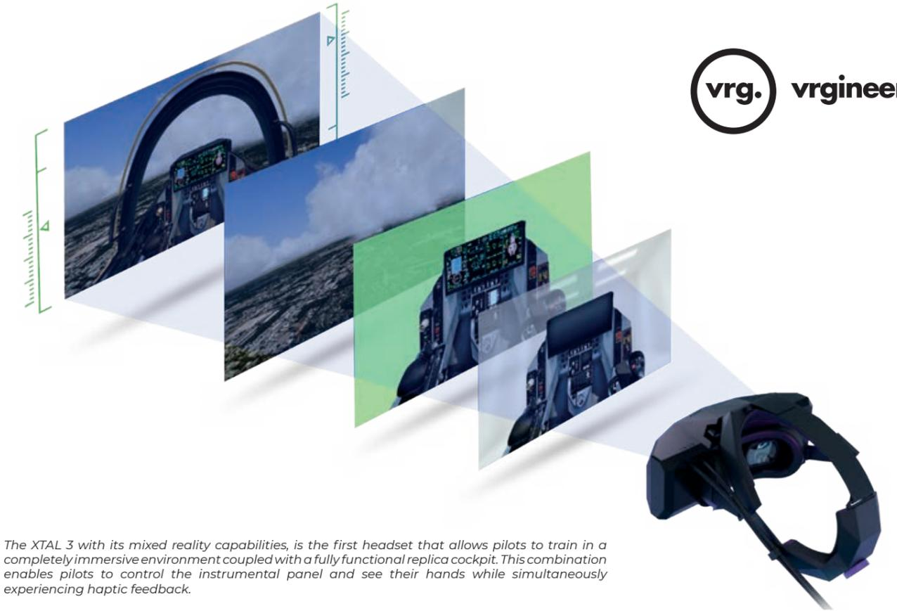
*The XTAL 3 with its mixed reality capabilities, is the first headset that allows pilots to train in a completely immersive environment coupled with a fully functional replica cockpit. This combination enables pilots to control the instrumental panel and see their hands while simultaneously experiencing haptic feedback.*
