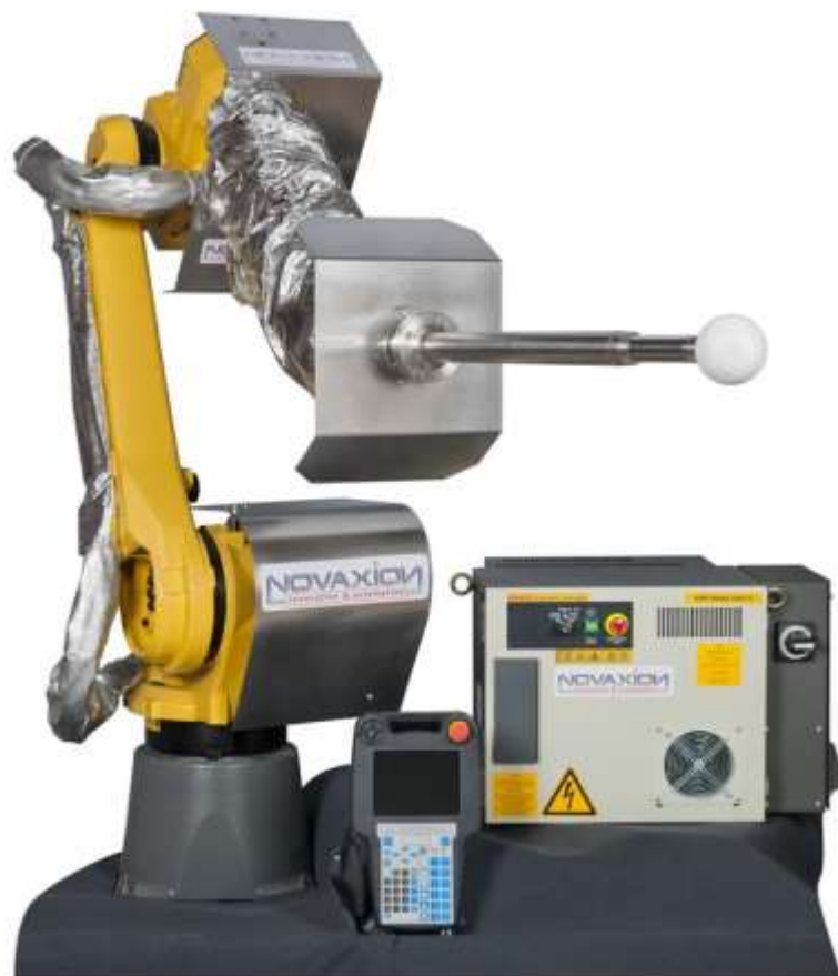
Fig. 8.13 Example of a ball-gatherer feeder (source: NOVAXION)
