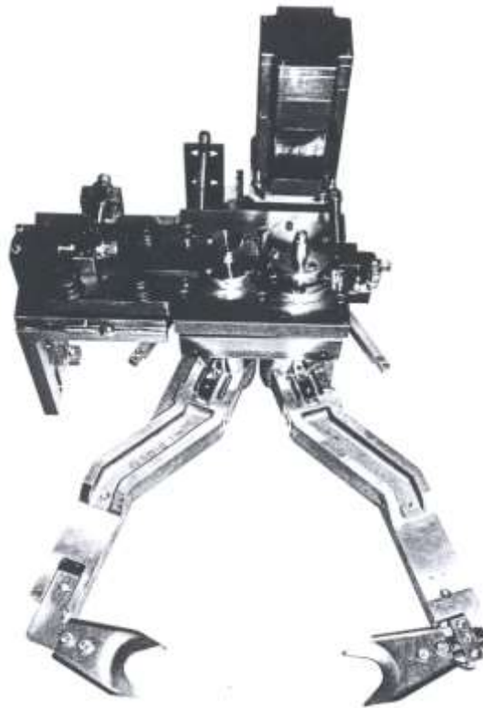
Fig. 8.10 Lever shears with servo drive (source: Walter)
