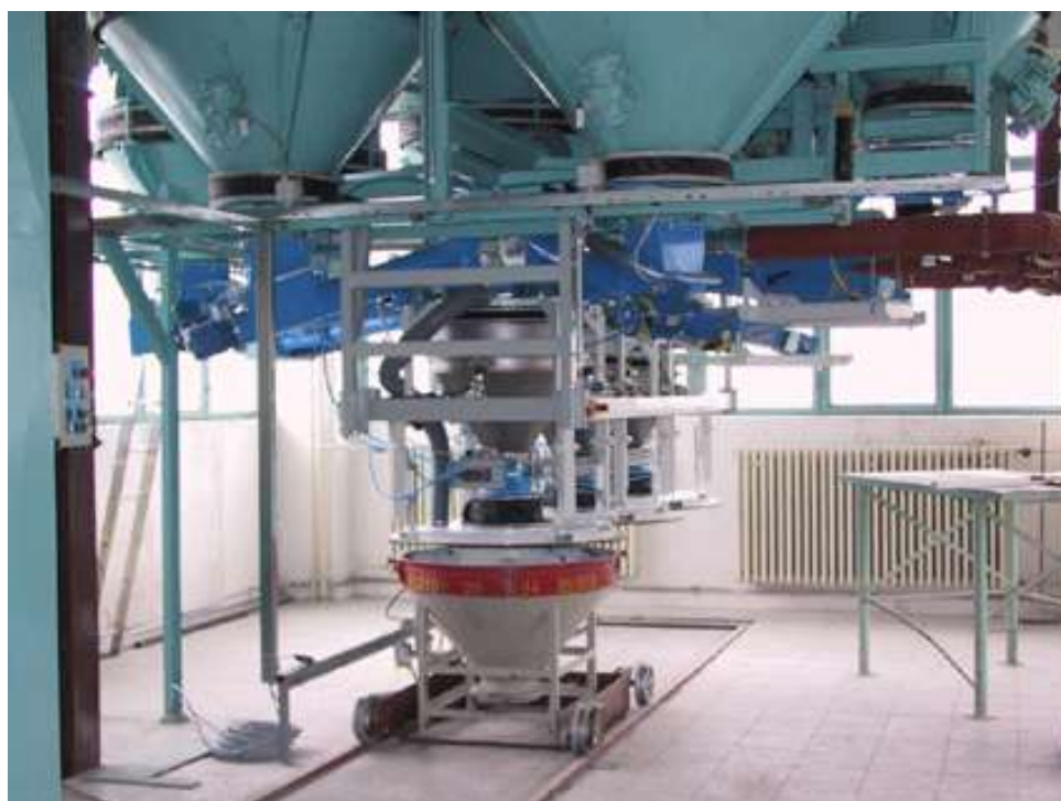
Fig. 5.3 View of the actual part of machinery of the batch house, the lower part of containers, raw material feeders, weigher, container (source: Dites spol. s r.o.)
