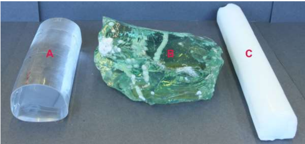
Fig. 3.8 Glass crystallization: A – clear glass pressing rod without visible crystallization, B – fragment of glass from a tank furnace with appreciable crystallization after heterogeneous nucleation, C - opal pressing rod with crystallisation after homogeneous nucleation
