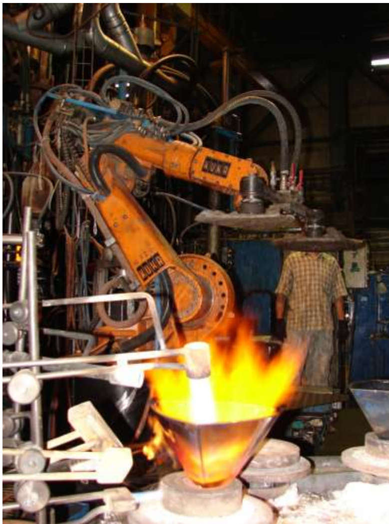
Fig. 11.29 Angular Kuka robot for handling in vase polishing
