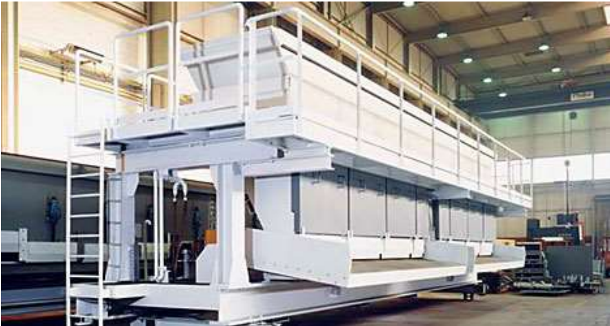
Fig. 6.5 Batch charger for large volumes of charge (source: Zimmermann-Jansen GmbH)
