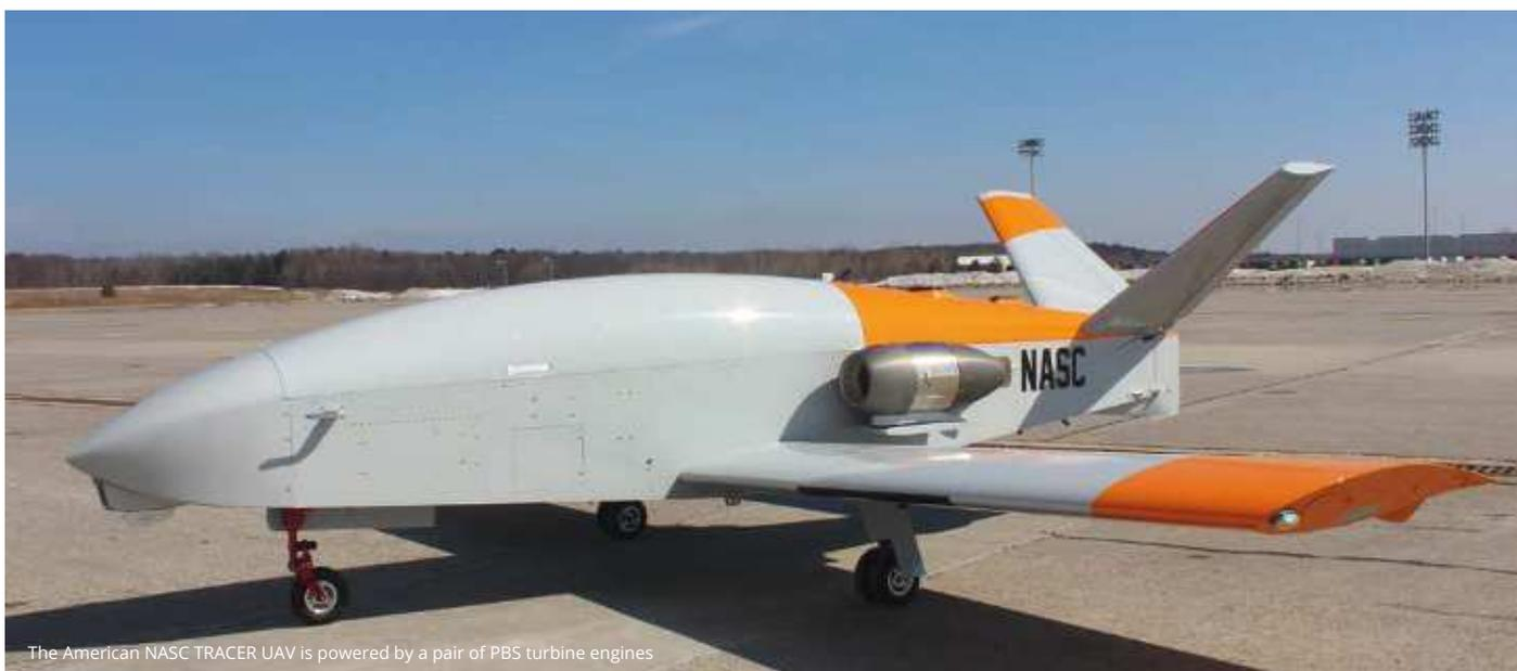
The American NASC TRACER UAV is powered by a pair of PBS turbine engines
