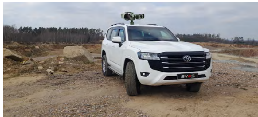
Armoured Toyota Land Cruiser with electro-optical surveillance system
