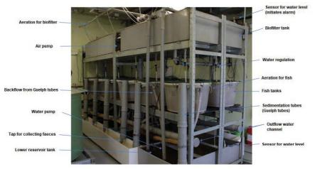
**Fig. 2.** Snapshot of our in-house Guelph system used for digestibility trials. (Photo: laboratory archive).
