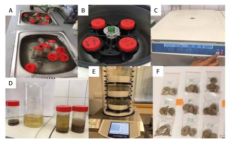
**Fig. 8.** Processing of collected faeces sample – **A:** thawing of frozen samples; **B** and **C:** centrifugation of thawed faeces; **D:** separation of water supernatant from faeces by decanting (after centrifugation); **E:** lyophilization of sedimented faeces; **F:** final faecal dry matterfor analysis. (Photo: laboratory archive).
