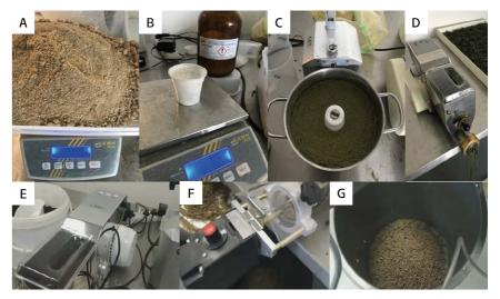
**Fig. 4.** Feed preparation – **A**: weighing of ingredients/feed; **B**: addition of marker; **C**: mixing with water to make dough; **D**: noodle maker machine (pelletizer); **E**: loading compartment of feed mix to pelletizer; **F**: motorized noodle cutter making pellets; **G**: final pellets. (Photos: laboratory archive).
