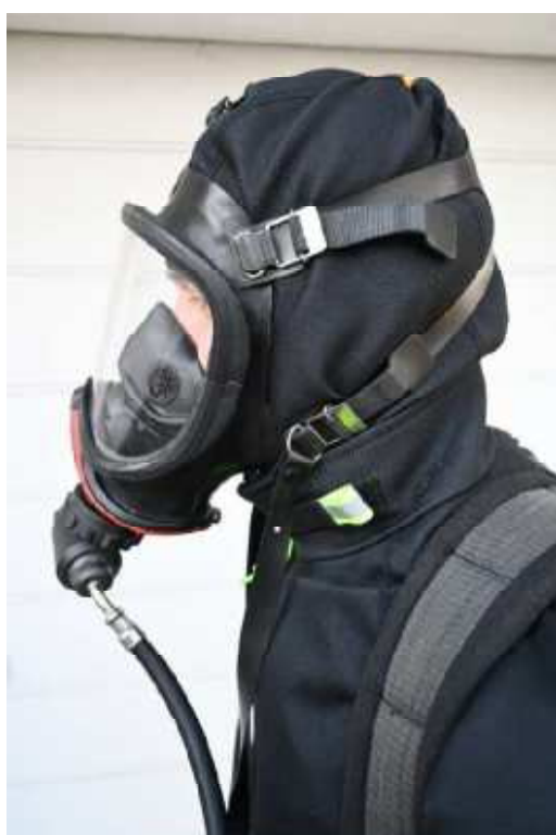
Adsorption carbon protective undergarment ActivSorb in combination with a breathing apparatus
