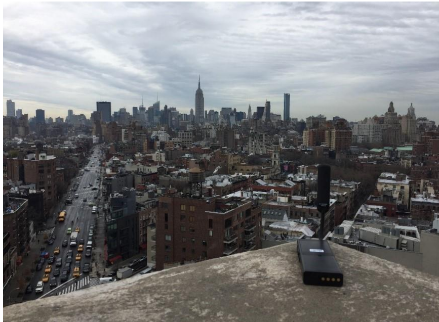
Figure 2-6 TW-400 CUB TSM Radio on Roof of NUSTL's Facility
