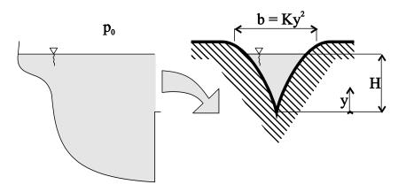
Determine the flow rate through an overflow weir, whose width is defined by the relation  $b = Ky^2$ , where the constant is  $K = 0.5 m^{-1}$ . Water level in the overflow weir is H = 0.9 m.
