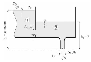
Water flows from tank 1, in which there is an opening with a size  $A_1 = 0.01 m^2$ , into tank 2. From here, water flows out through an opening with a size  $A_2 = 0.02 m^2$  into the surrounding atmosphere. Calculate the mass flow rate of water through tanks and the height  $h_2$ , at which water stabilises in tank 2. The flow coefficients of openings are  $\mu_1 = 0.6$  or  $\mu_2 = 0.91$ .
