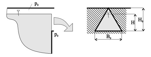
The fluid is located in a large tank (figure on the left) and flows out through a triangular opening (figure on the right). Calculate the volumetric flow rate of fluid through this triangular opening with a width  $B_0 = 4 m$  and a height  $H_0 = 2.3 m$  if fluid level from the base of the triangle is H = 1.85 m.
