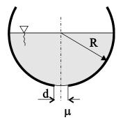
Calculate the time needed to empty a spherical vessel with a radius R = 1.3 m if water flows out through an opening with a diameter d = 60 mm. The initial fluid level in the tank is exactly in the centre of the sphere, i.e. the level is R. The discharge coefficient of the opening is  $\mu = 0.86$ .
