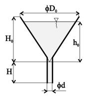
Calculate the time at which a conical vessel with a height  $H_0 = 3 m$  and a diameter  $D_0 = 1.8 m$  is emptied if filled with water up to a height  $h_0 = 2.3 m$  and with a tube with a length H = 1.3 m and a diameter d = 60 mm connected to the vessel. Neglect flow losses, neglect also the time needed to empty the connected tube.
