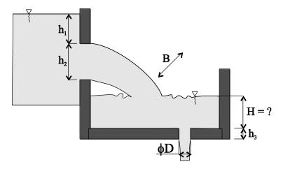
Determine the equilibrium water level in the lower tank into which the water flows through a rectangular opening with a width B = 1.3 m and a height  $h_2 = 0.7 m$  if water in the upper tank reaches a height  $h_1 = 0.96 m$  above the upper edge of the outlet drain. The diameter of the opening in the bottom of the lower tank is  $\phi D = 0.6 m$ , the wall thickness of the lower tank is  $h_3 = 22 cm$ . The upper opening is considered as large.
