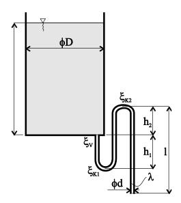
Calculate the time at which a vessel with a diameter D = 650 mm shown in the figure is emptied. The outlet drain is connected to a hose with a diameter d = 12.5 mm. Other dimensions are  $h_1 = 0.38 \text{ m}$ ,  $h_2 = 0.61 \text{ m}$ , l = 1.28 m. The original level is at a height H = 0.95 m. Consider local losses  $\xi_V = 0.5$ ,  $\xi_{K1} = 0.4$ ,  $\xi_{K2} = 0.6$  and the coefficient of friction  $\lambda = 0.03$ .
