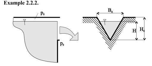
The fluid is located in a large tank (figure on the left) and flows out through a triangular opening (figure on the right). Calculate the volumetric flow rate of fluid through this triangular opening with a width  $B_0 = 3 m$  and a height  $H_0 = 2.8 m$  if fluid level from the top of the triangle is H = 1.9 m.
