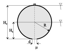
Calculate the time at which the level drops in a spherical tank shown in the figure from the initial height  $H_0 = 2R$  to the final height  $H_k = R$ . The spherical tank has a radius R = 3 m, fluid flows out through an opening with a diameter d = 100 mm with a discharge coefficient  $\mu = 0.67$ .
