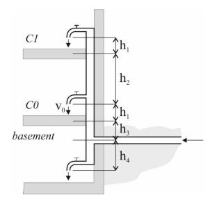
Water emerges from the tap in the classroom C0 (ground floor of building C in the figure) at a maximum velocity  $v_0 = 18 m s^{-1}$ . Determine the maximum velocity at which water emerges in the classroom C1 and in the basement. Different heights are  $h_1 = 1.2 m$ ,  $h_2 = 3 m$ ,  $h_3 = 1.8 m$  and  $h_4 = 1.5 m$ .
