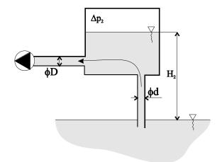
Calculate the volumetric flow of the water sucked in by the pump shown in the figure, if the pipe diameter is D = 100 mm, d = 64 mm, water level is  $H_2 = 2 \text{ m}$  and tank vacuum is  $\Delta p_2 = 25 \text{ kPa}$ .
