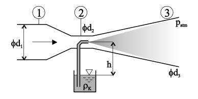
The airbrush shown in the figure sucks in the fluid with a density  $\rho_k = 800 \ kg \ m^{-3}$  from the container. Calculate the minimum air velocity at point (1), at which the fluid is sucked. The values are as follows:  $d_1 = 12 \ mm$ ,  $d_2 = 6 \ mm$ ,  $d_3 = 16 \ mm$ ,  $h = 8 \ cm$  and air density  $\rho = 1.2 \ kg \ m^{-3}$ .
