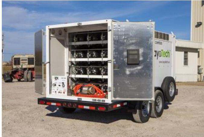
Figure 2: Example of mobile hydrogen storage.
