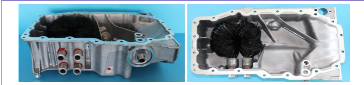
Figure 7: Hollow Fiber plastic oil heat exchanger for immersion cooling [5]
