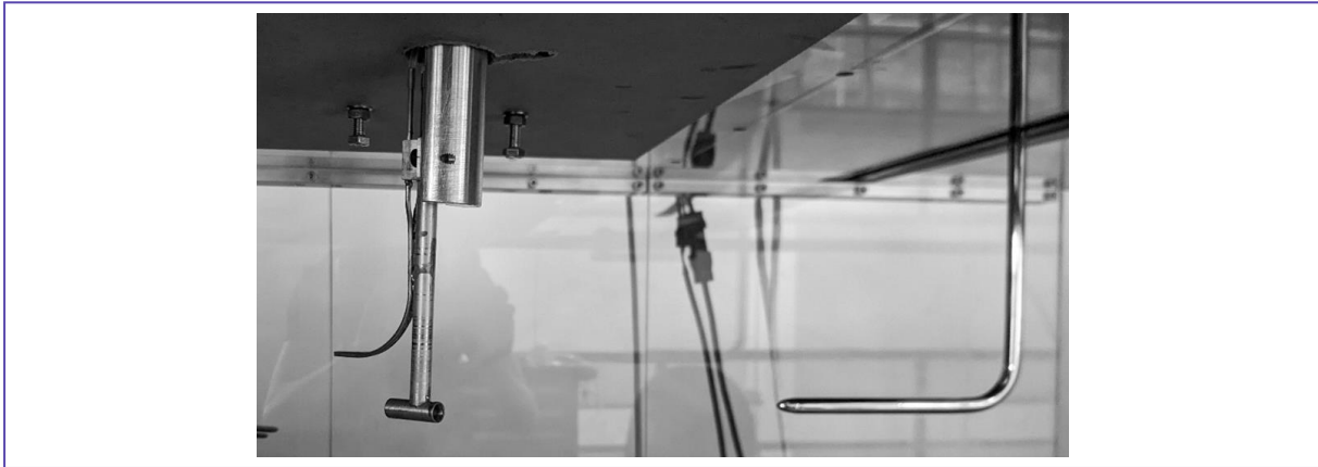
Figure 3: Probe during calibration and tunnel pitot tube at right side
