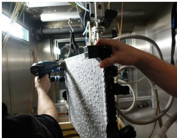
Figure 19: Filled heat exchanger bottom side with icicles
