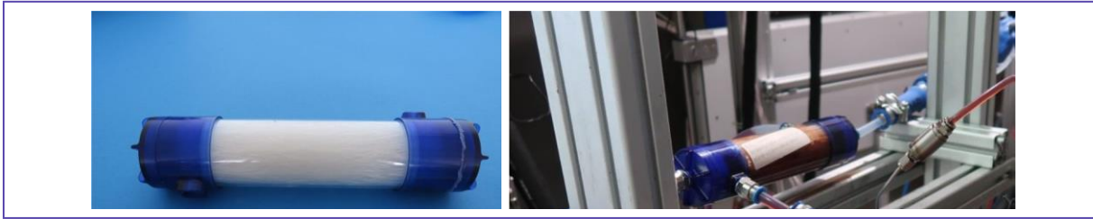
Figure 6: Oil to coolant heat exchanger with polyamid hollow fibers [4], [7]
