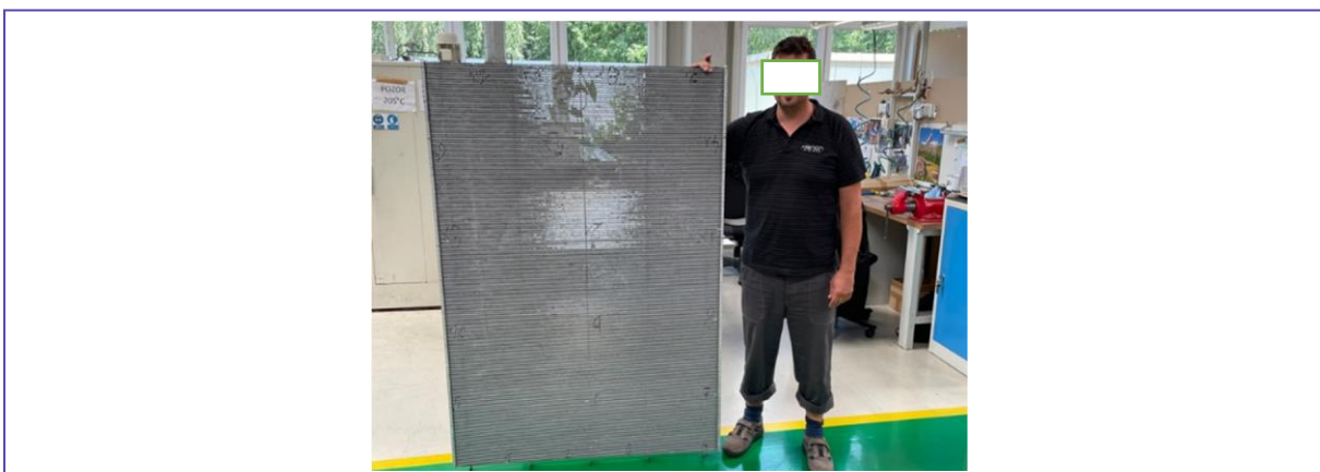
Figure 11: Aluminium brazed tube-fin heat exchanger for indirect immersion cooling, full size of approx. 1200 x 1600 mm, 10,8mm thickness [6]
