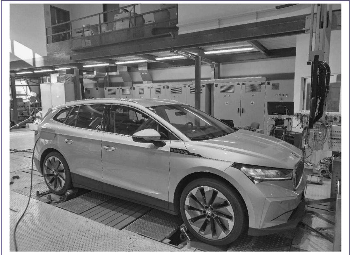
Figure 1: The tested Škoda Enyaq - electric vehicle on the BR4VDM chassis dynamometer located at Mendel University in Brno (Source: author)
