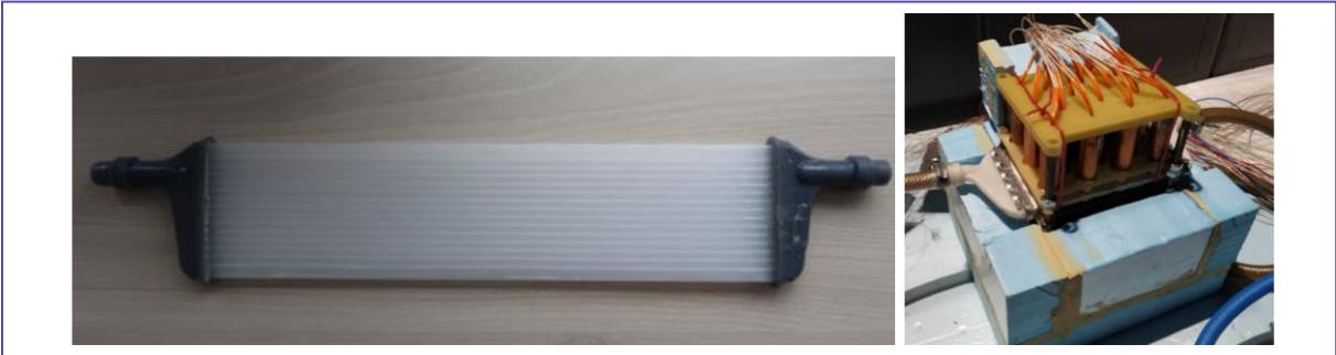
Figure 4: Extruded plastic heat exchanger for cylindrical cells [6]
