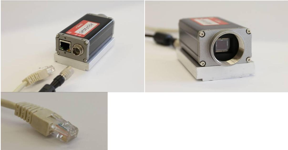
*Fig. 3.3 Camera with area sensor and GigE connector*
