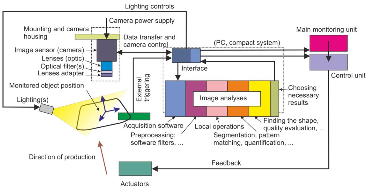
*Fig. 1.11 Diagram of the vision system*
