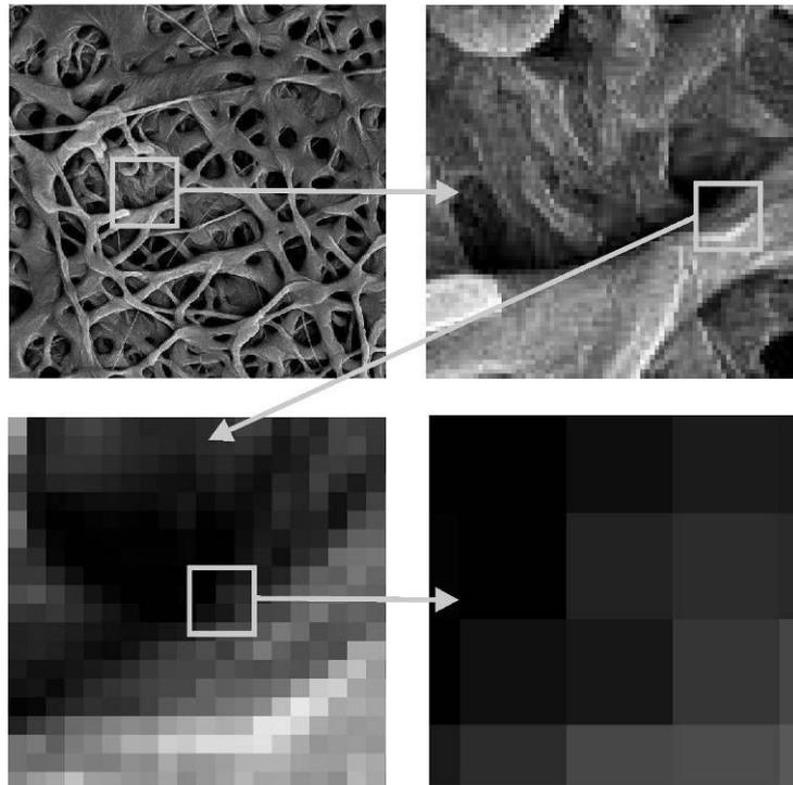
*Fig. 1.10 Magnification of part of digital image up to an apparent matrix of points (pixels)*
