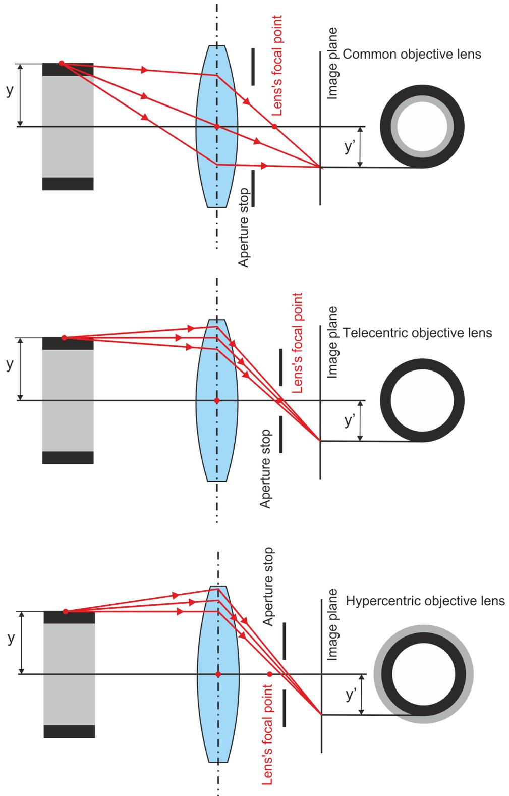
*Fig. 4.6 Difference in scanning by means of normal, telecentric and hypercentric objective lens*
