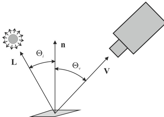
Fig. 1.8 Description of direction vectors towards the light source and observing element
