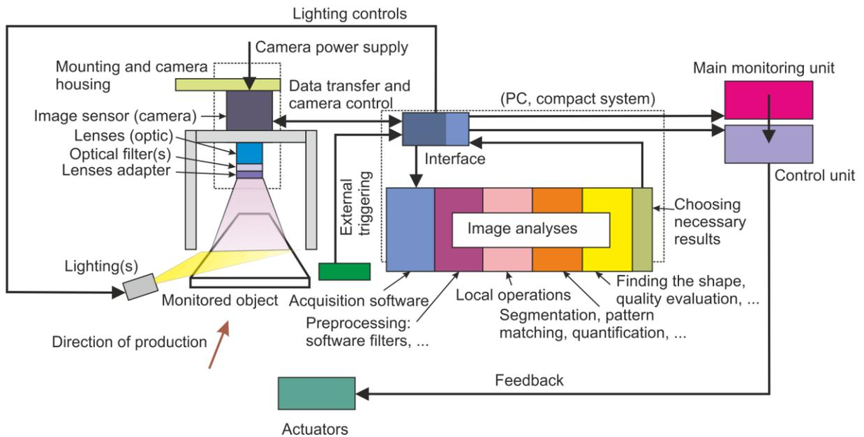
Fig. 3.6 Diagram of a system with line scan camera
