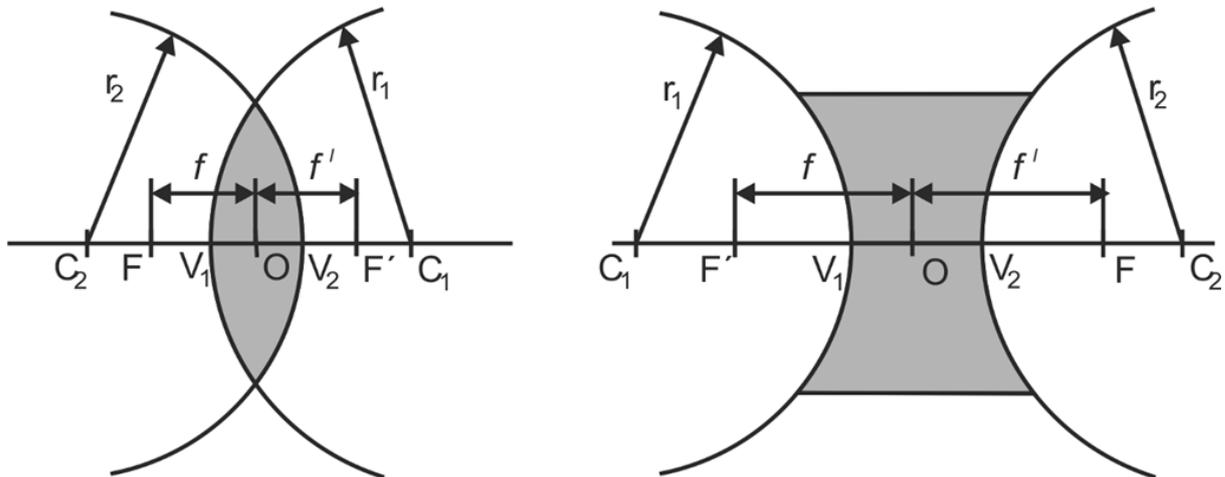
Fig. 4.2 Parameters of negative lens and positive lens
