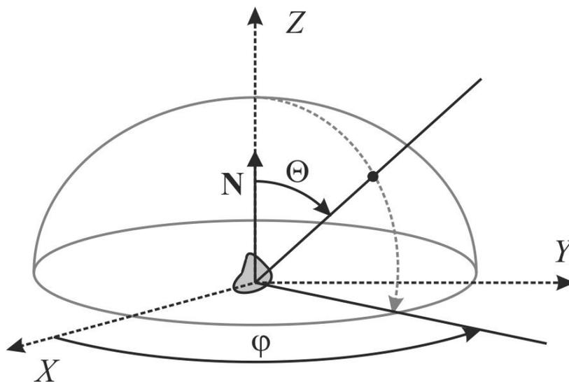
Fig. 1.9 Description of spot orientation in a spherical coordinate system
