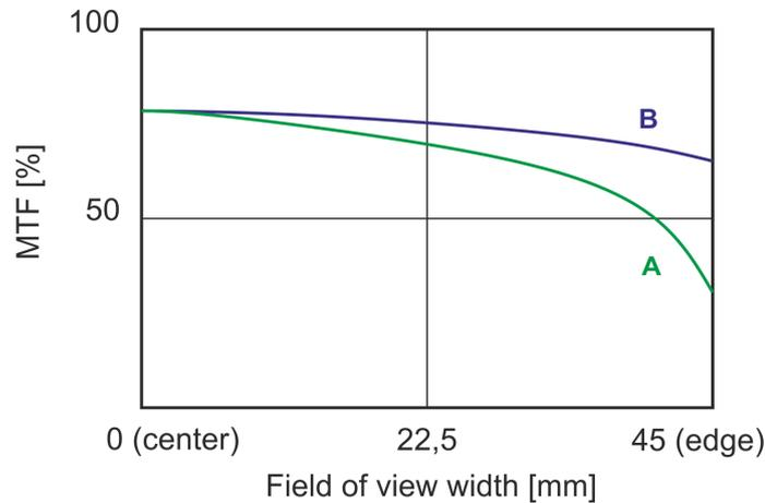
*Fig. 4.5 The MTF (modular transfer function) characteristics, A – common objective lenses, B – example of special high quality objective lenses; accurate MTF curve also depends on working distance and aperture value; the parameters are distinguished separately for radial and tangential direction*
