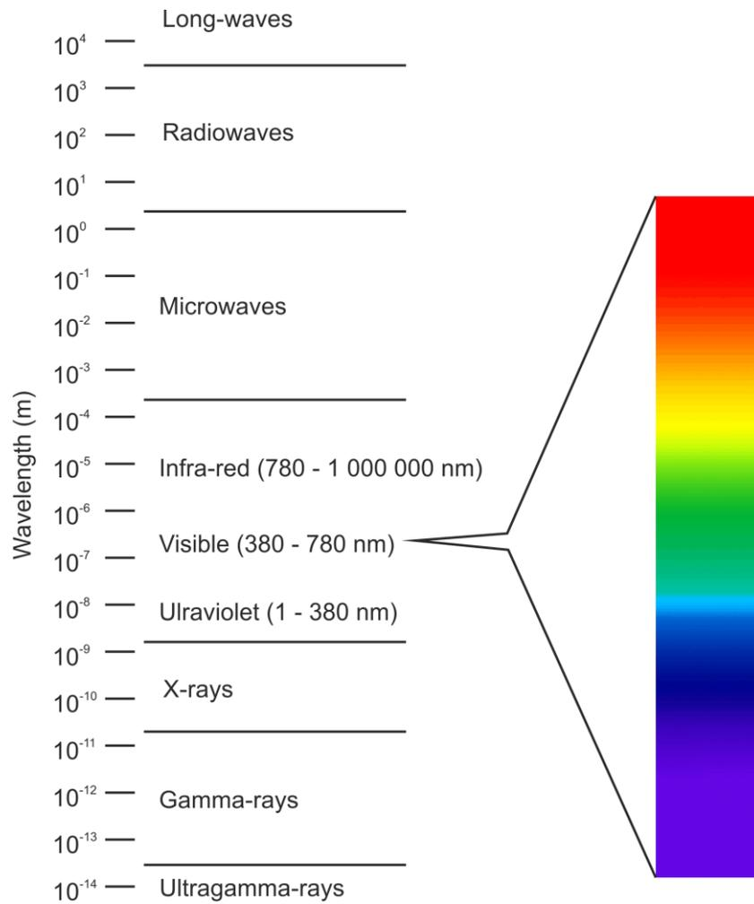
*Fig. 1.1 Electromagnetic radiation and display of coloured light spectrum*
