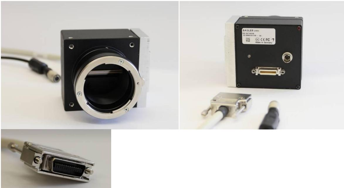
*Fig. 3.4 Line scan camera and Camera Link connector*
