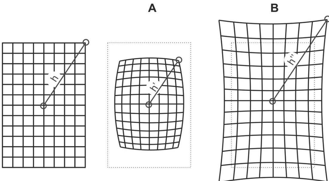
*Fig. 4.4 Basic types of radial distortion objective lens, A – barrel distortion, B – pincushion distortion*
