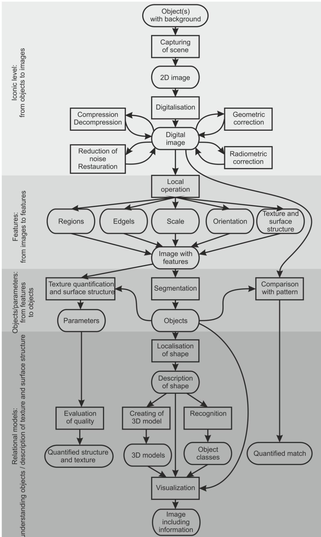
Fig. 1.4 Hierarchy of image processing tasks, is based on [2]
