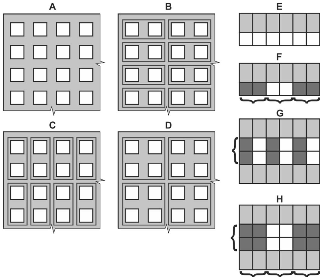
*Fig. 2.9 Pixel binning – principle of merging neighbouring pixels: A - area sensor without merging neighbouring pixels, B – area sensor with horizontal merging, C – area sensor with vertical merging, D – area sensor with horizontal and vertical merging, E – line sensor without merging neighbouring pixels, F – line sensor with horizontal merging, G – dual-line sensor with vertical merging, H – vertical and horizontal pixel binning*
