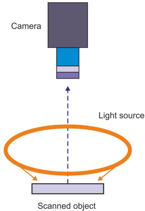
*Fig. 6.7 Dark-field ring lighting – low angle lighting*
