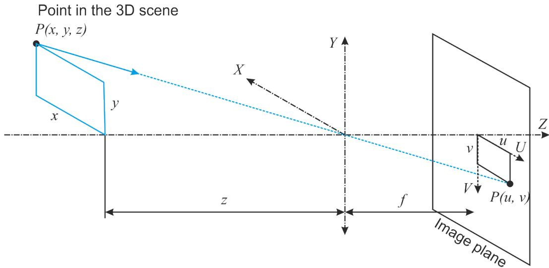
Fig. 1.5 Geometry of perspective projection, so called pinhole camera model
