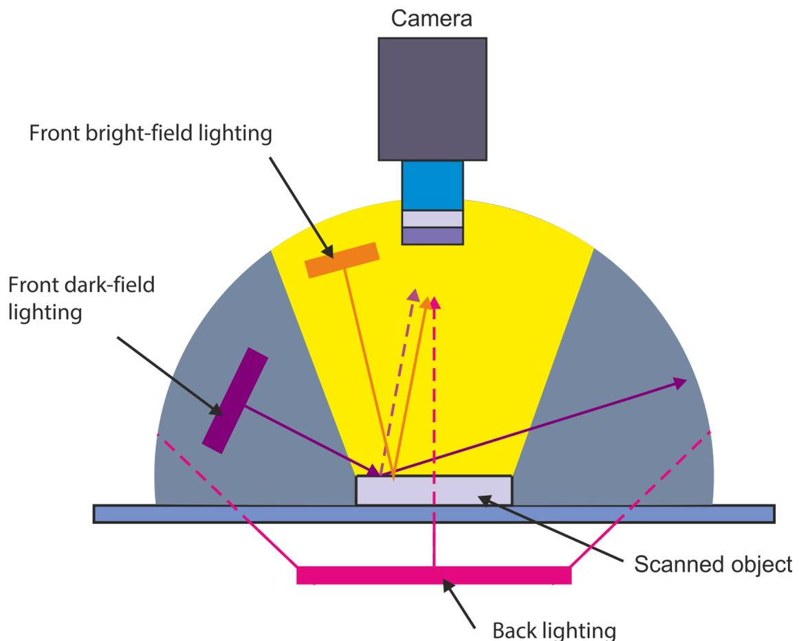
*Fig. 6.1 Basic geometry of light used when designing machine vision solution*
