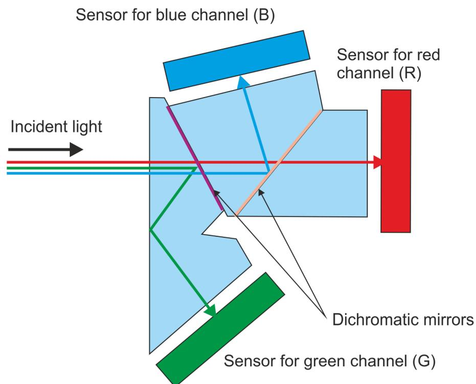
*Fig. 2.5 Principle of three-chip configuration for image capturing in colour using area sensor*
