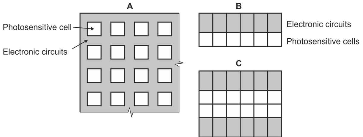
*Fig. 3.7 Configuration of area and line sensor, C – dual-line sensor*
