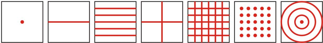
Fig. 6.11 Example of laser lighting types, from the left: point, line, 5 lines, cross, grid, matrix of point, set of circles
