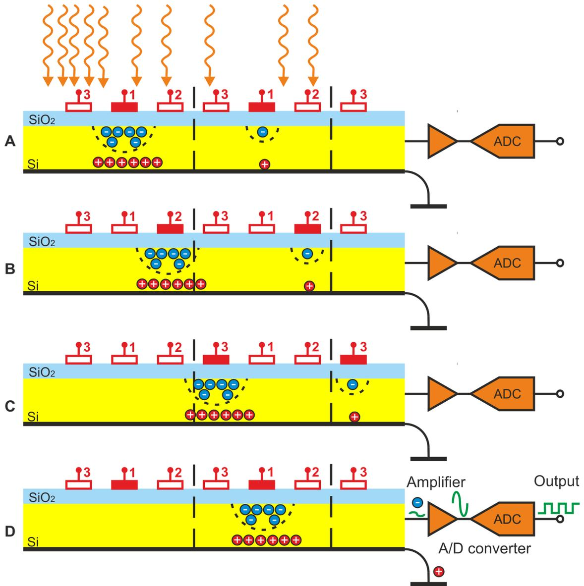
Fig. 2.1 The principle of CCD sensor operation
