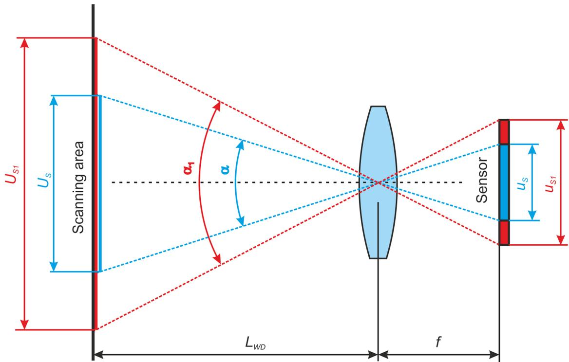
Fig. 4.3 Relation between angular field of view, focal length and sensor size
