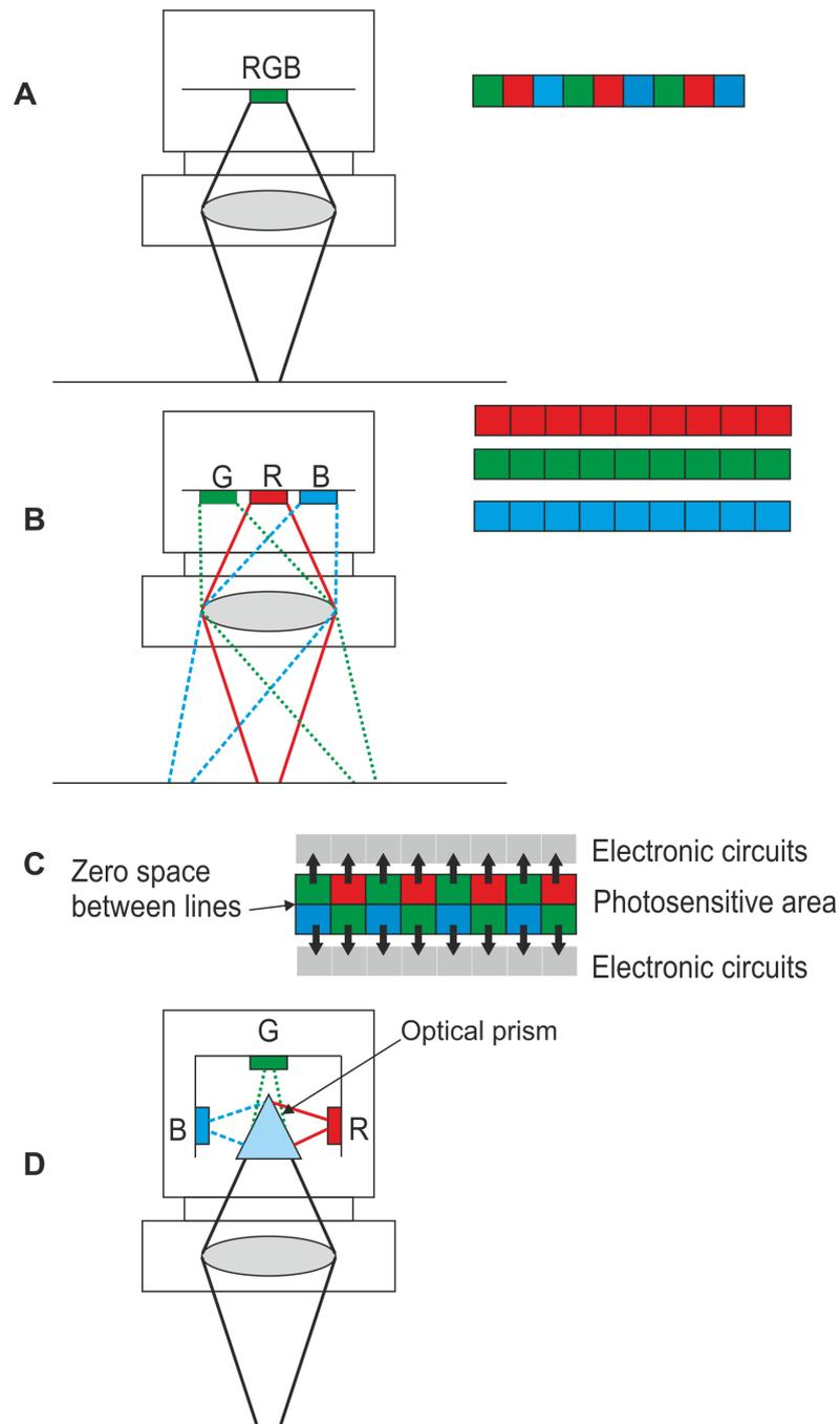
*Fig. 2.8 Variants of line cameras fitted with filters for colour image capture*
