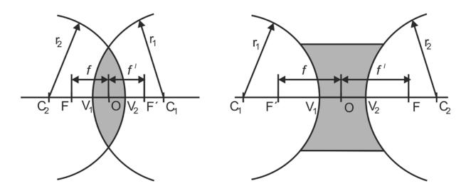
Fig. 4.2 Parameters of negative lens and positive lens
