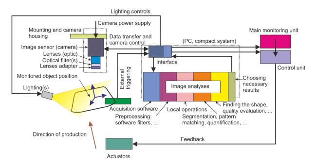
Fig. 1.11 Diagram of the vision system
