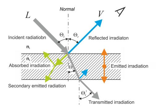
Fig. 1.3 Interaction of radiation and observed object
