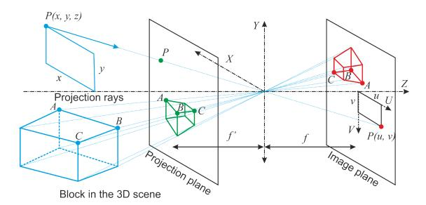
Fig. 1.6 Geometry of perspective projection of a point and a block, display of a plane of projection, so called pinhole camera model
