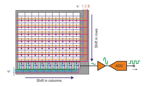
Fig. 2.2 Principle of operation of area (matrix) CCD sensor, FF reading for mechanical shutter
