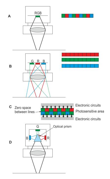
Fig. 2.8 Variants of line cameras fitted with filters for colour image capture
