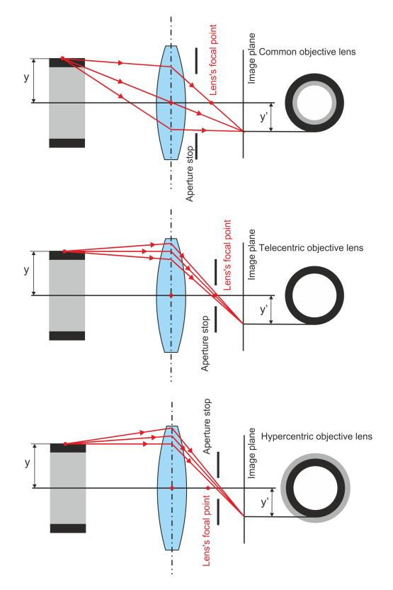
Fig. 4.6 Difference in scanning by means of normal, telecentric and hypercentric objective lens
