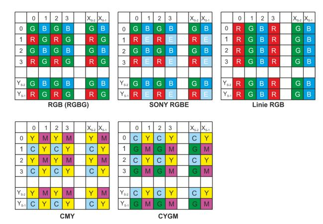
Fig. 2.6 Bayer RGB filter, Sony RGBE, CMY a C-Y-G-M filter for area sensor cameras
