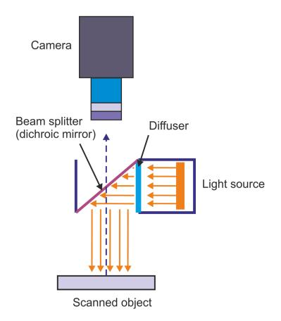
Fig. 6.6 Diffused on axis lighting
