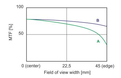
Fig. 4.5 The MTF (modular transfer function) characteristics, A – common objective lenses, B – example of special high quality objective lenses; accurate MTF curve also depends on working distance and aperture value; the parameters are distinguished separately for radial and tangential direction
