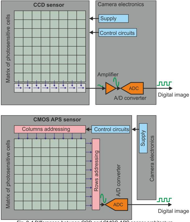
Fig. 2.4 Differences between CCD and CMOS APS sensor architecture
