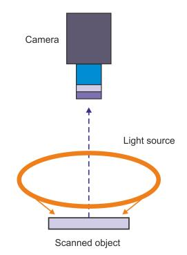
Fig. 6.7 Dark-field ring lighting – low angle lighting
