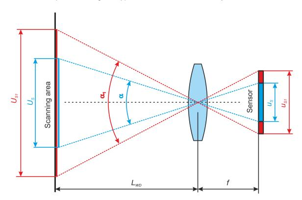
Fig. 4.3 Relation between angular field of view, focal length and sensor size
