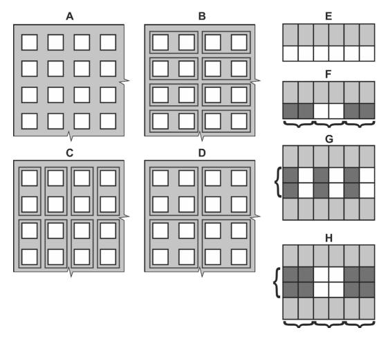
Fig. 2.9 Pixel binning – principle of merging neighbouring pixels: A - area sensor without merging neighbouring pixels, B – area sensor with horizontal merging, C – area sensor with vertical merging, D – area sensor with horizontal and vertical merging, E – line sensor without merging neighbouring pixels, F – line sensor with horizontal merging, G – dual-line sensor with vertical merging, H – vertical and horizontal pixel binning
