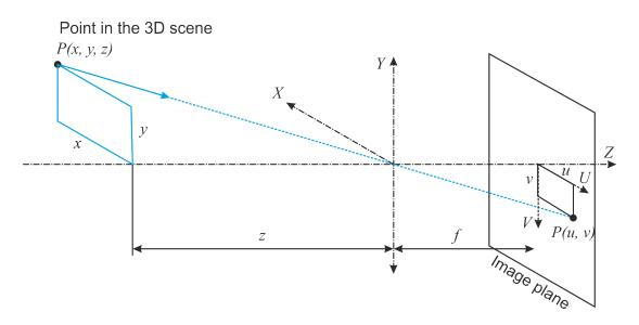
Fig. 1.5 Geometry of perspective projection, so called pinhole camera model
