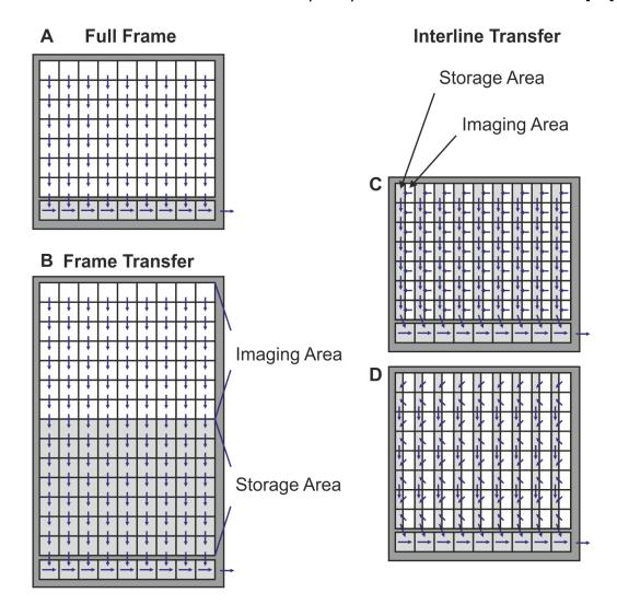
Fig. 2.3 Sensor diagram according to their reading method A - FF, B - FTR, C - ITR progressive reading, D - ITR interlaced reading (reading even images)
