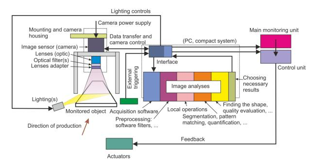
Fig. 3.6 Diagram of a system with line scan camera
