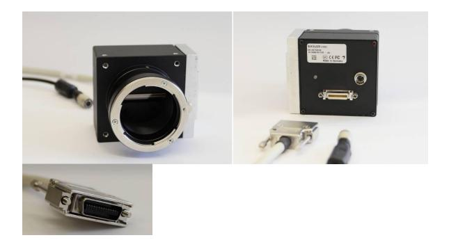
Fig. 3.4 Line scan camera and Camera Link connector
