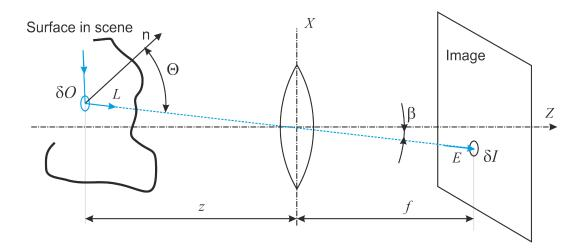
Fig. 1.7 Relation between radiation intensity E and lighting L
