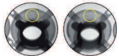
Comparison of X-ray images of castings using standard technology and the new technology
