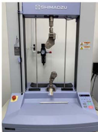
Figure 4. (Left) Merino wool yarn loaded in capstan grips on the Shimadzu load frame. (Right) Force vs. strain data for 10 samples of Merino wool yarn.
