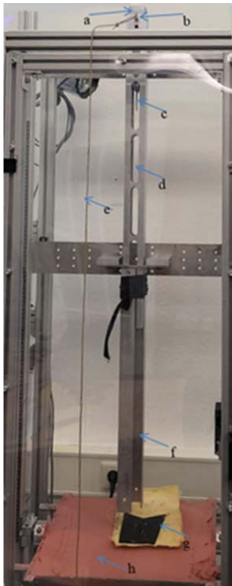
Figure 4: Drop test stand with: a) Dropping weight b) Dropping weight fixing hook c) Knife d) Safety path e) Hook pulling rope f) Safety bar g) Specimen of plastiline h) Plastiline
