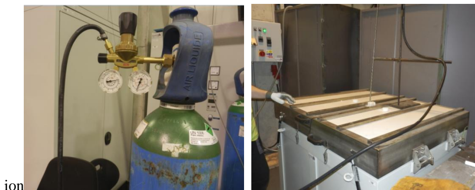
Fig. 7.54 Argon used for direct foaming of the aluminium alloy melt in the furnace
