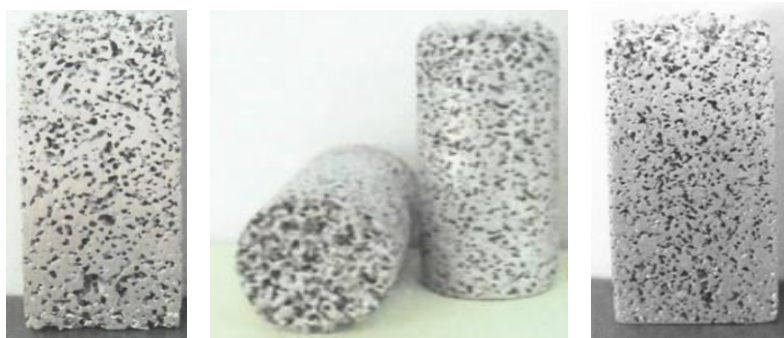
sample produced using 0.6 mm NaCl particles (left) sample produced using NaCl particles with a particle size of 0.3 mm (right)
