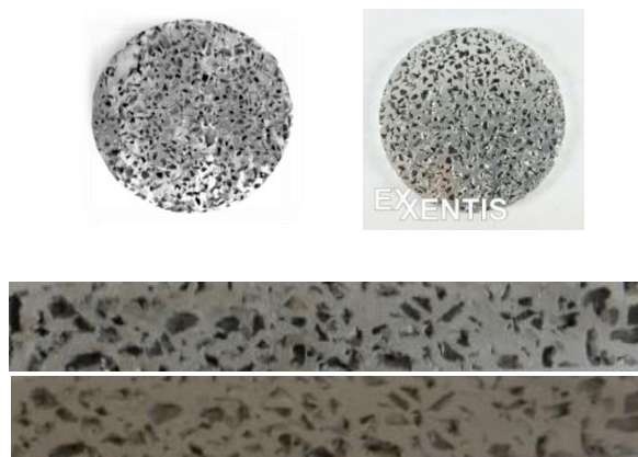
Fig. 7.12 Macrostructure of a porous sample of aluminium alloy AlSi 12, \varnothing 60 x 10 mm, left; aluminium alloy cut by EXXENTIS, right; cross-section through the manufactured sample, bottom
