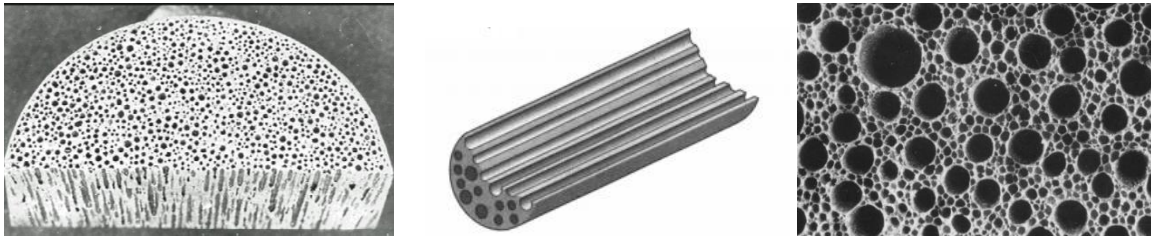
Fig. 1.17 Cellular metal system produced by the Gasar method, contains mostly elongated pores (cells), according to V. Shapovalov, as shown in [1]
