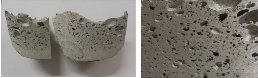
Fig. 7.60 View of a section through AISi7Mg0 alloy specimen 2, left and its foamed part (foamed specimen \varnothing 118 mm; maximum height 80 mm), right, specimen 2
