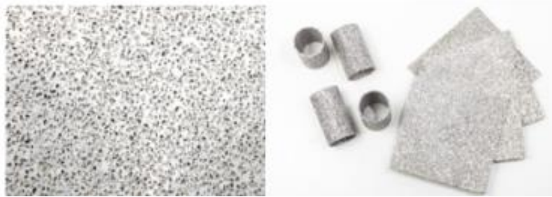
Fig. 2.21 Products made of porous aluminium material with salt particles promoted by Material District, Narden [19]
