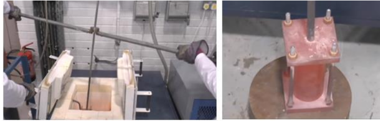
Fig. 2.17 View of the open furnace, when removing the mould with special preparation (left), removed mould (right), [15]
