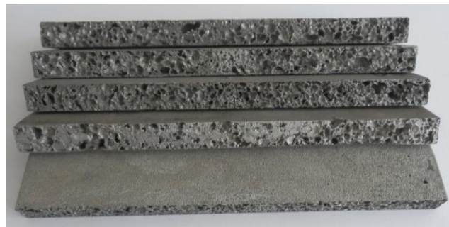
Fig. 1.25e) Aluminium foams with surface crusting, based on powder technology (AlSi12 and \text{TiH}_2 powder), size 150 x 50 x 10 mm, [55]
