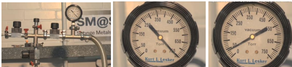
Fig. 2.16 T distribution system, flowing into the mould; switching on the vacuum pump and creating a vacuum until the gauge needle reaches "0", [15]
