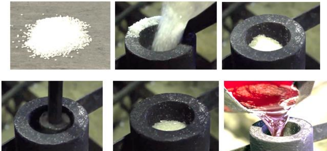
Fig. 2.4a) Production of porous aluminium, at the time of pouring the salt into the mould and subsequent impregnation of the salt with the aluminium melt to form the Al-NaCl composite system, ALUPOR
