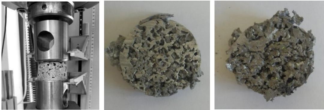
Fig. 7.38 Strength measurements on the TIRA Test machine and samples after the compressive test
