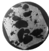
Fig. 7.61 View of the sample for metallographic observation of the distribution of Al_2O_3 particles
