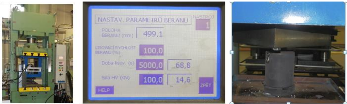
Fig. 7.20 View of the hydraulic press and its monitor with the setting of the necessary values of the pressing parameters
