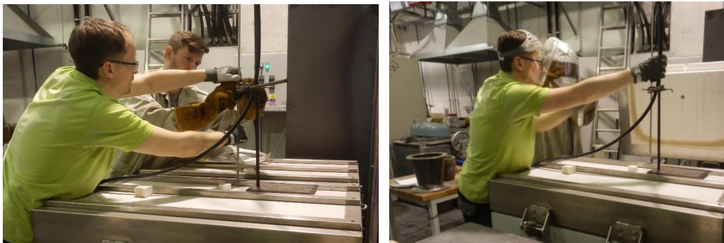
Fig. 7.52 Preparation of the foaming process and view of the introduction of the foaming sensor into the aluminium melt, Dr. Sobotka and Dr. Korecek
