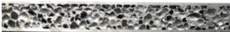
Fig. 1.28b Structure of an AFS sandwich panel, thickness approx. 10 mm, with all parameters maintained in the correct manufacturing process [54]
