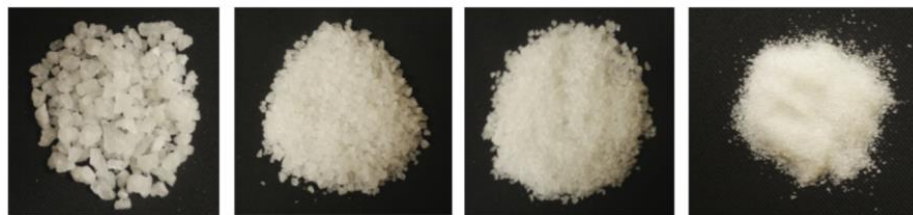
A B C D (A: 8 to 10 mm; B: 5 to 7 mm; C: 3 to 5 mm; D: 1 to 3 mm)
