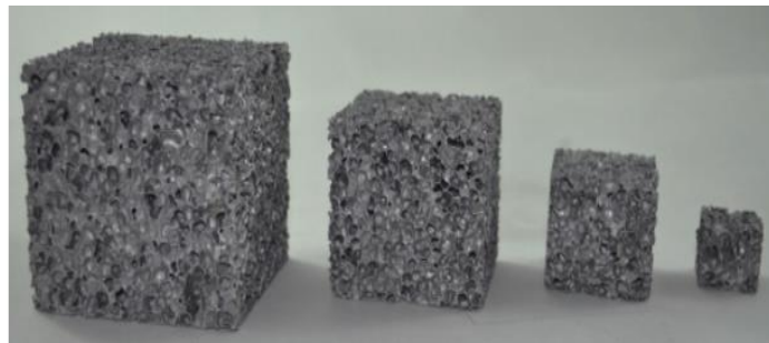
Fig. 1.10c) Cutting of aluminium foam produced by the ALPORAS method (1.5 % wt. Ca; 1.6 % wt. TiH_2 foaming agent) [18]
