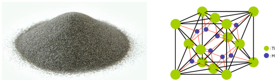
Fig. 4.3 Titanium hydride, a very reactive chemical compound (melting point 450 °C, density = 3760 kg·m -3 , molar mass 49.91 g·mol -1 ), cubic crystal lattice FCC TiH 2 with the tetrahedral arrangement of hydrogen atoms [20]
