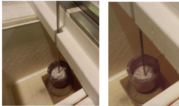
Fig. 7.53 View of the foamed melt in the ceramic crucible
