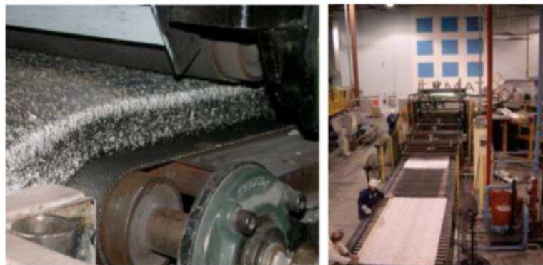
Fig. 1.5b) Conveyor belt of the continuous aluminium foam production line by CYMAT [1]
