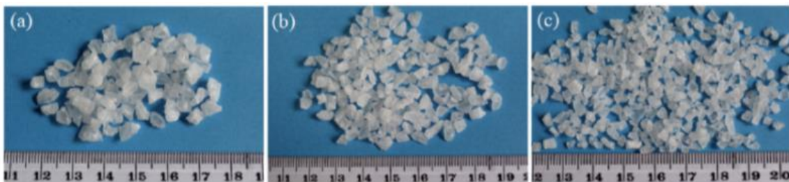
Fig. 2.38 View of NaCl particle sizes used for the production of porous aluminium systems (aluminium "foams"): (a) NaCl particle size from 4.7 to 4.0 mm; (b) NaCl particle size from 4.0 to 3.3 mm; and (c) NaCl particle size from 3.3 to 2.0 mm [27].
