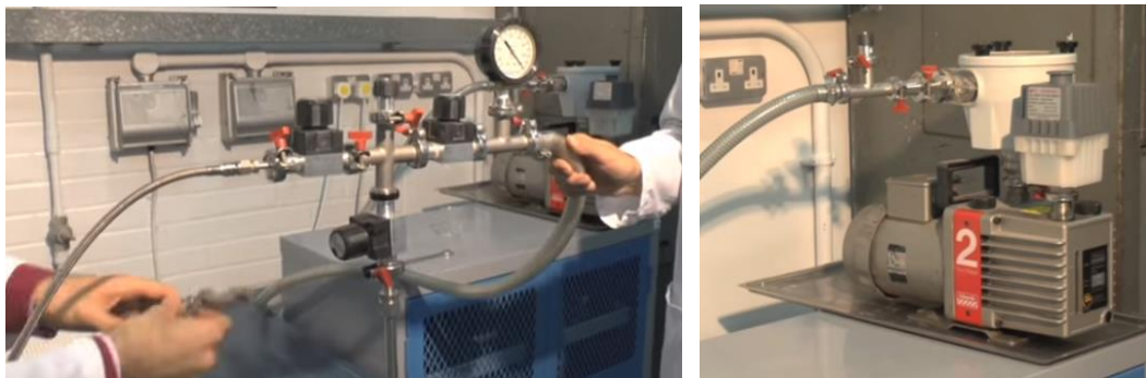
Fig. 2.15 View of the vacuum system for extracting air from the assembled mould, [15]
