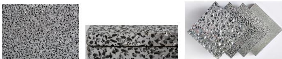
Fig. 2.20c) Structure of porous aluminium materials based on Al-NaCl, (produced by Alumeco Group and Exxcentis) [17]
