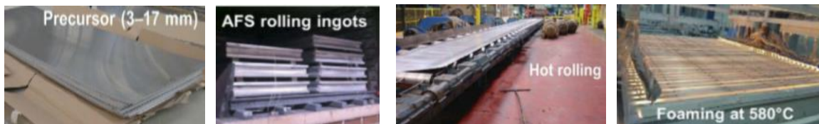
AFS rolling ingots, Hot rolling, Precursor (3-17 mm), Foaming at 580 °C
