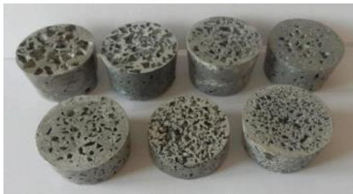
Fig. 7.21 View of fabricated samples of aluminium porous material, AISi12 alloy, perspective view (samples 1,2,3,4,5,6, and 7)
