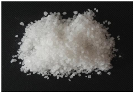
Fig. 7.8 Sodium chloride used for the production of porous aluminium
