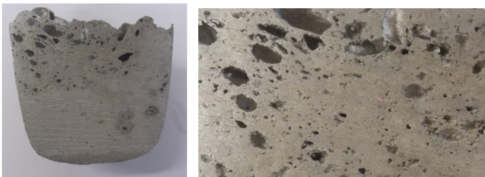
Fig. 7.66 Section through a fabricated foamed specimen ( \varnothing 125 mm; \varnothing 85 mm; maximum height 105 mm), left and plan view of the foamed part of the AlSi5Mg specimen (50 x 75 mm section), right
