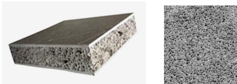
Fig. 4.11 Metal foam (metal cellular system) fabricated using \text{ZrH}_2 foaming agent (left); porous aluminium foam structure fabricated using \text{TiH}_2 , the area shown is 80 x 80 mm (right), Nanjing University, Southeast China
