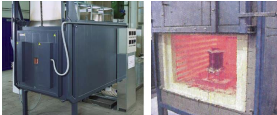
Fig. 1.25c) Resistance electric furnace for realization of the foaming process of aluminium semi-finished products produced by powder metallurgy (LKR company), [55]
