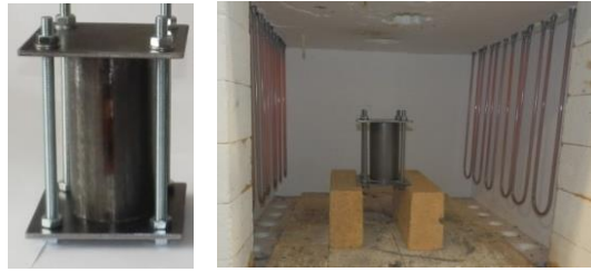
Fig. 7.9 Preparation and furnace for the production of porous aluminium systems
