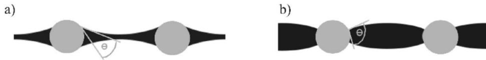
Fig. 3.14 Schematic of the effect of contact angle on effective particle bridging, a) the stability condition is 90^\circ for \theta \leq ; b) the instability condition is \theta > 90^\circ , according to IPA [33].
