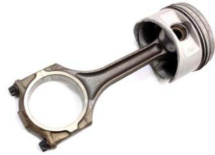
Fig. S48. Piston and connecting rod
