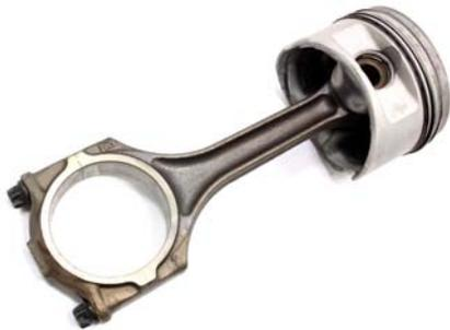
Fig. I08. Connecting rod and piston – actual machine parts
