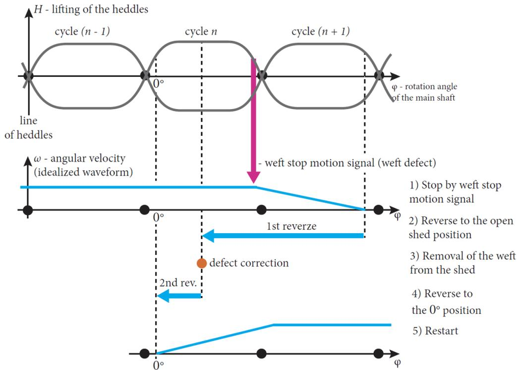
Figure 193: Positioning with weft thread defect
