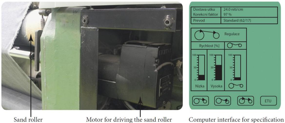
Figure 72: Photograph of the main parts of the fabric take-up system of the Picanol Gamma machine
