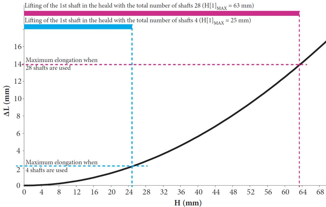
Figure 143: Maximum elongation for the heald with 4 and 28 shafts
