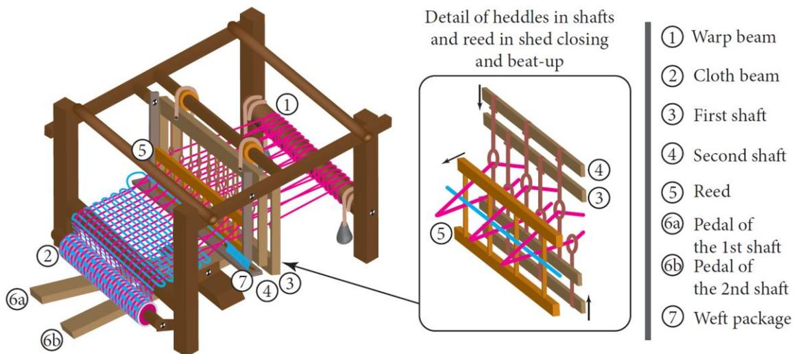
Figure 10: Scheme of hand loom from the Middle Ages
