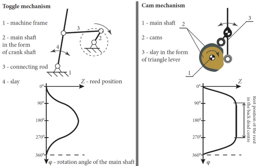
Figure 178: Kinematic diagram of the fourbar and cam beat-up mechanisms
