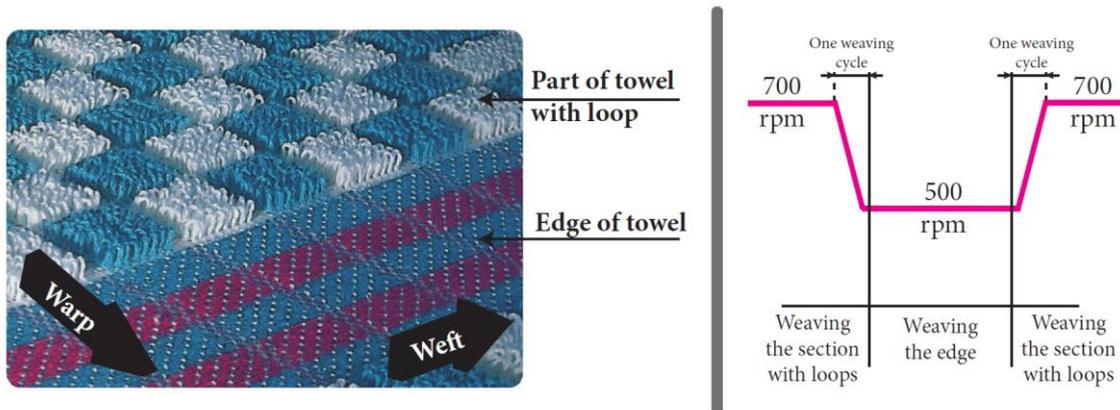
Figure 65: Example of automatic speed change in the production of terry cloth (source [20])
