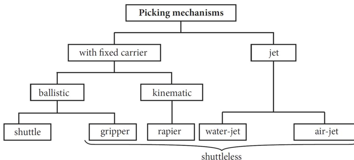
Figure 145: Division of picking mechanisms
