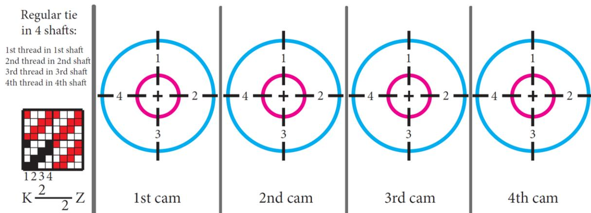
Figure 95: First step of the procedure for drawing the shapes of cams for stitched 4-harness twill
