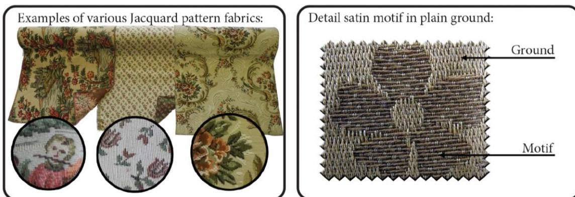
Figure 35: Examples of various Jacquard pattern fabrics and detail of fabric with a satin pattern and a plain ground
