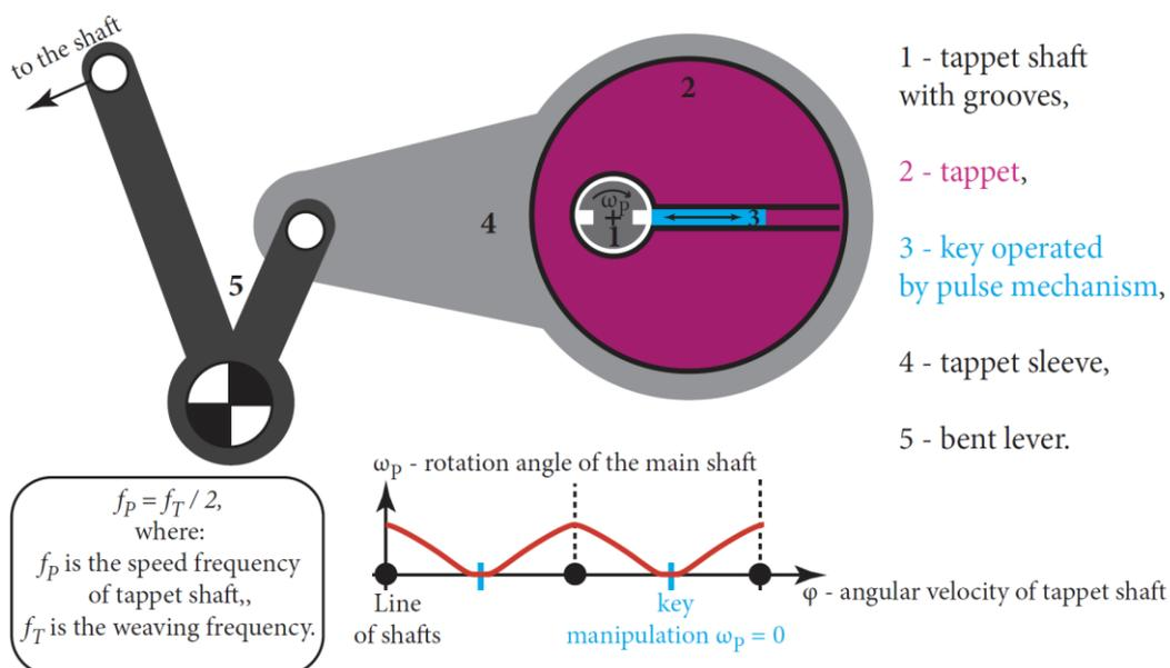
Figure 106: Diagram of the rotary dobby mechanism
