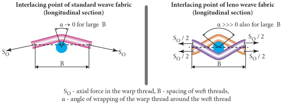
Figure 198: Interlacing point of standard and leno weave fabric at low number of weft threads per unit length (in longitudinal section)
