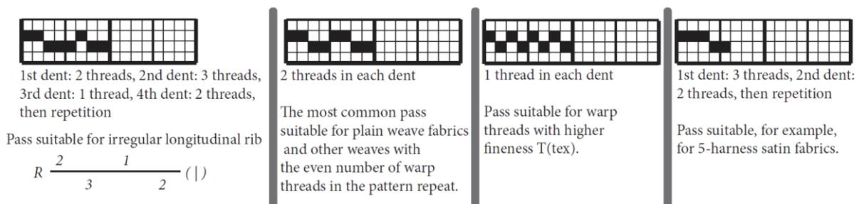
Figure 115: Examples of different ways of passing the warp threads through the dents of the reed
