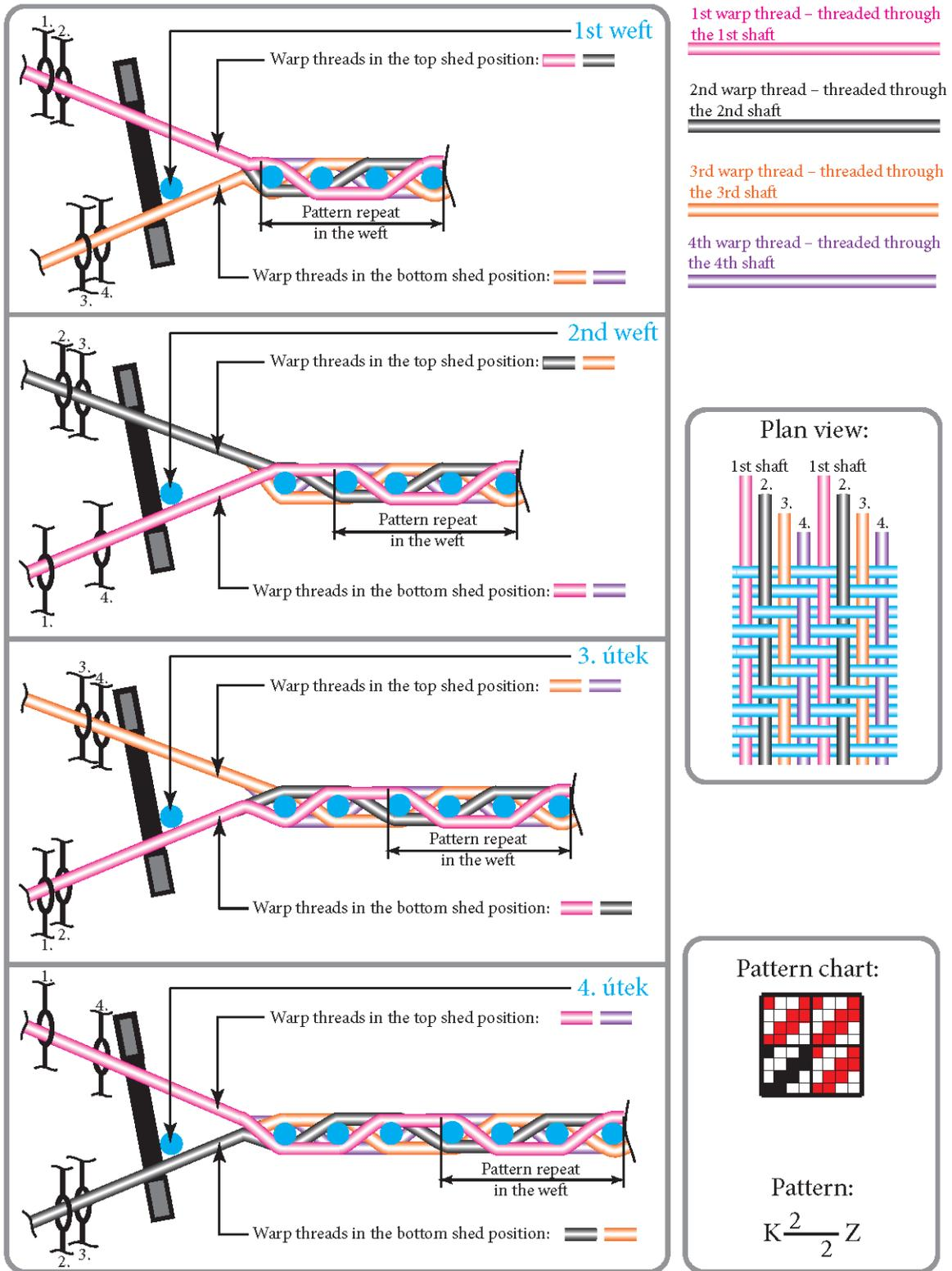
Figure 80: Diagram of the position of shafts in making a stitched 4-harness twill using four shafts with plain draft
