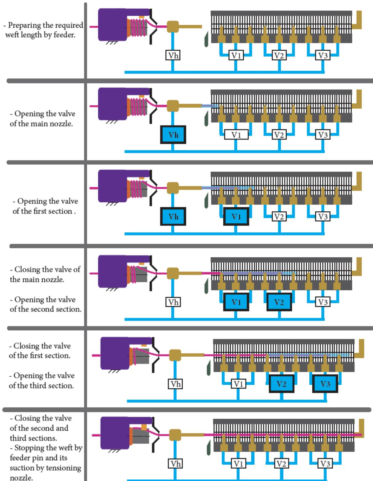
Figure 171: Diagram of weft insertion on the air-jet weaving machine
