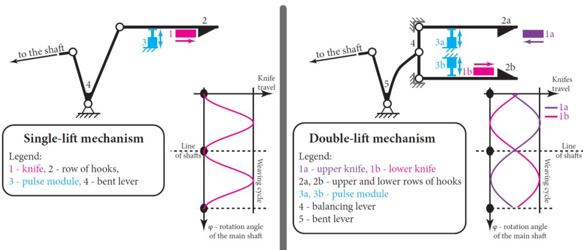
Figure 102: Hattersley single-lift and double-lift dobby mechanism
