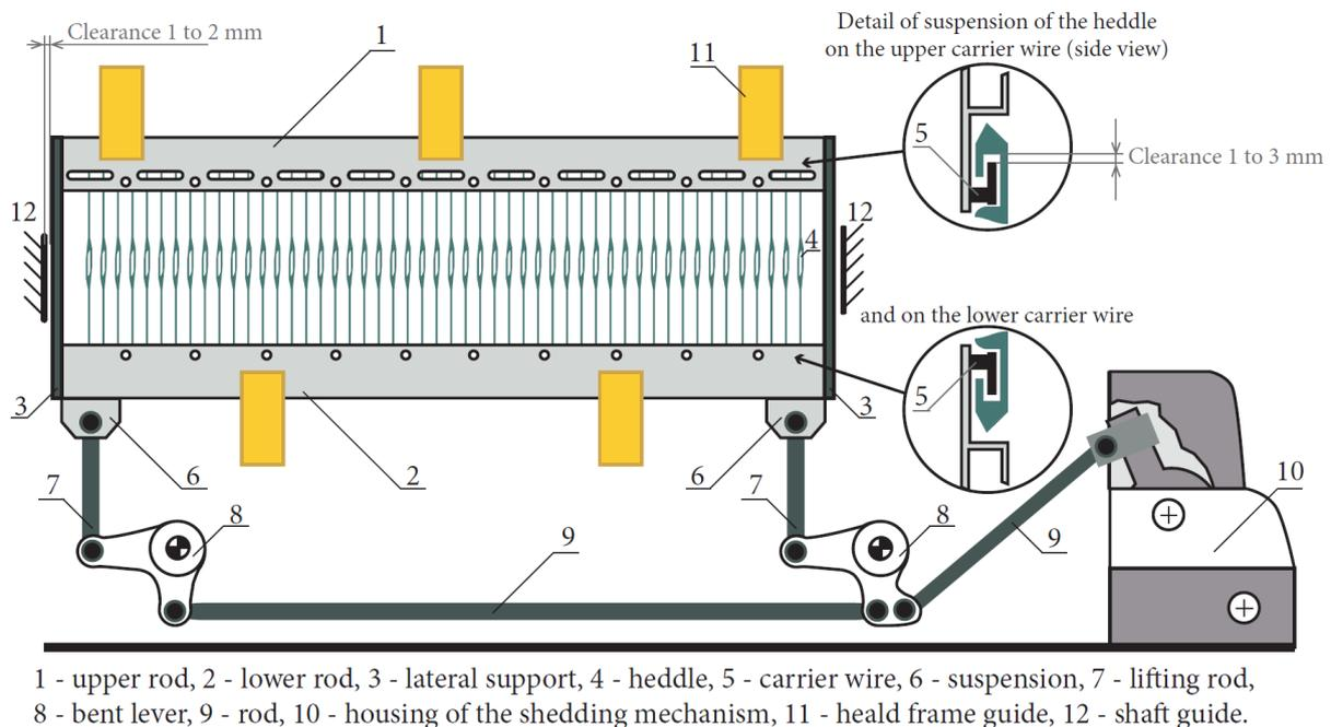
Figure 81: Main parts of the heald shaft and its configuration
