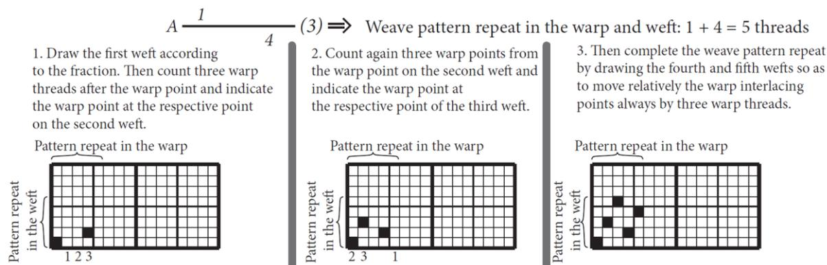
Figure 31: Drawing procedure for 5-harness satin weave with move numbers 3
