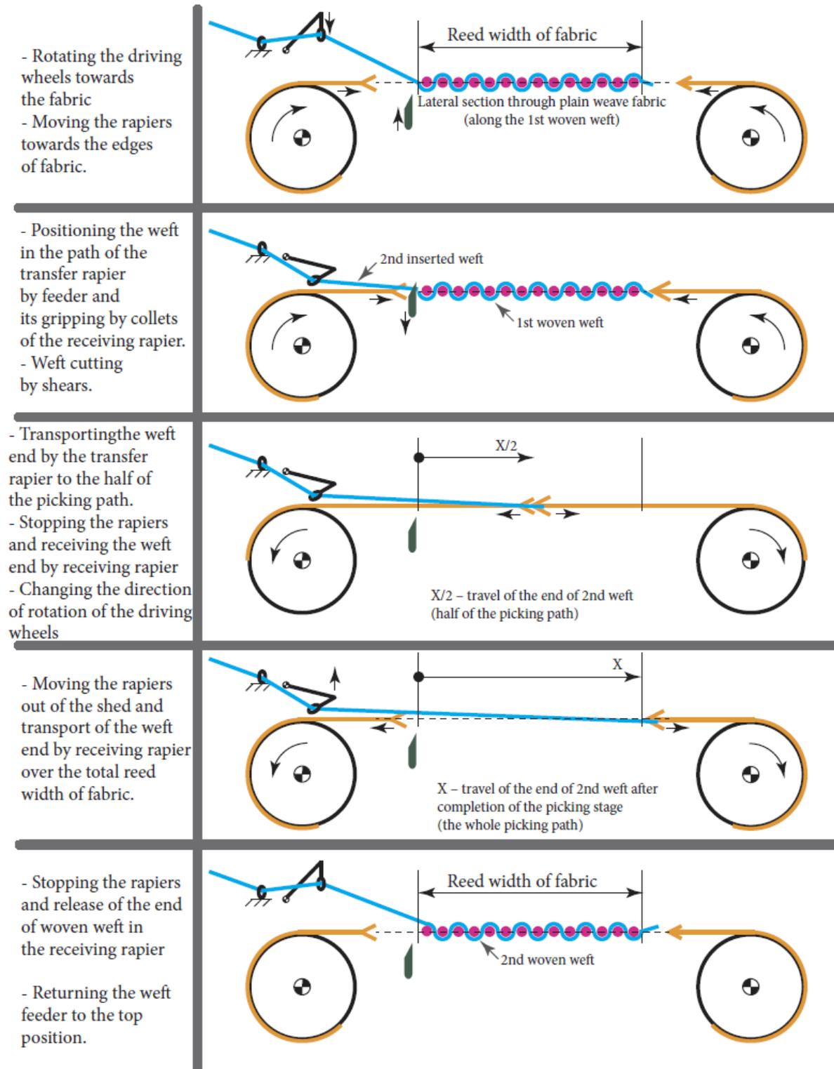
Figure 154: Simplified diagram of the weft insertion by means of two flexible rapiers
