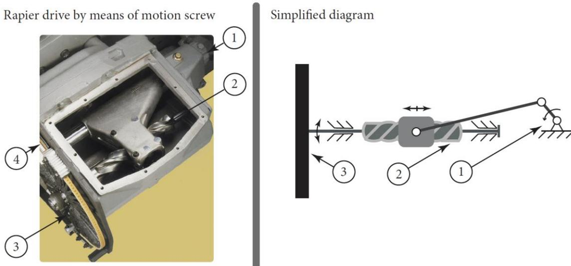
1 - main shaft drive, 2 - motion screw, 3 - driving wheel of the rapier, 4 - rapier
