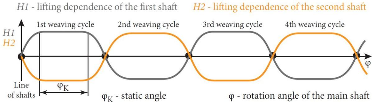
Figure 94: Lifting dependence of shafts during four weaving cycles for plain weave
