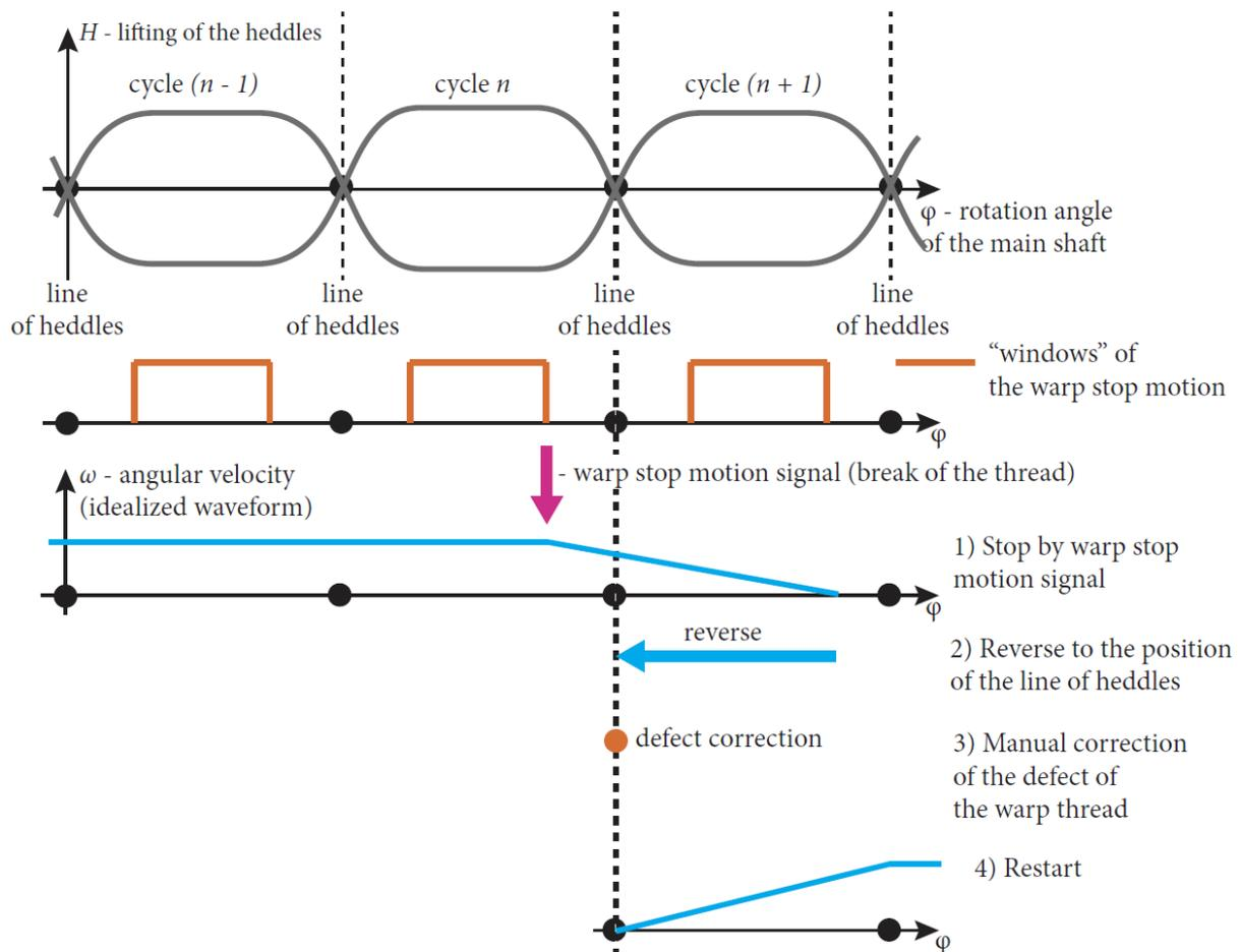
Figure 192: Positioning with warp thread defect
