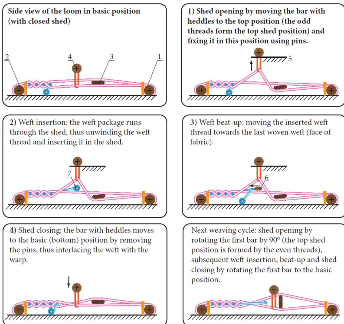
Figure 9: Phase of fabric production on the ancient Egyptian loom
