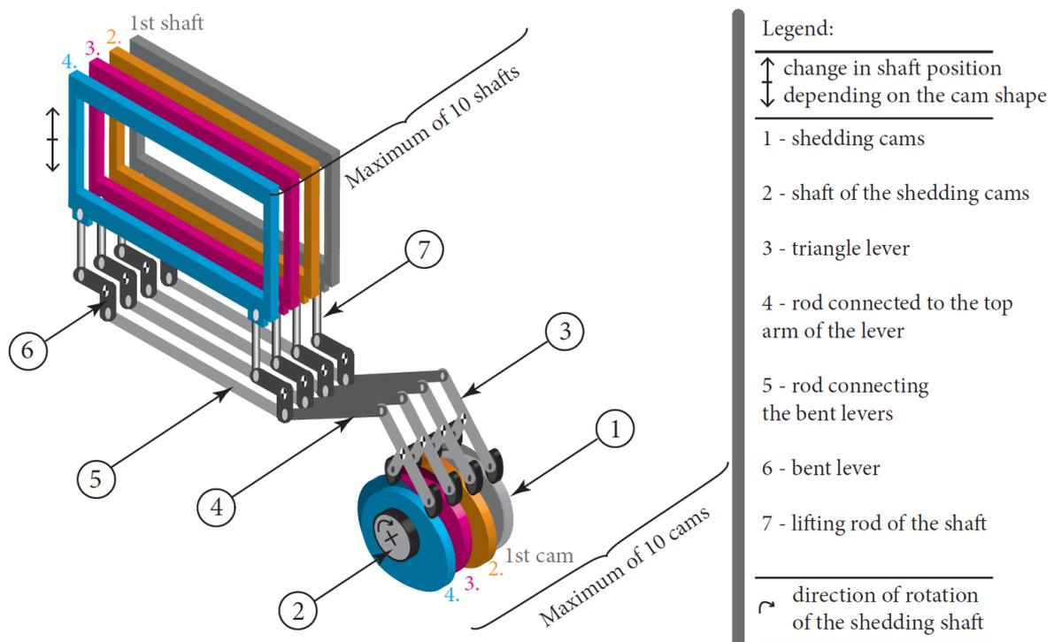
Figure 89: 3D diagram of the cam shedding mechanism with four shafts
