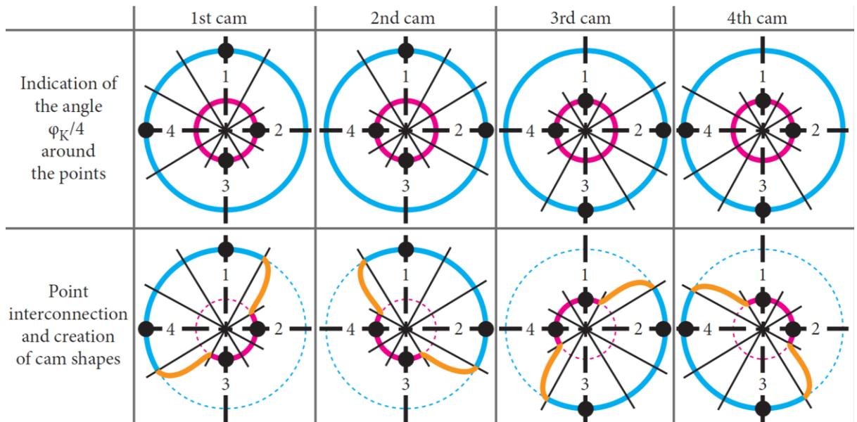
Figure 97: Last step of the procedure for drawing the shapes of cams for stitched 4-harness twill
