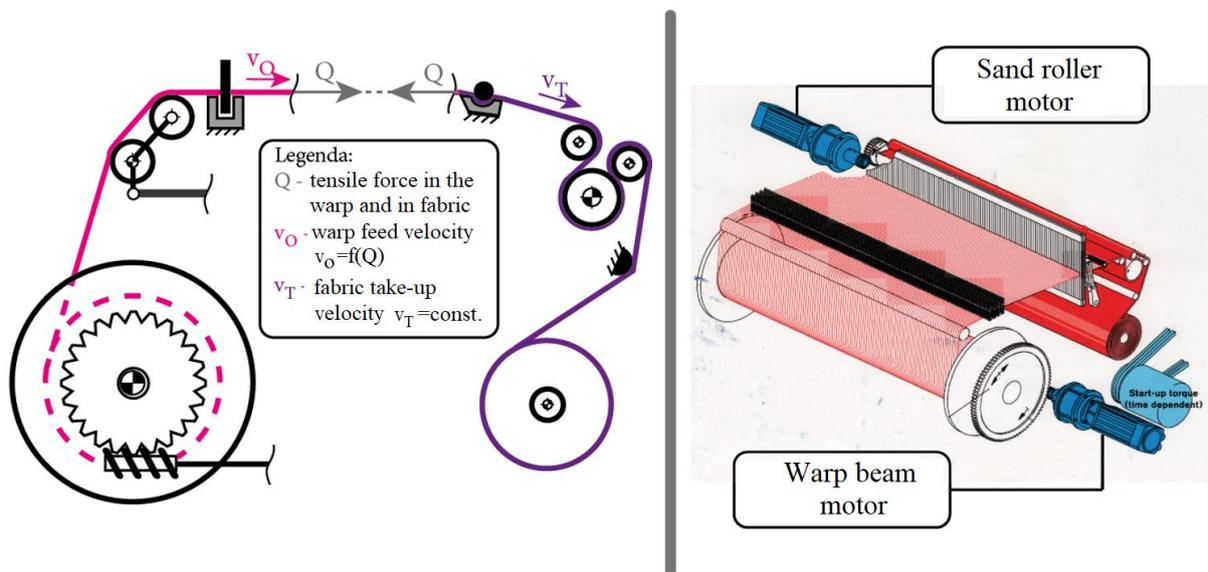
Figure 66: Warp unwinding and fabric take-up
