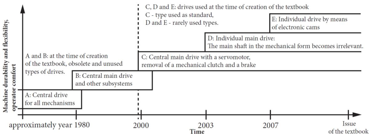
Figure 59: Development stages of drives at the turn of the Millennium
