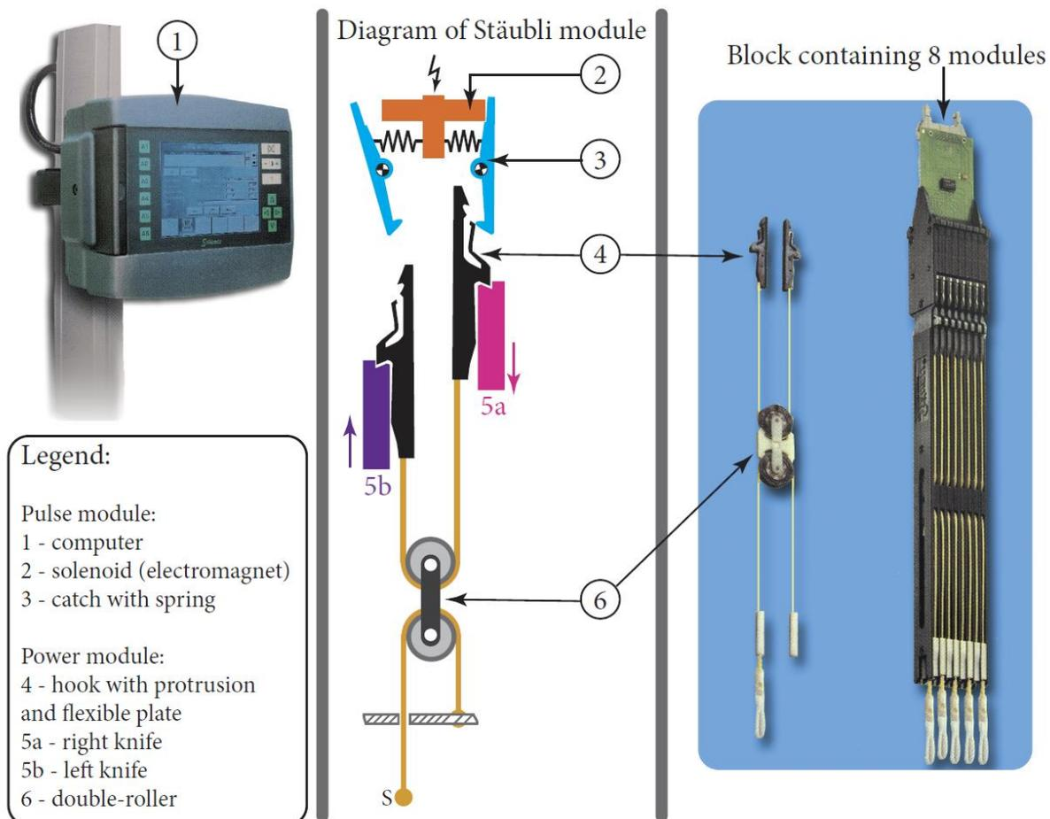
Figure 131: Main parts of the Stäubli Jacquard mechanism (source [27])
