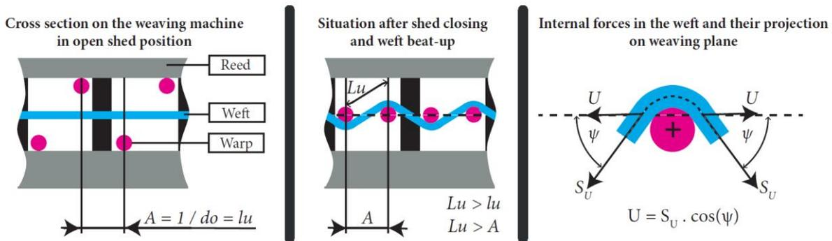
Figure 42: Situation after inserting weft in the shed and after interlacing it
