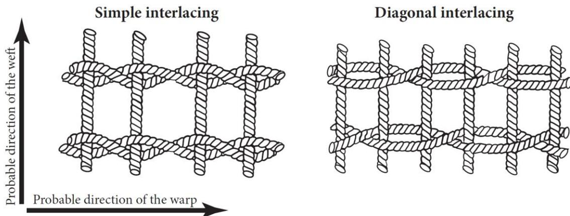
Figure 6: Scheme the oldest fabrics with the so-called “simple and diagonal interlacing”
