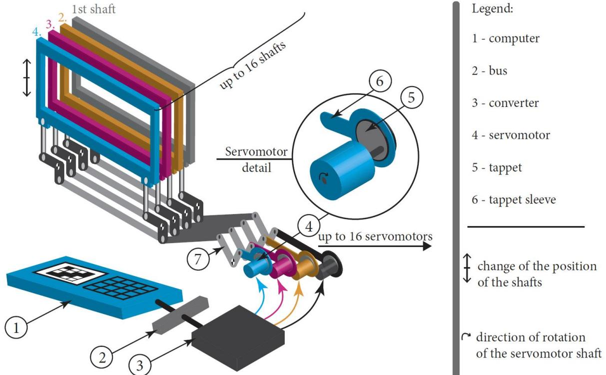
Figure 138: Main parts of the shedding mechanism with electronic cams
