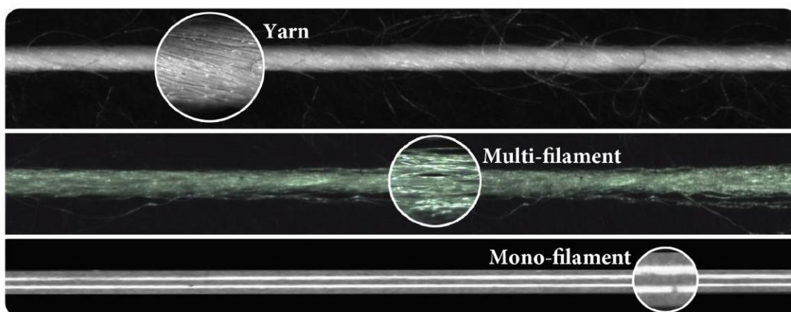
Figure 12: Examples of threads: yarn, multi-filament and mono-filament
