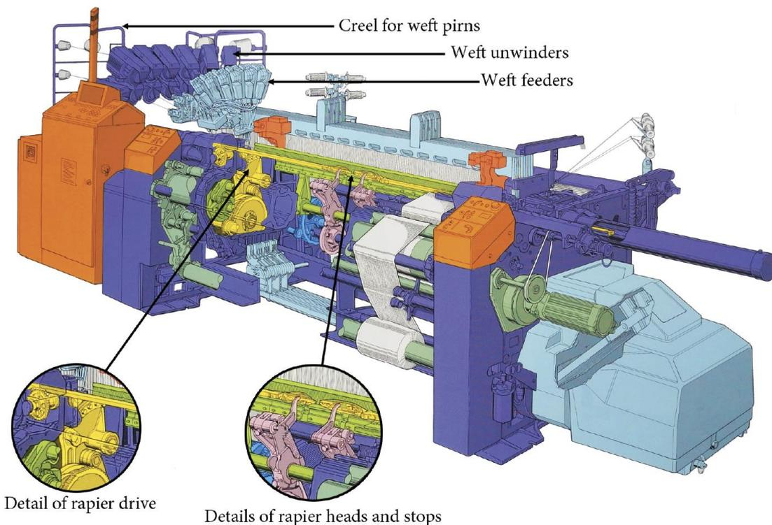
Figure 156: Dornier rapier weaving machine with rigid rapiers (source [30])
