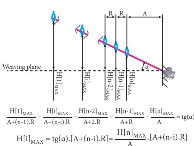
Maximum lifting of the individual shafts in the heald for: - total number of shafts  $n = 28$ ,
