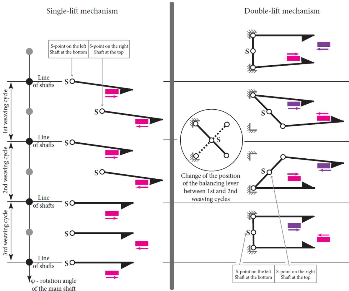
Figure 103: Schematic representation of the extreme positions of the hooks and knives during three weaving cycles
