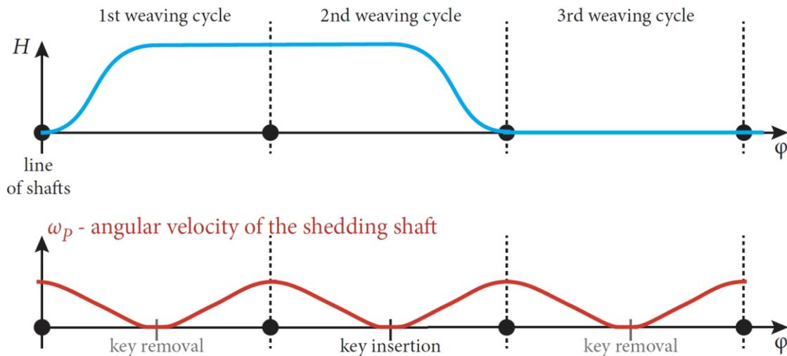
Figure 109: Course of shaft lifting during three weaving cycles for the above described model situation
