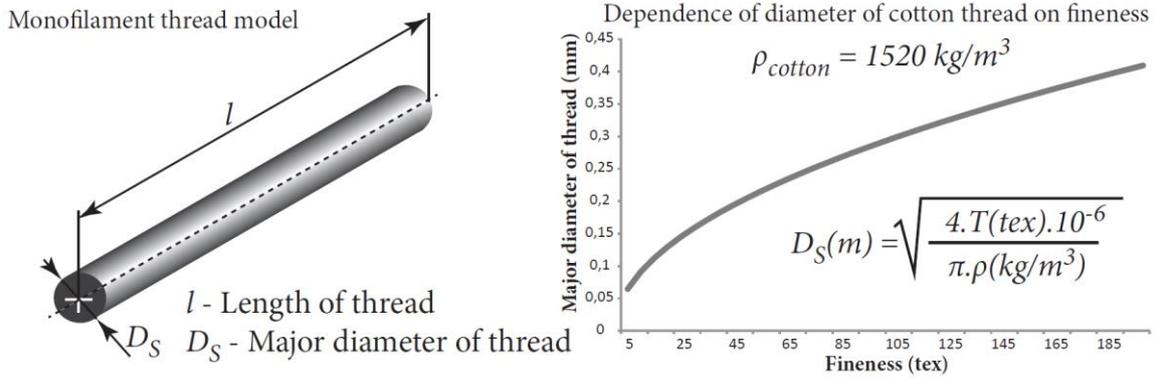
Figure 13: Model of thread (mono-filament), its major diameter and its fineness dependence
