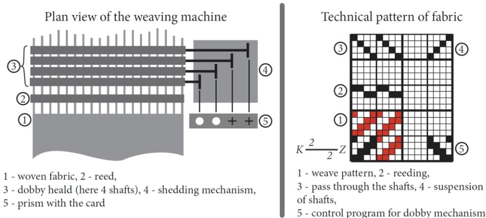
Figure 113: Plan view of the weaving machine and example of the technical pattern of fabric
