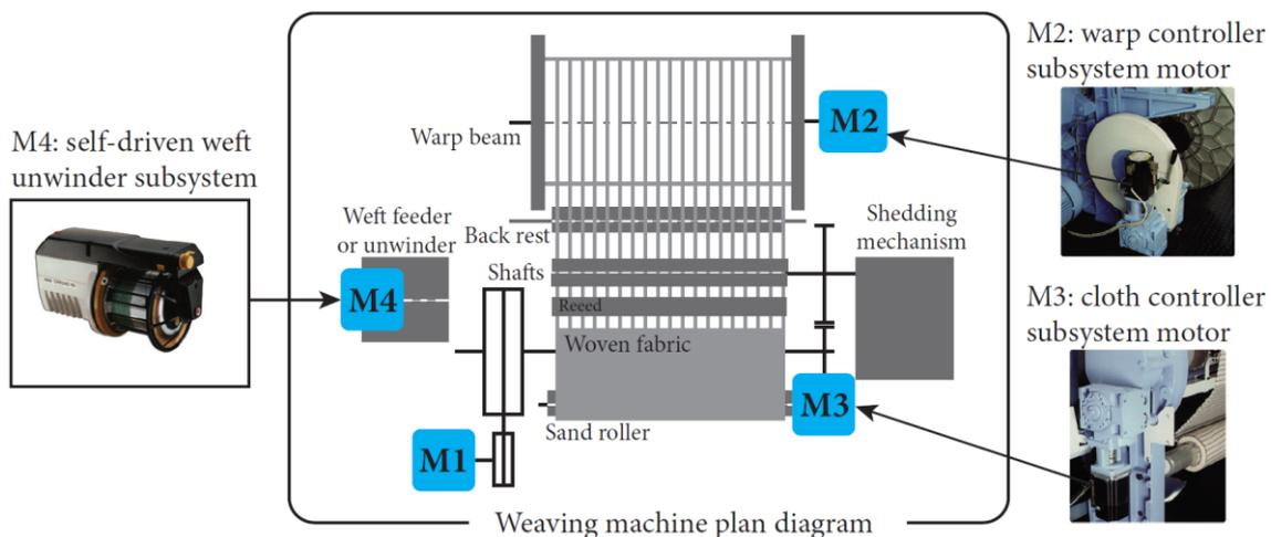
Figure 61: Structure of drive type B, subsystem photographs (source [18], [33])
