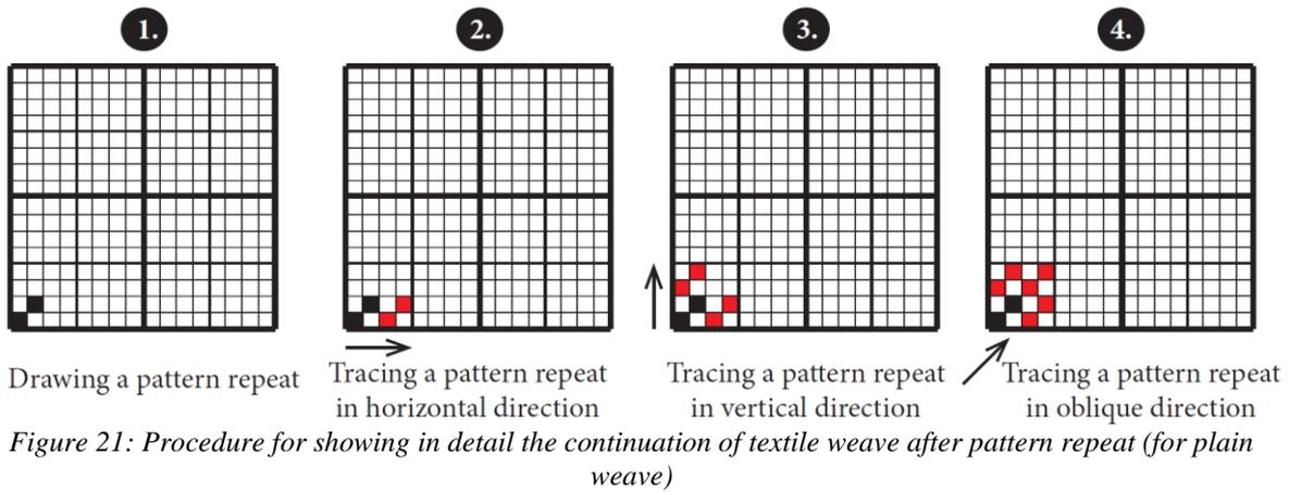
This makes it possible to relatively easily graphically represent any form of interlacing the warp and weft threads (see example of the so-called “5-harness twill weave” shown in Figure 22).
