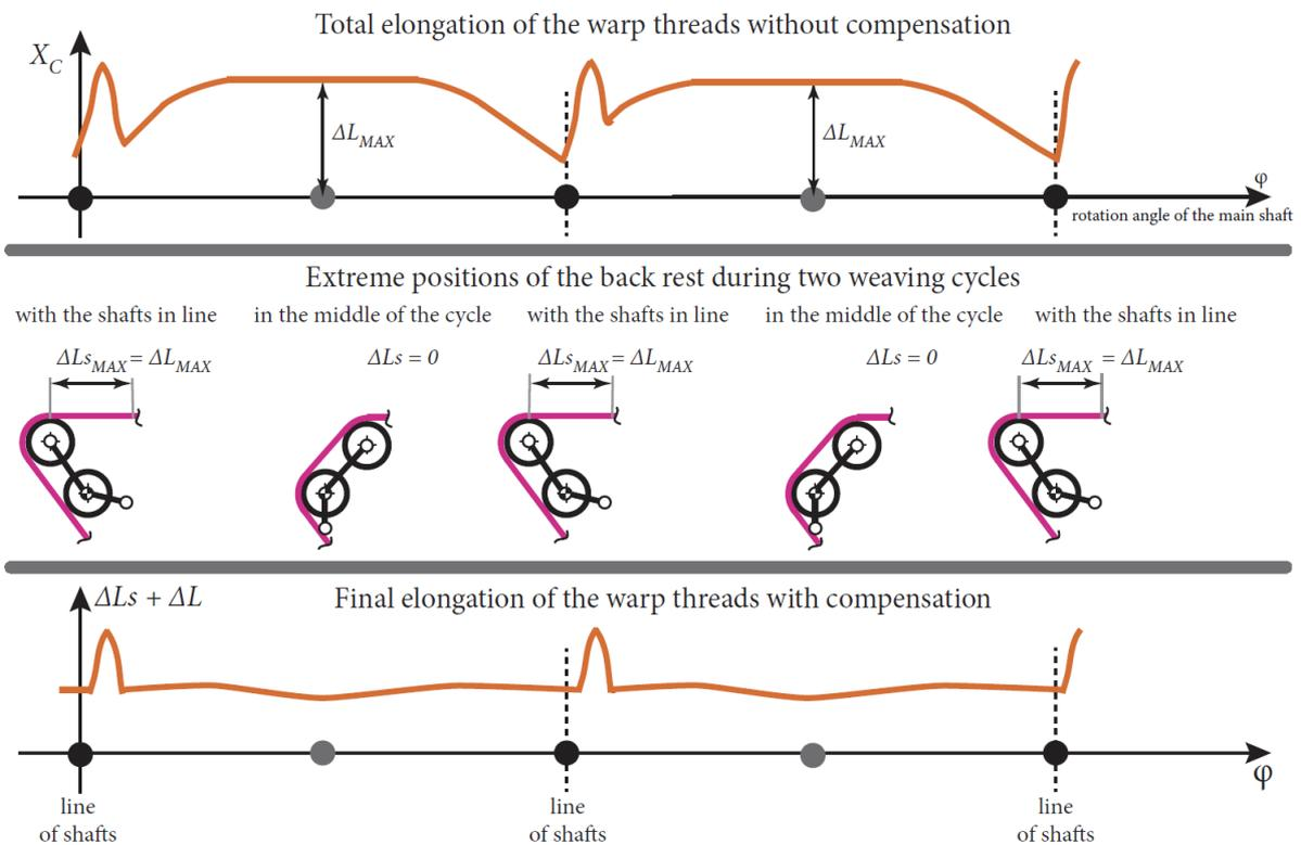
Figure 187: Operation of the back rest with forced drive in compensation for elongation of the warp threads
