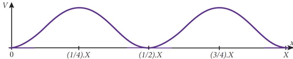
$V$  - weft velocity,  $x$  - picking path,  $X$  - reed width of fabric
