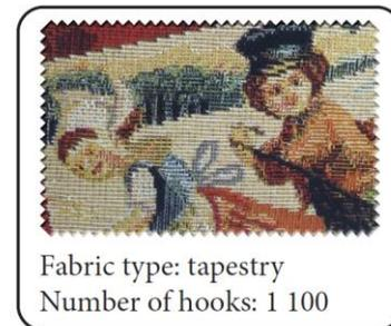
Figure 126: Examples of the fabrics produced with a certain number of hooks (source [26])
