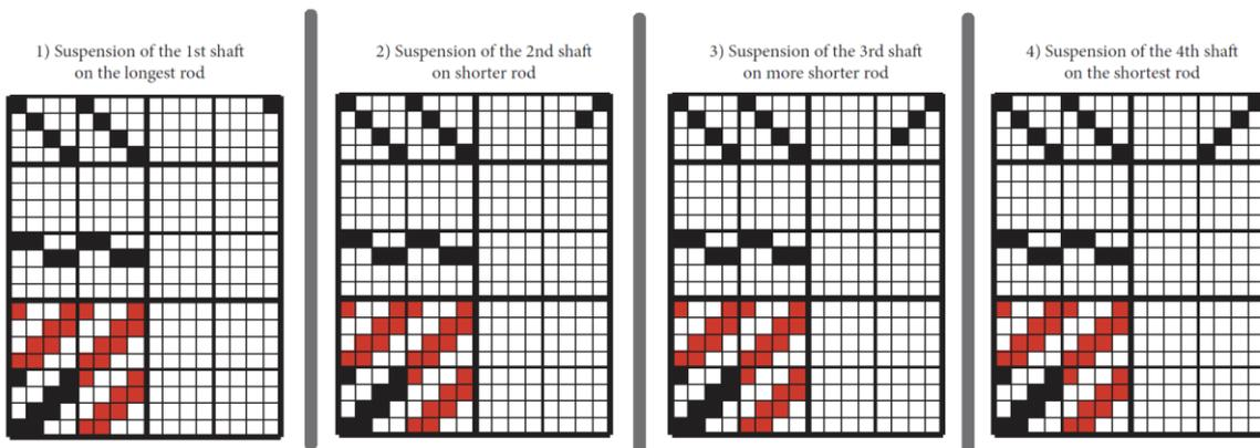
Figure 118: Procedure for drawing the suspension of shafts for the above technical pattern
