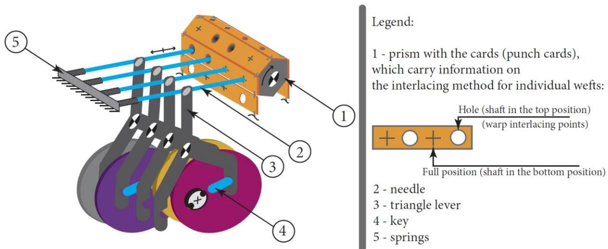
Figure 110: Main components of the pulse module of the mechanically controlled dobby mechanism
