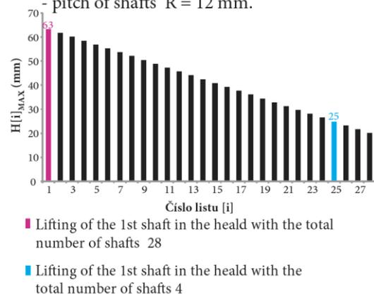
Figure 142: Maximum lifting of the individual shafts in the heald
