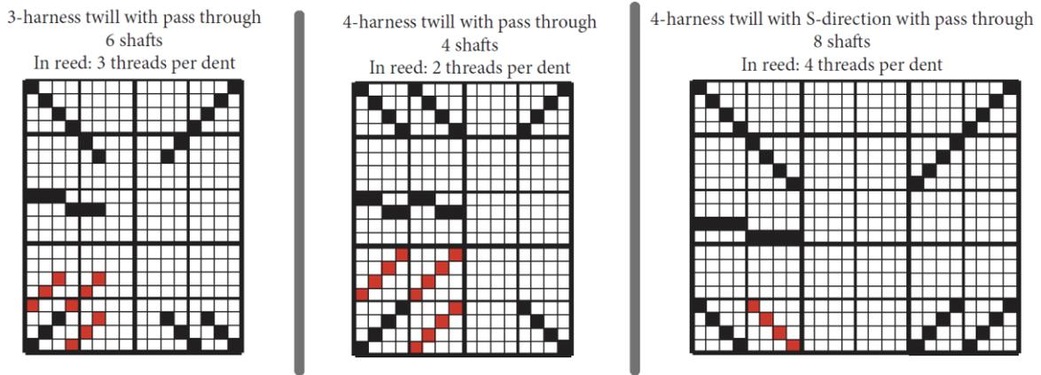
Figure 122: Technical patterns for different ground twills
