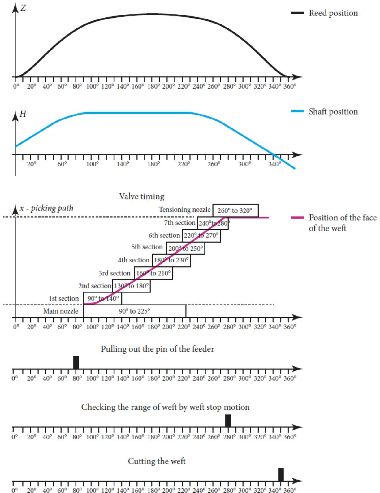
Figure 191: Operation of the mechanisms of the air-jet weaving machine depending on the rotation angle of the main shaft
