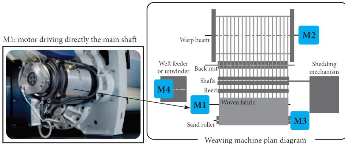
Figure 62: Structure of the drive type C, photographs of the motor for direct drive of the main shaft (source [16])
