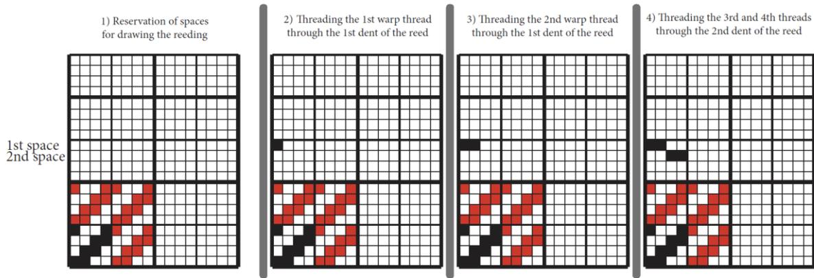
Figure 114: Procedure for drawing the reeding for the above technical pattern
