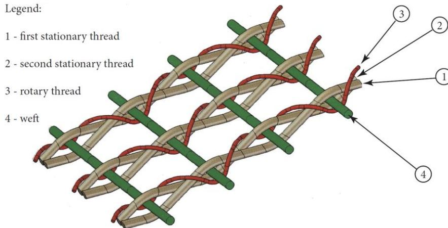
Figure 207: 3D diagram of the combined weave (source [19])
