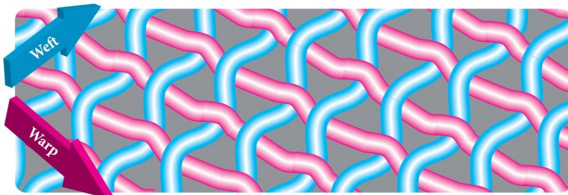
Figure 3: Scheme of standard plain weave fabric
