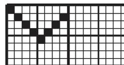
Figure 117: Example of the point tie in five shafts
