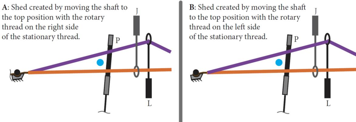
Figure 206: Rapier heald with the open shed and weft insertion
