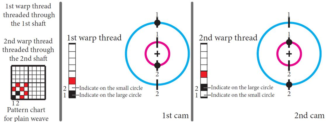
Figure 92: Second step of the procedure for drawing the shapes of cams for plain weave
