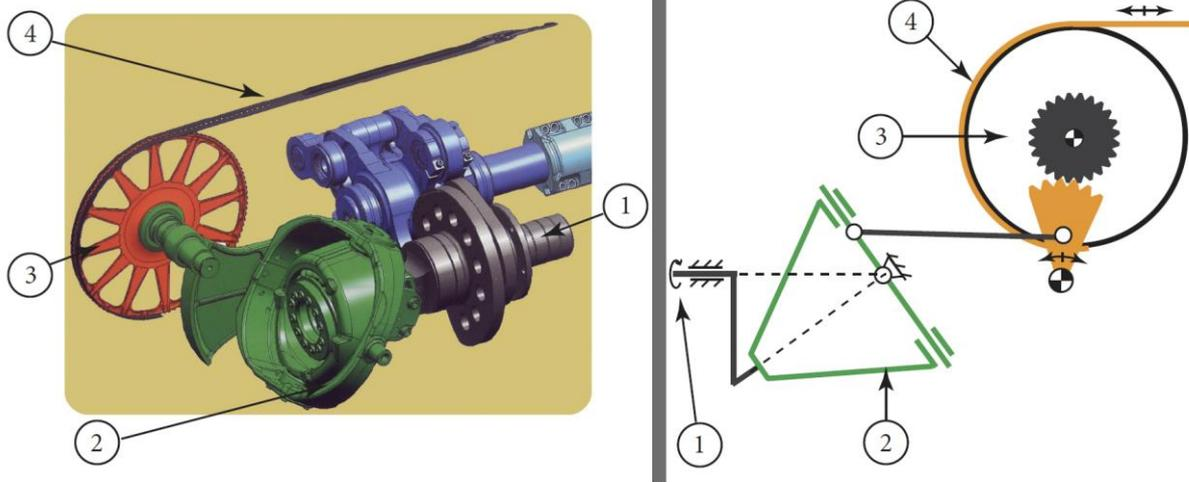
1 - main shaft drive, 2 - spatial toggle mechanism, 3 - driving wheel of the rapier, 4 - rapier
