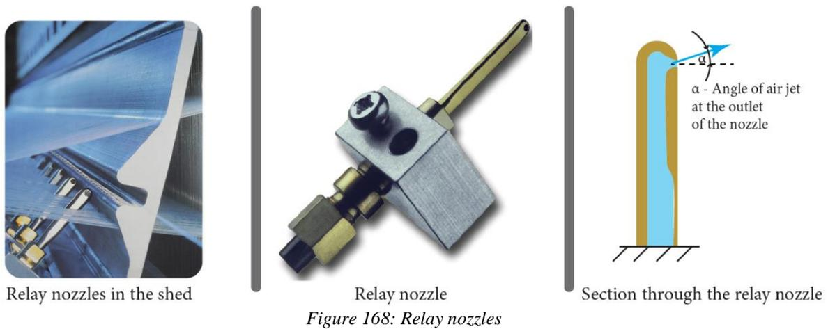
Figure 168: Relay nozzles
