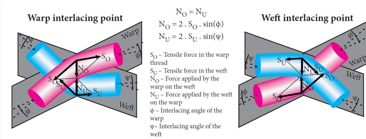
Figure 4: Warp and weft interlacing points, interaction of forces between the warp and the weft
