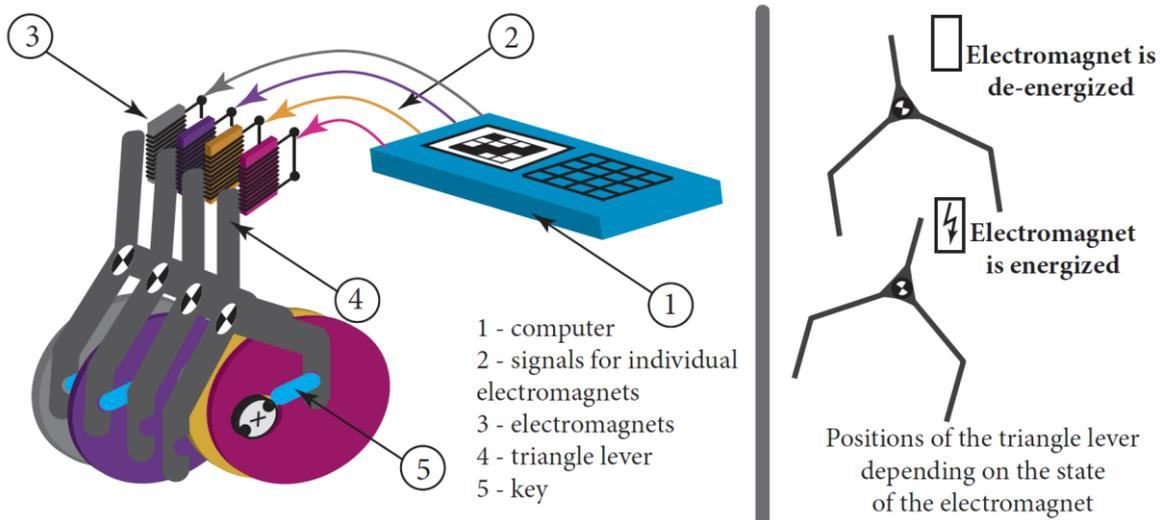
Figure 112: Main components of the pulse module of the electronically controlled dobby mechanism
