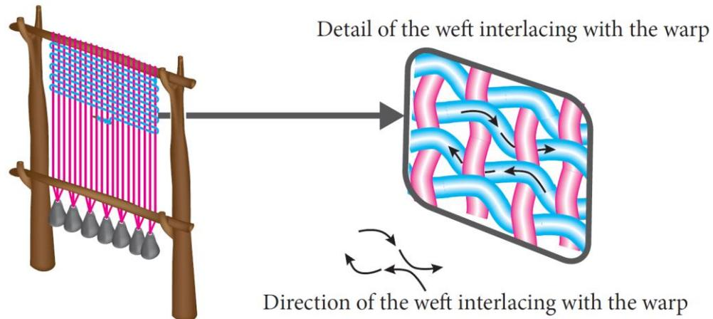
Figure 7: Probable method of fabric production in the Neolithic Age (vertical loom without a shedding device)
