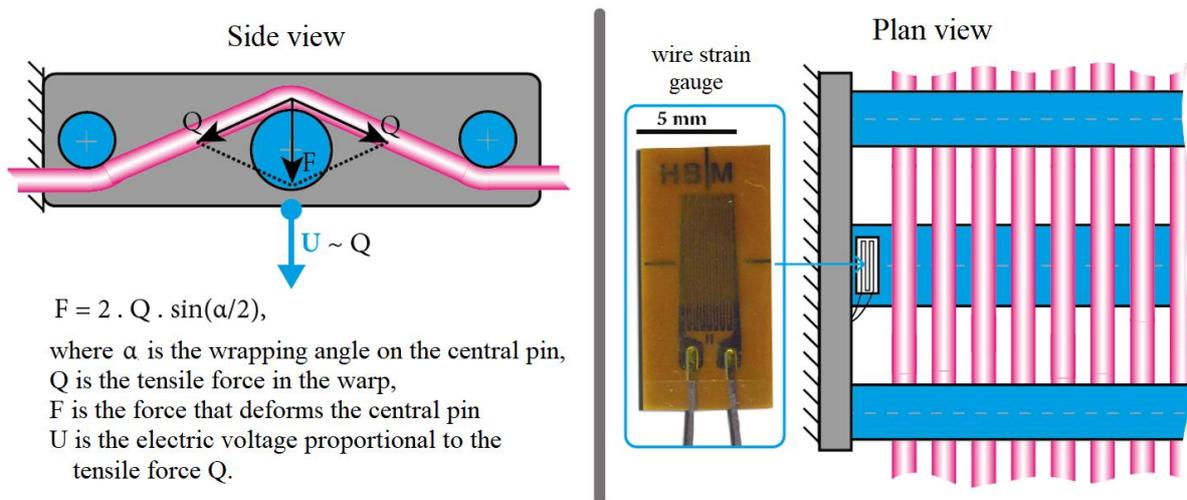
Figure 67: Strain gauge of the tensile force in the warp
