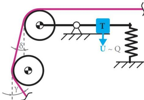
$\delta$  - The angle  $\delta$  on the second roller of the back rest is independent of the radius of package on the warp beam  $r_V$ .
