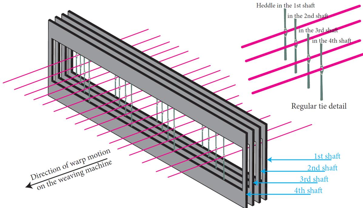
Figure 76: 3D diagram of the dobby heald with regular tie in four shafts
