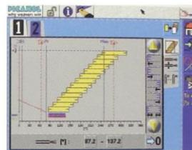
Interface for entering the values of the timing of nozzle valves in the setter mode.
