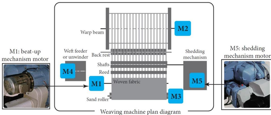
Figure 63: Structure of the drive D, photographs of motors for driving the beat-up and shedding mechanisms (source [18])
