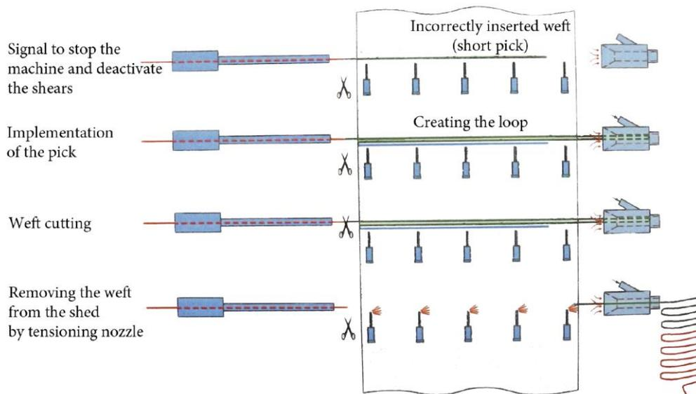
Figure 194: Diagram of the automatic unweaving on the Somet machine (source [15])
