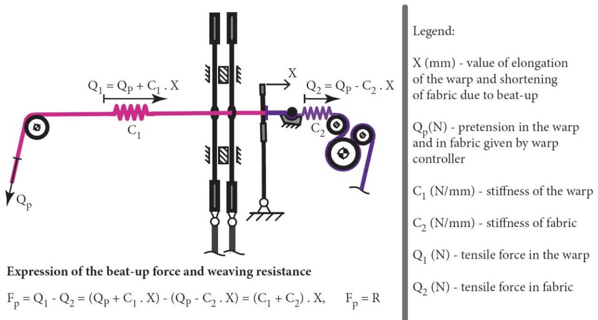
Figure 180: Diagram for expressing the beat-up force and the weaving resistance
