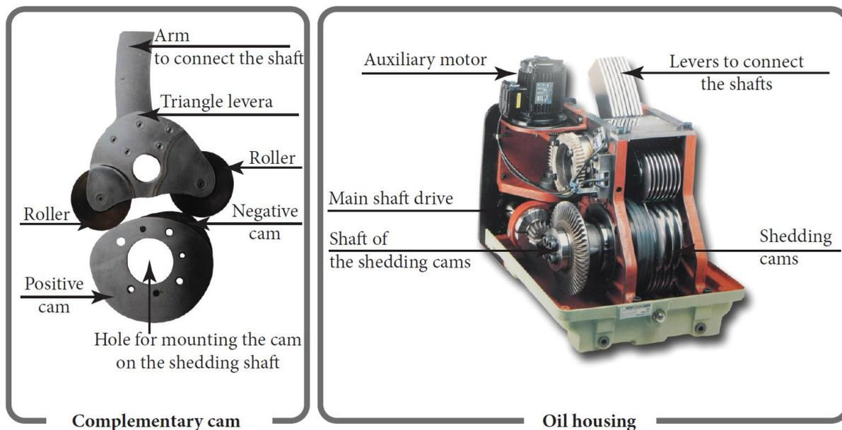
Figure 88: Main parts of the cam shedding mechanism (source [25])
