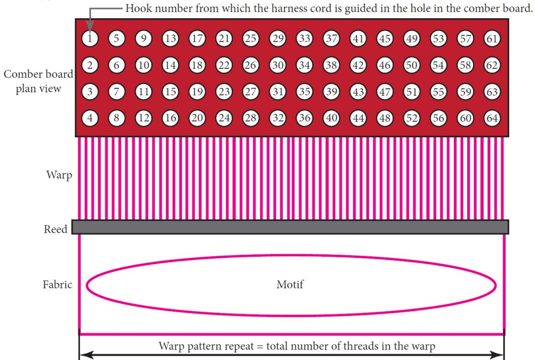
Figure 84: Plan view showing the guide of the harness cords in the comber board in case of creating a pattern across the width of fabric
