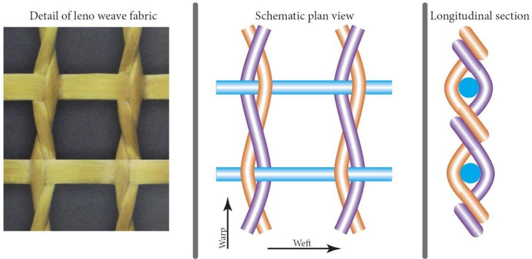
Figure 197: Detail of leno weave fabric, its schematic plan view and longitudinal section
