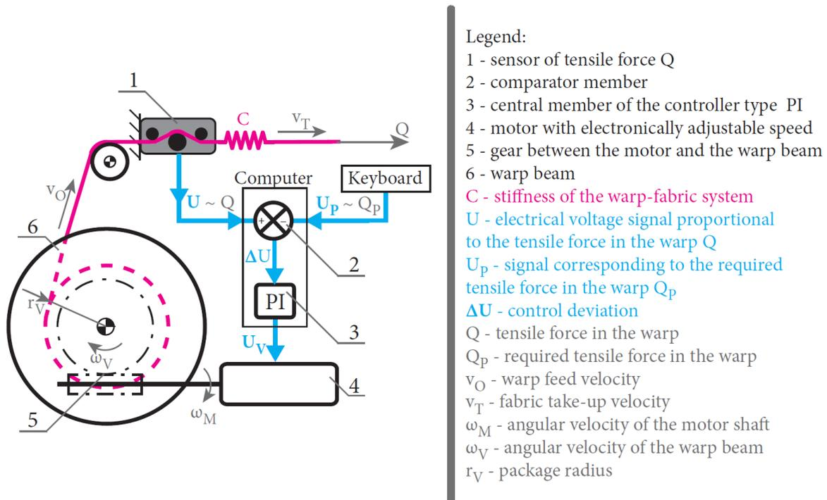
Figure 68: Diagram of the feedback circuit of the warp controller
