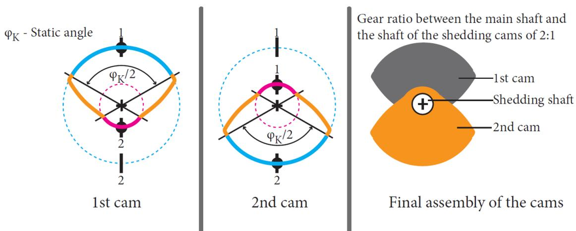
Figure 93: Last step of the procedure and final assembly of the cams for plain weave
