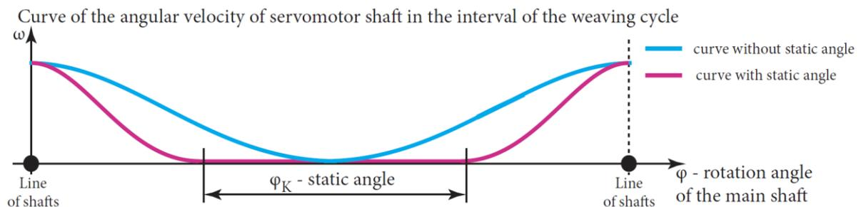
Figure 139: Example of the course of angular velocity of the servomotor in the interval of the weaving cycle
