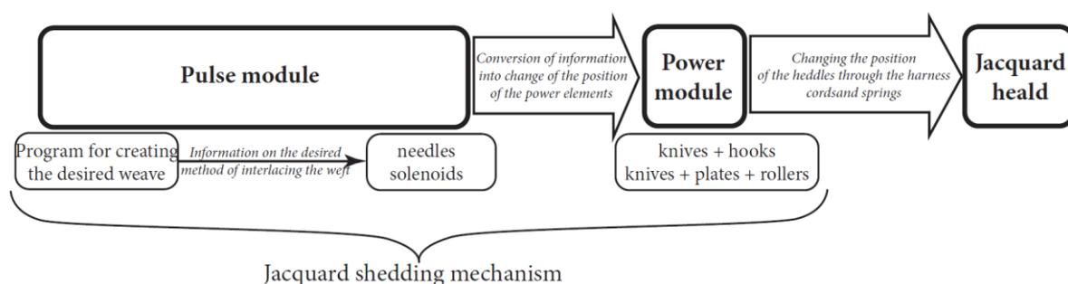
Figure 127: Block diagram of the main parts of Jacquard shedding mechanisms
