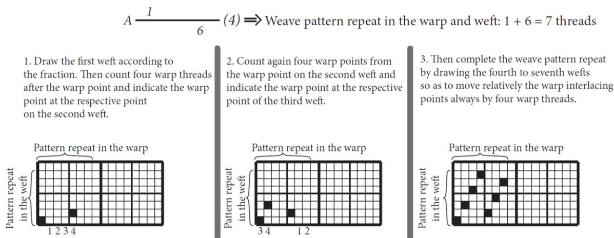
Figure 32: Drawing procedure for 7-harness satin weave with move numbers 4
