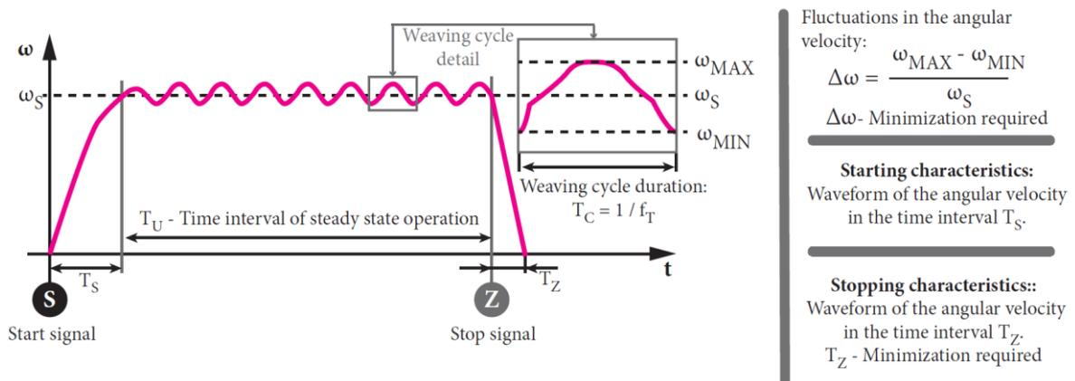
Figure 58: Angular velocity-time dependence: starting and stopping characteristics
