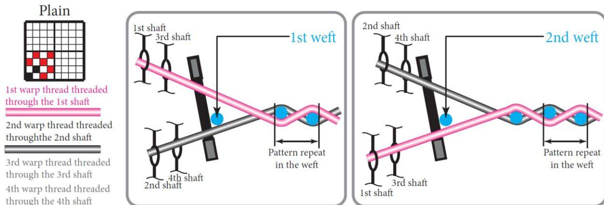
Figure 77: Diagram of the position of shafts in making a plain weave using four shafts with plain draft
