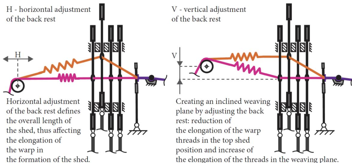
Figure 182: Horizontal and vertical adjustment of the feeding roller (back rest)
