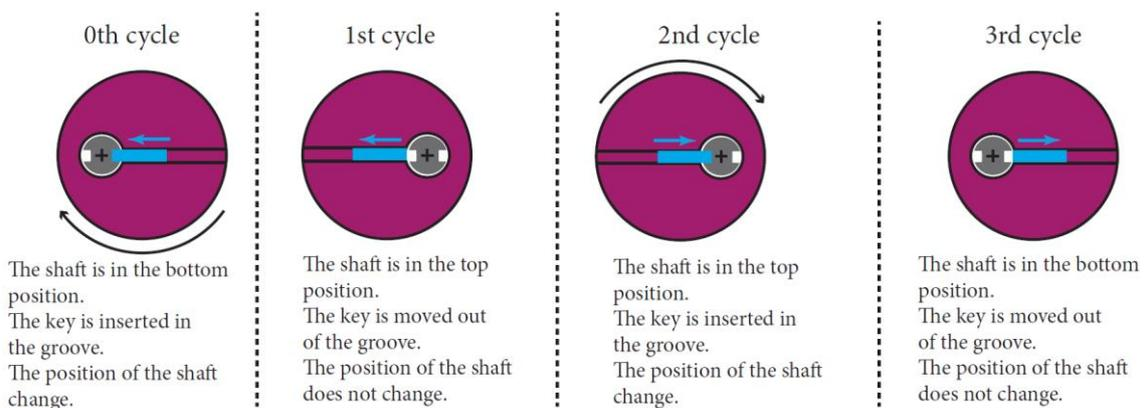
Figure 108: Tappet positions during three weaving cycles for the above described model situation
