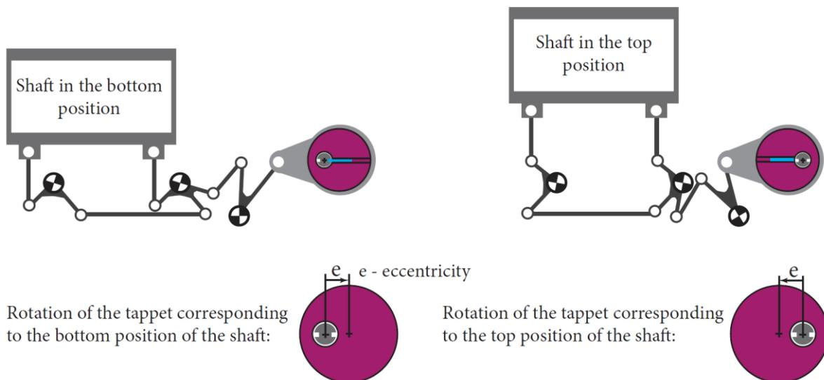
Figure 107: Tappet positions that correspond to the extreme positions of the shaft
