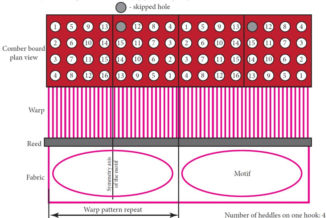
Figure 86: Plan view showing the guide of the harness cords in the creation of symmetrical patterns using the point tie
