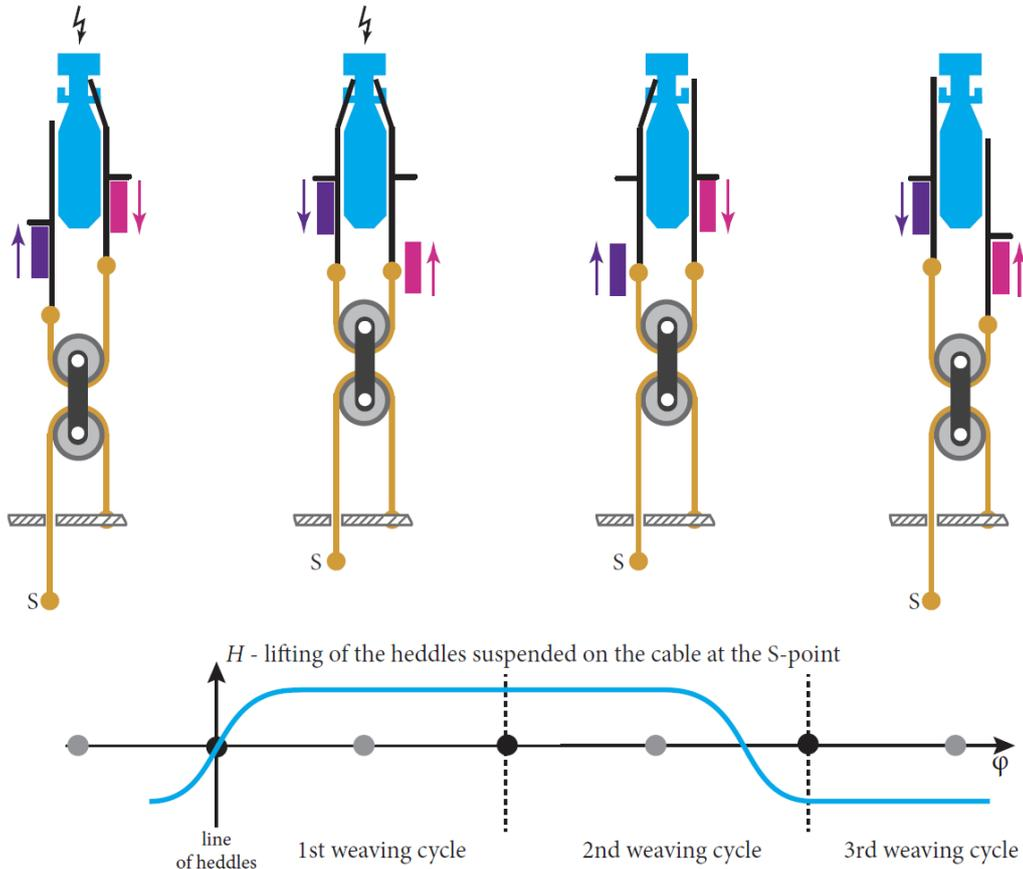
Figure 134: Positions of the plates and knives of the Bonas Jacquard mechanism during three weaving cycles
