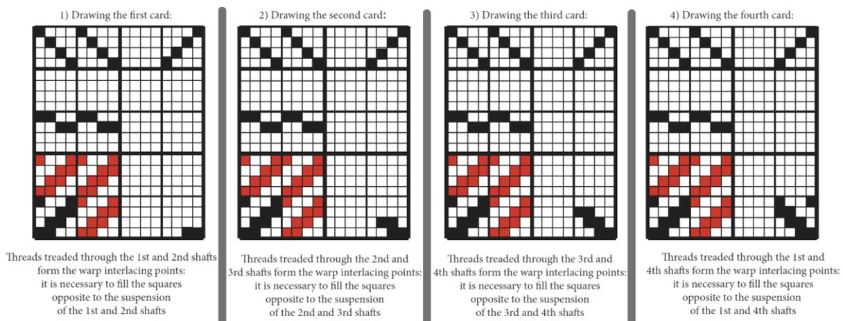
Figure 120: Procedure for drawing the cards for the above technical pattern
