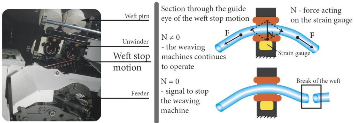
Figure 163: Weft stop motion on the Panter rapier machine (source [32]) and the principle of its function
