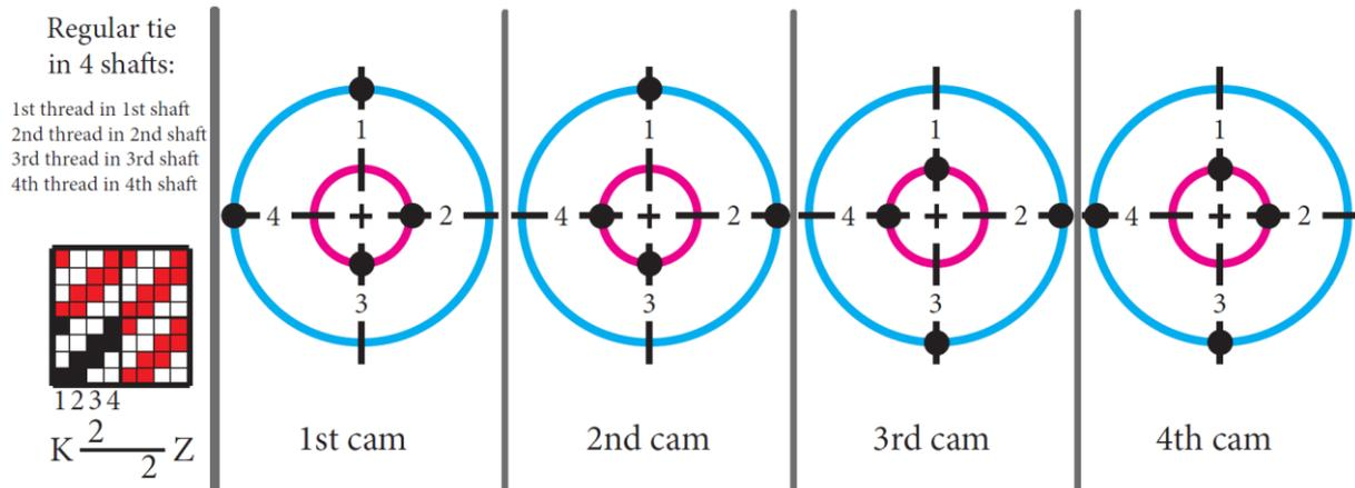
Figure 96: Second step of the procedure for drawing the shapes of cams for stitched 4-harness twill
