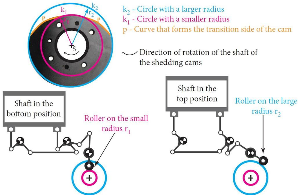
Figure 90: Parts of the shedding cam in the system of a pair of concentric circles
