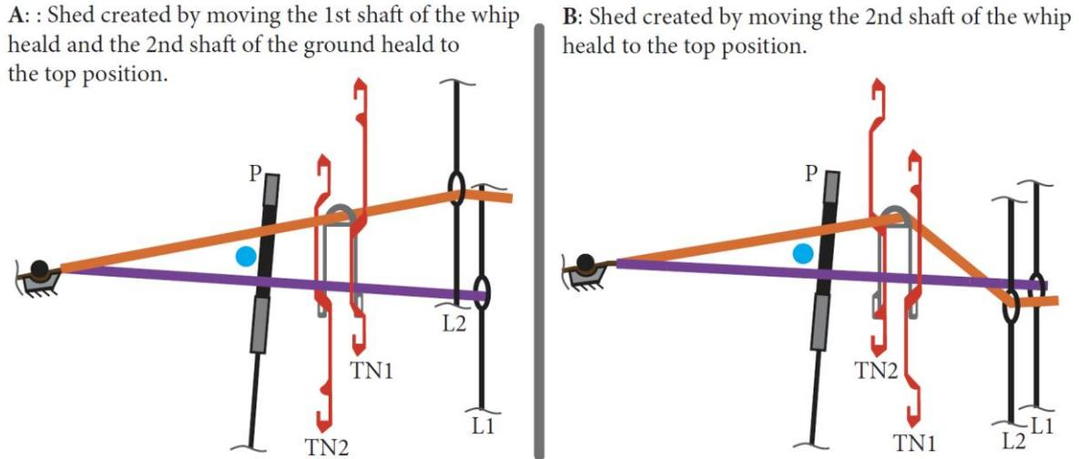
Figure 202: Leno heald with the open shed and weft insertion
