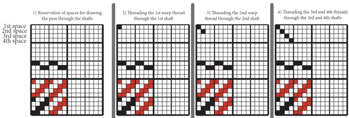
Figure 116: Procedure for drawing the pass through the shafts for the above technical pattern
