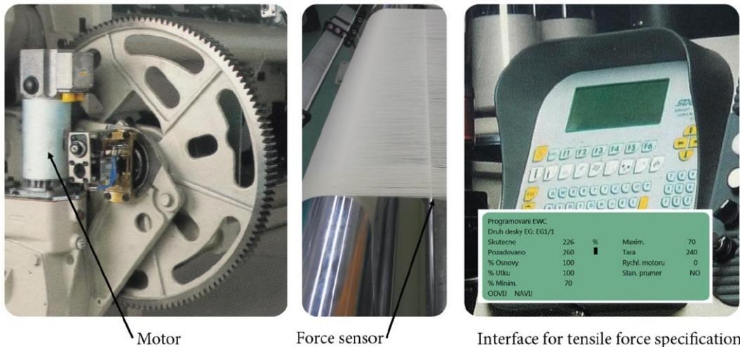
Figure 69: Photographs of the parts of warp controller of the Somet Excel machine
