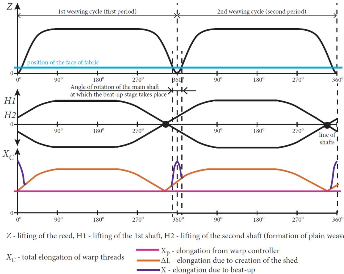
Figure 183: Dependence of the reed lifting, shafts and warp elongation on the rotation angle of the main shaft
