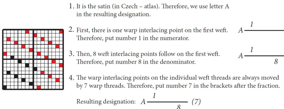
Figure 33: Procedure for writing the pattern according to the given weave (9-harness satin with move number 7)
