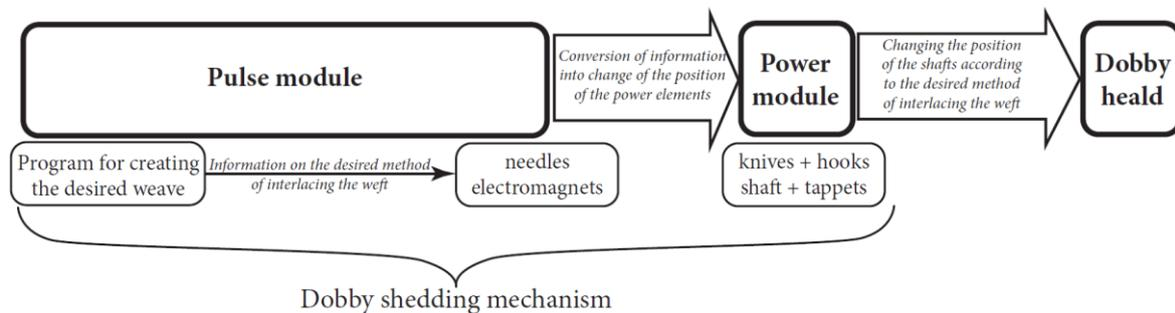
Figure 100: Block diagram of the main parts of dobby shedding mechanisms
