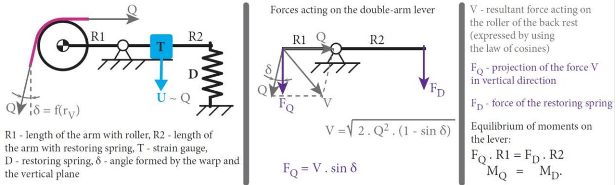
Figure 184: Single-roller free back rest
