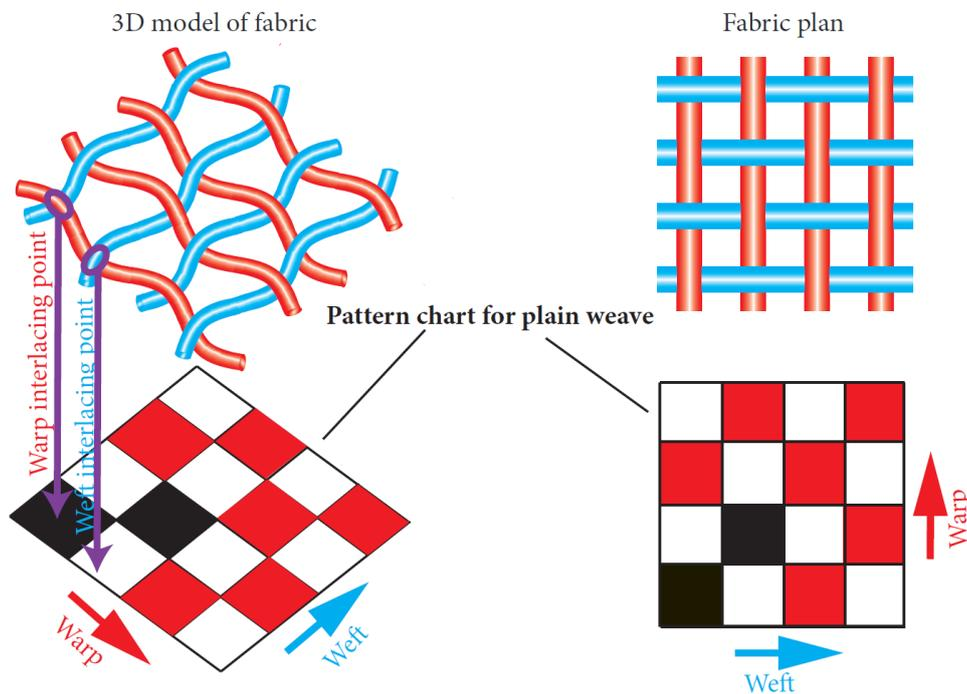
Figure 20: Method of indicating warp and weft interlacing points on the pattern chart paper (for plain weave)
