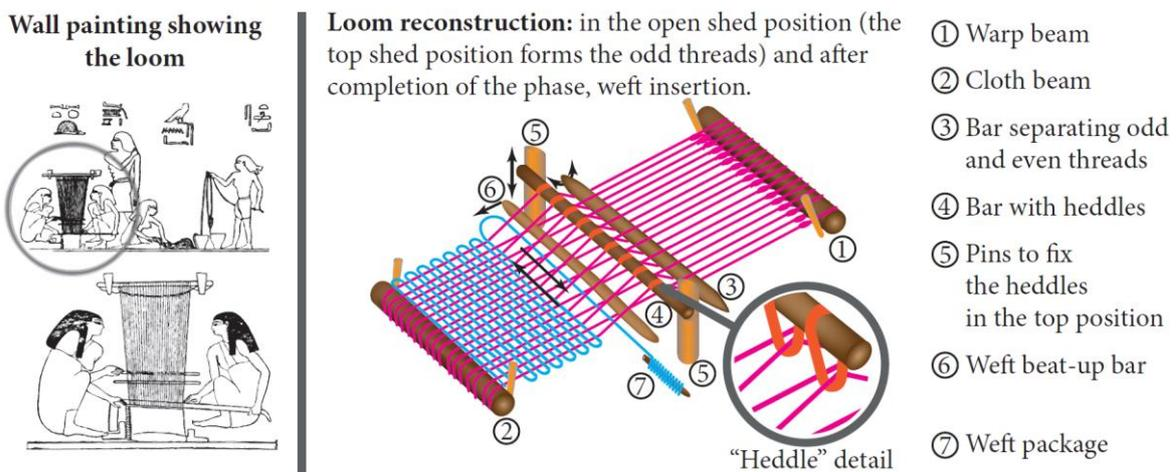
Figure 8: Scheme of Egyptian loom from the period of 5,000 BC
