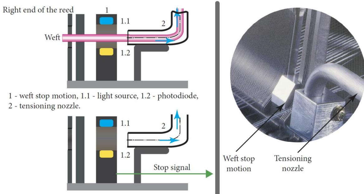
Figure 170: Weft stop motion and tensioning nozzle
