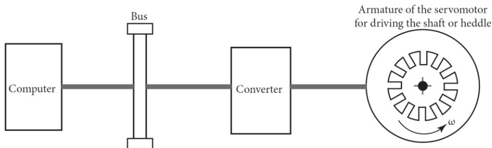
Figure 137: Diagram of the individual drive of shaft or heddle
