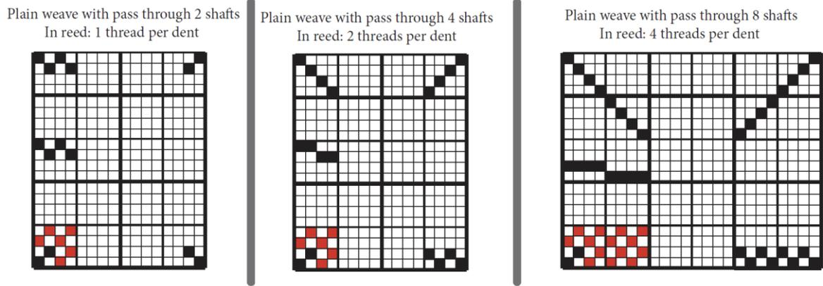
Figure 121: Technical patterns for plain weave with regular tie in different number of shafts
