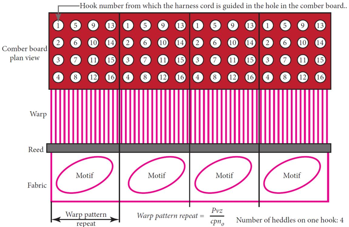
Figure 85: Plan view showing the guide of the harness cords in the comber board in case of repeating patterns (regular tie)
