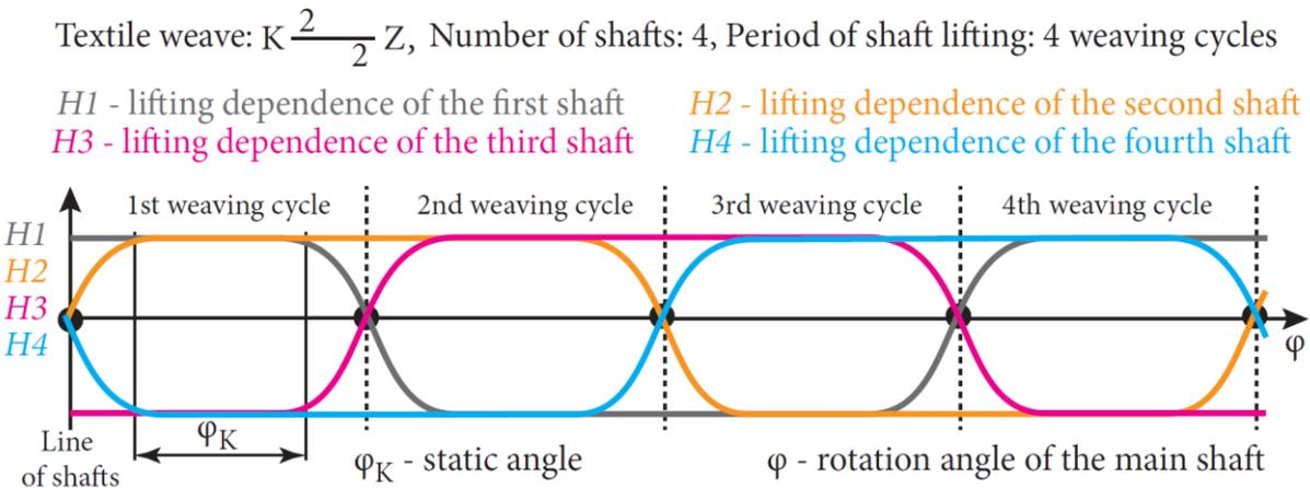
Figure 99: Lifting dependence of shafts during four weaving cycles for stitched twill
