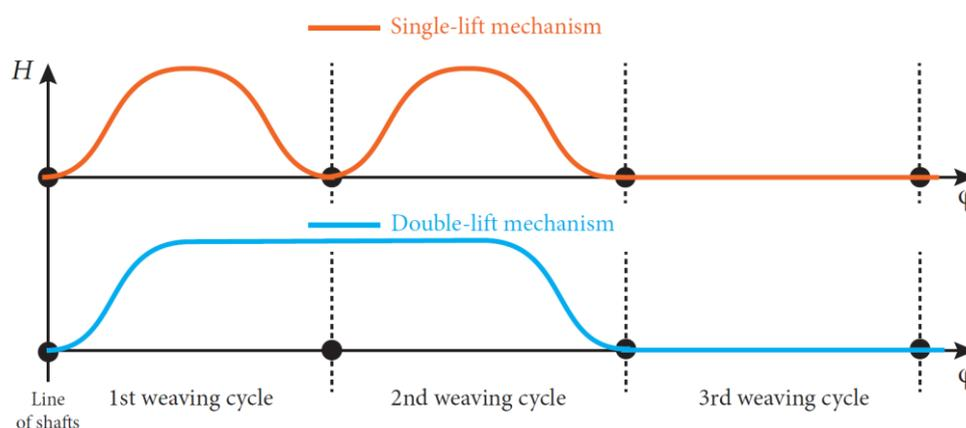
Figure 104: Course of shaft lifting during three weaving cycles, as described above
