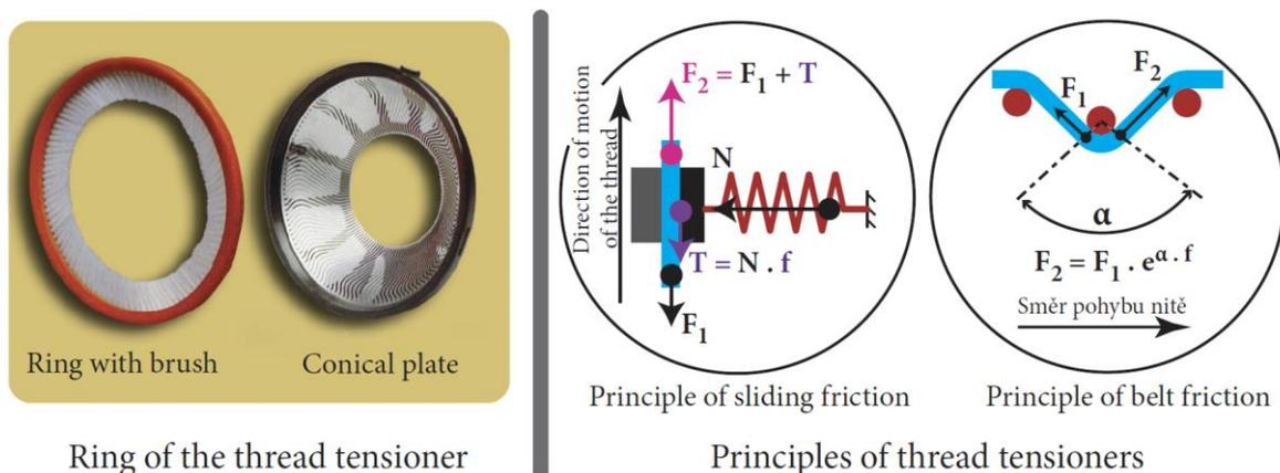
Figure 162: Rings of the thread tensioners and diagram of the principles of their functions
