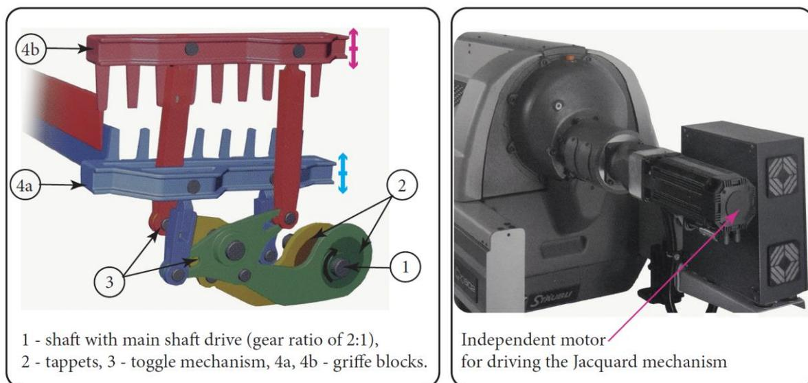
Figure 136: Jacquard device driving mechanism and independent drive (source [27])
