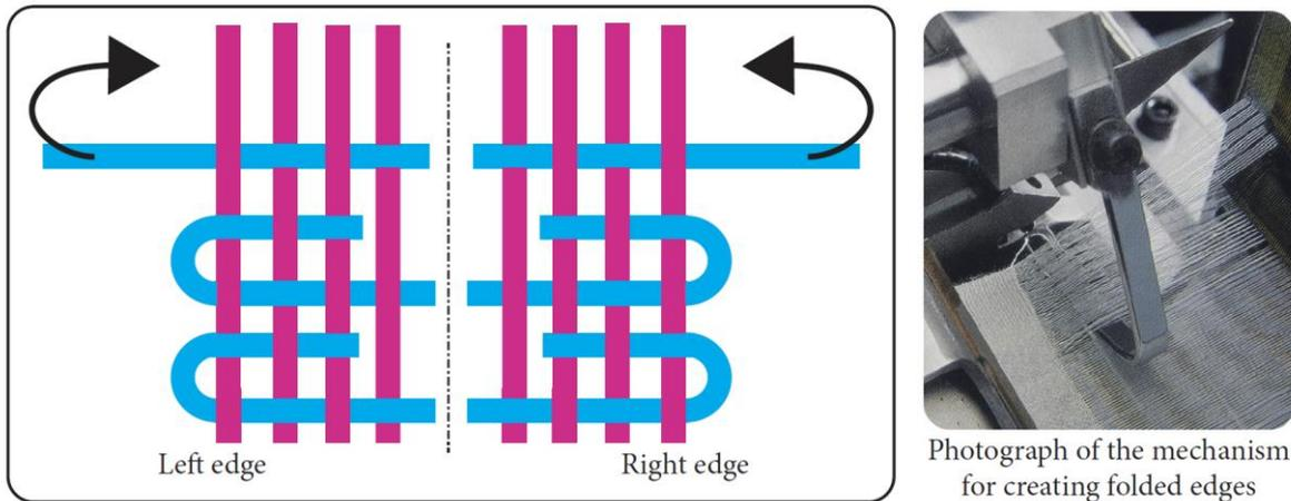
Figure 174: Reinforcing the edges of fabric by folding the edges of weft
