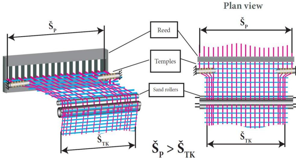
Figure 41: Reed width of fabric and fabric width on the cloth beam
