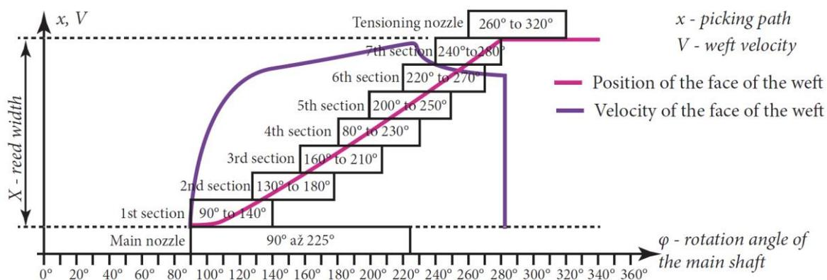
Figure 172: Valve timing and dependence of the weft velocity on the rotation angle of the main shaft
