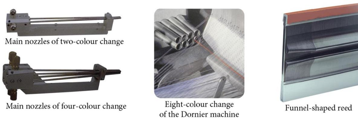
Figure 173: Main nozzles of the colour change of the air-jet weaving machines
