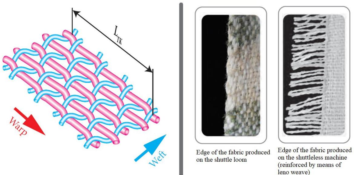
Figure 40: Fabric length and edge of fabric produced on shuttle loom and shuttleless machine
