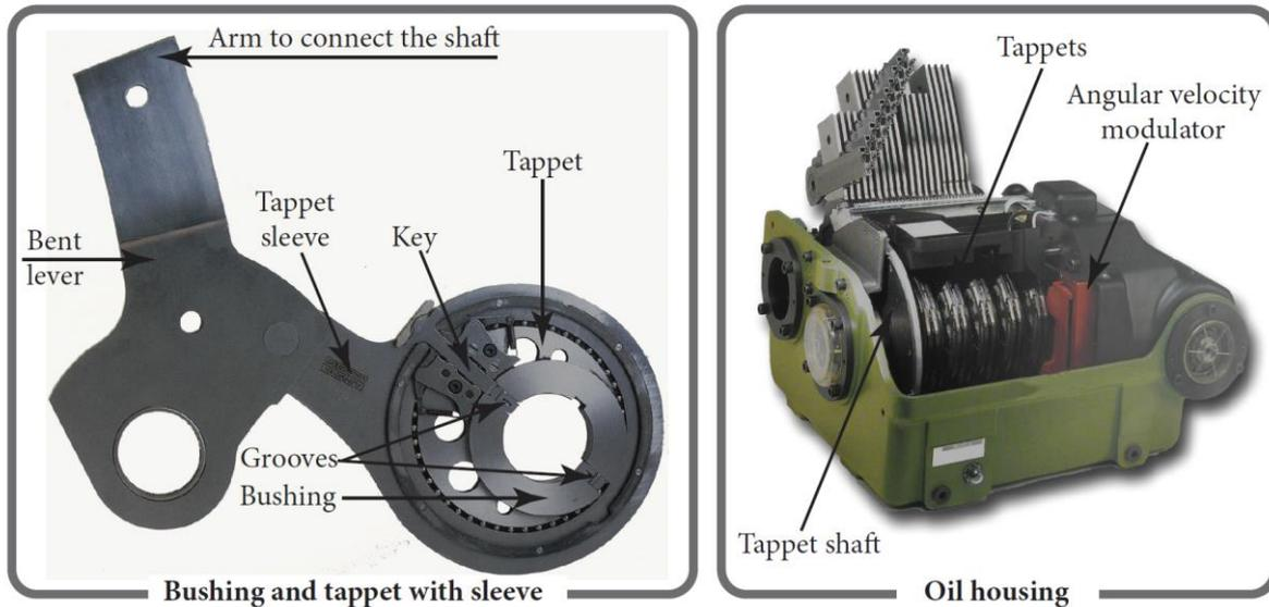
Figure 105: Main parts of the double-lift rotary dobby mechanism (source) [25]
