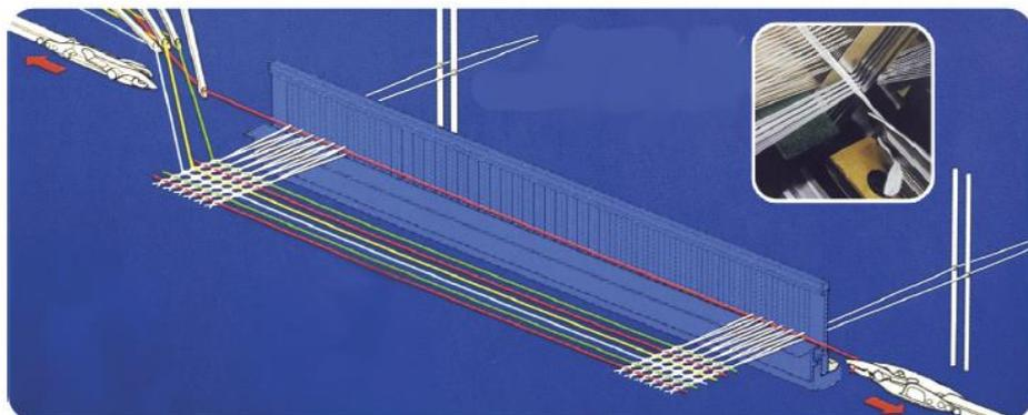
Figure 157: Diagram of the weft insertion by means of two rigid rapiers (source [30])
