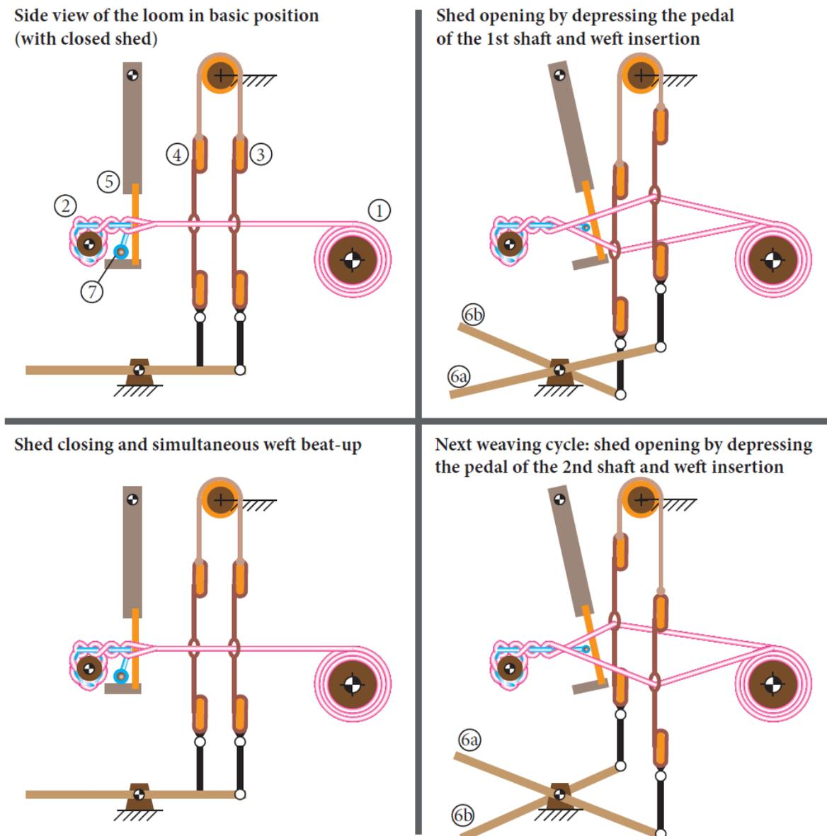
Figure 11: Phase of fabric production on the hand loom
