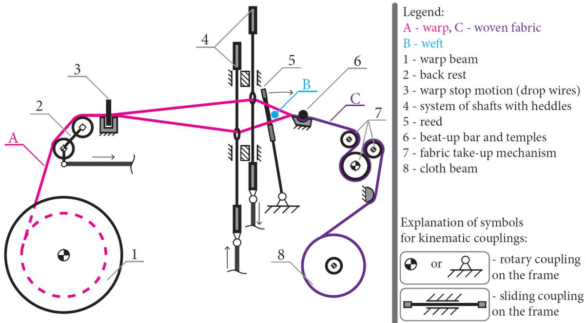
Figure 46: Basic diagram of the weaving machine
