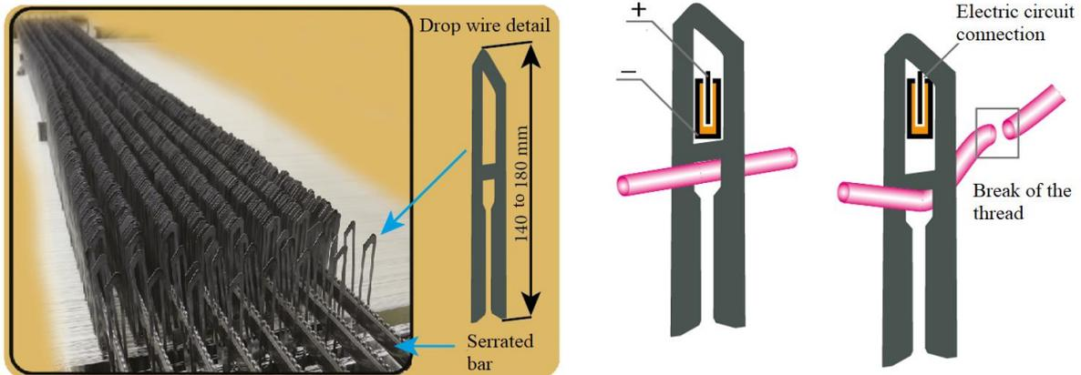
Figure 50: Drop wires of warp stop motion
