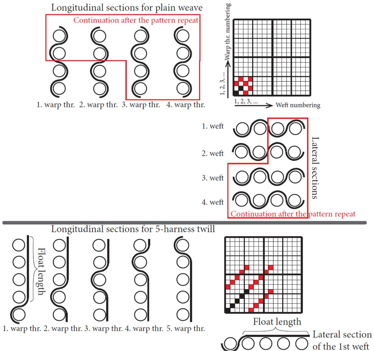
Figure 23: Representation of the lateral and longitudinal section through plain and twill weave
