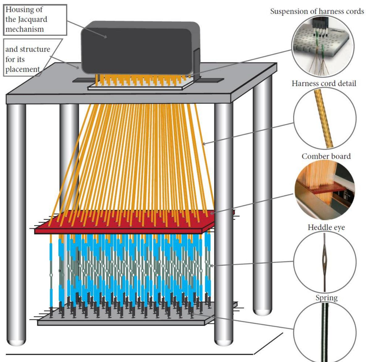
Figure 82: 3D diagram of the Jacquard heald - main parts and configuration
