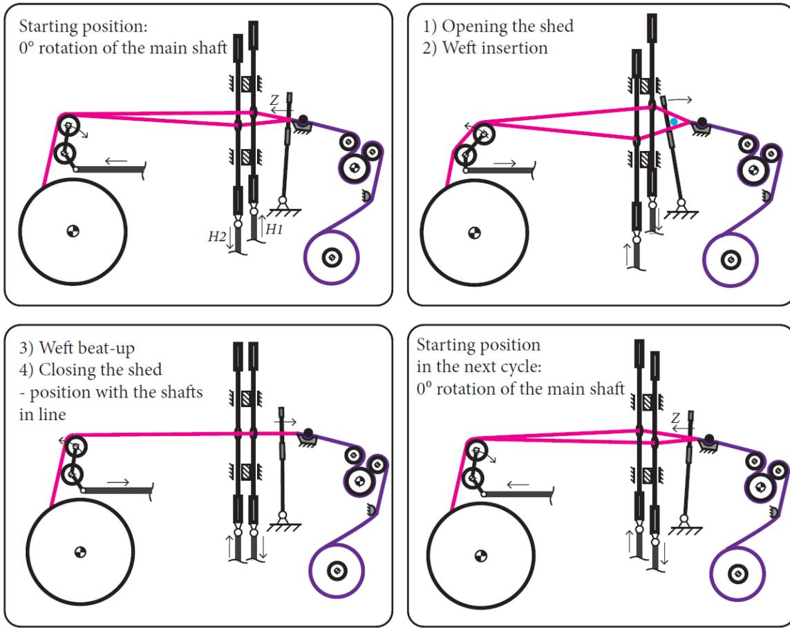
Figure 56: Phase of fabric production on the weaving machine
