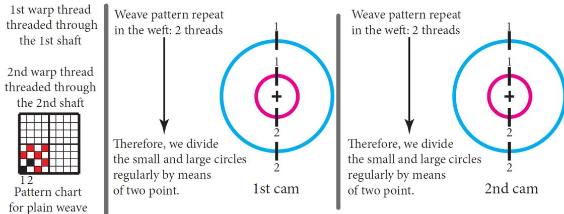
Figure 91: First step of the procedure for drawing the shapes of cams for plain weave
