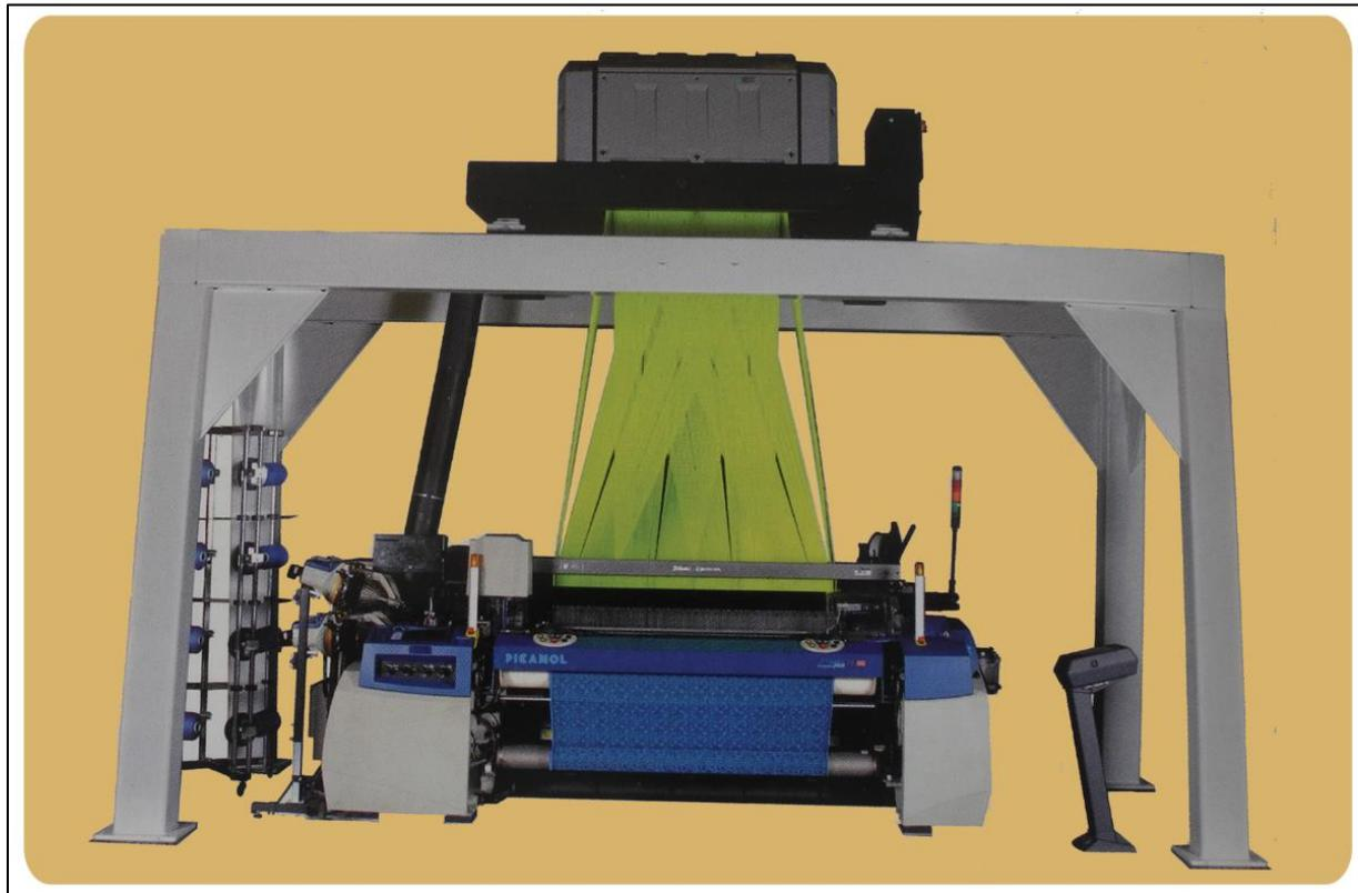
*Figure 87: Weaving machine equipped with the Jacquard shedding mechanism (source [16])*
