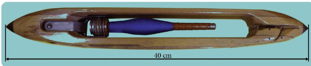
Figure 146: Plan view showing the weft insertion using a shuttle
