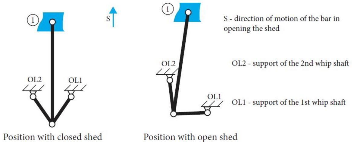
Figure 203: Forced motion of the bar using the fourbar mechanism (source [39])
