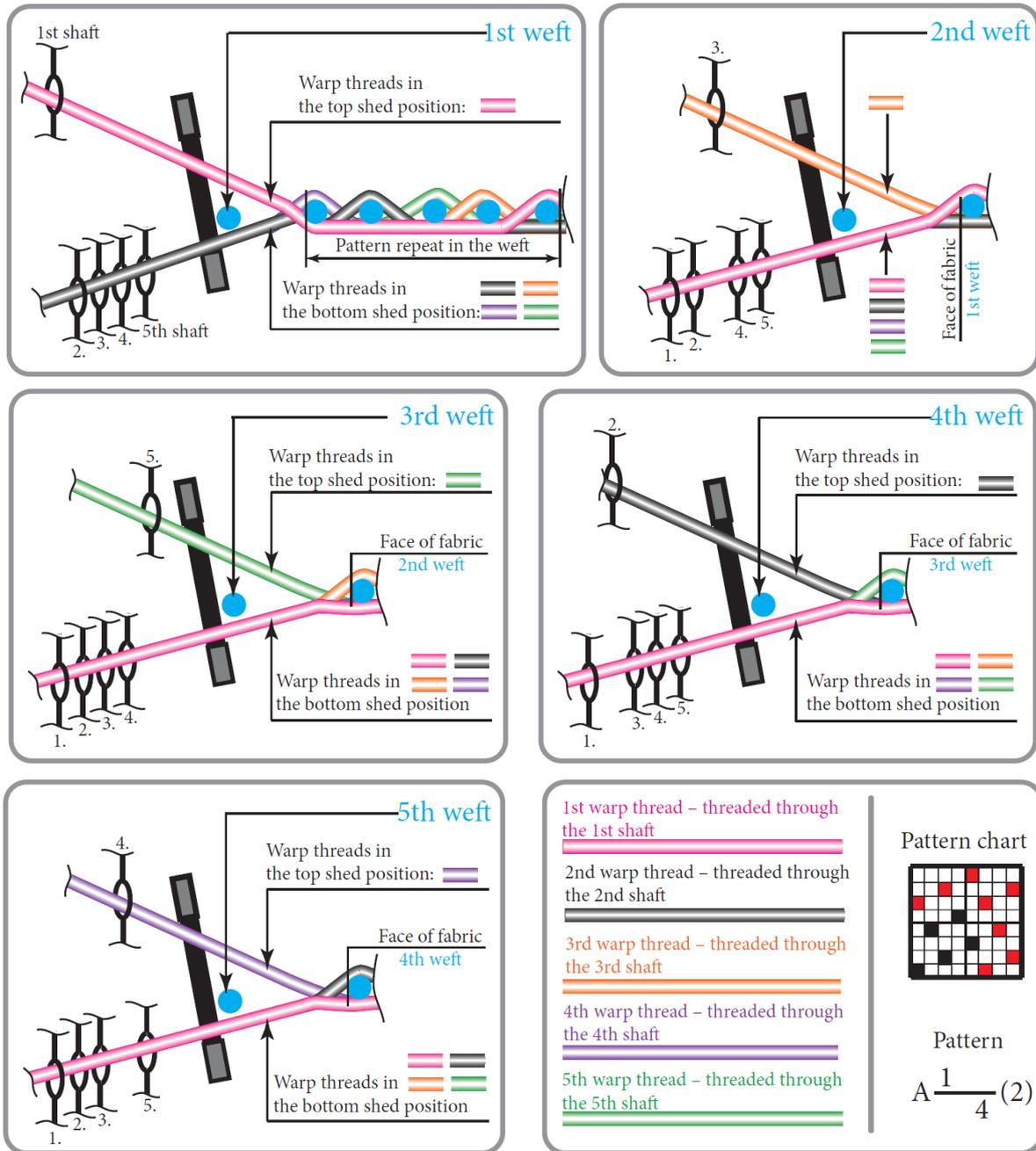
Figure 78: Diagram of the position of shafts in making a 5-harness satin using five shafts with plain draft
