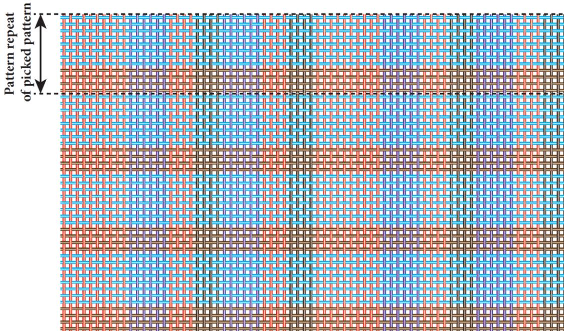
Figure 17: Scheme of checked fabric
