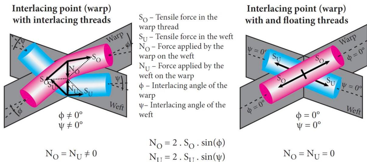
Figure 24: Action of forces between the warp and the weft in the interlacing point (warp) with interlacing and floating thread
