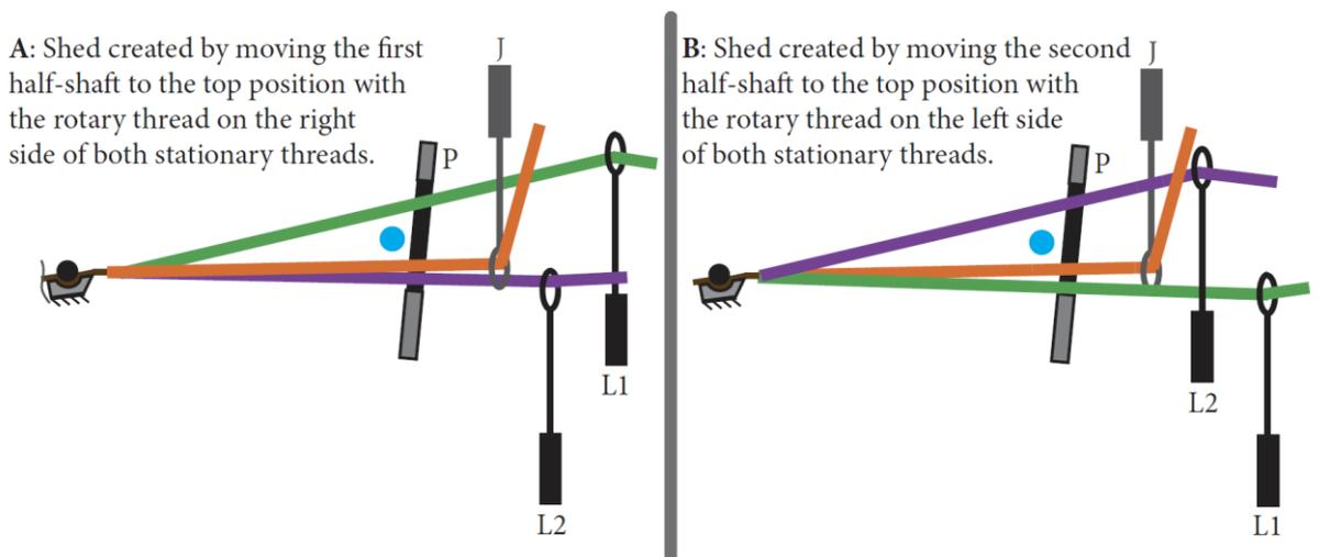
Figure 211: Rapier heald with the open shed and weft insertion - formation of the combined weave
