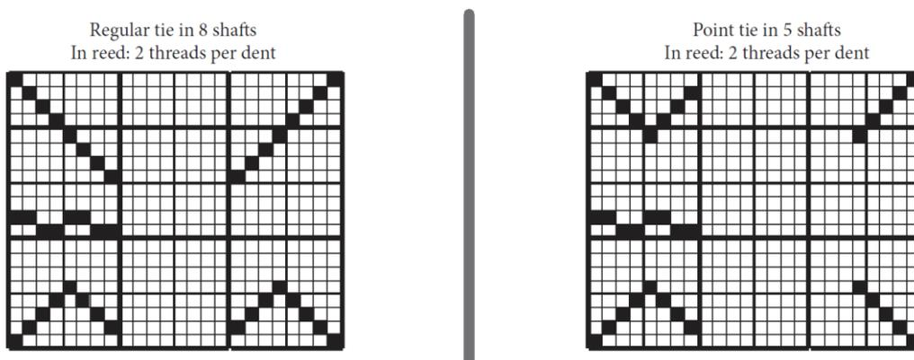
Figure 125: Technical patterns for longitudinal point twill
