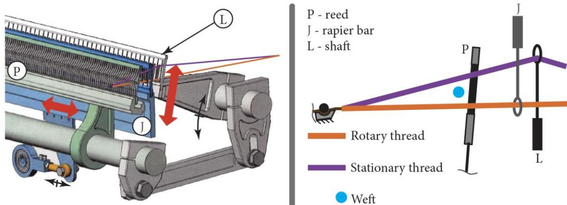
Figure 204: Diagram of the main parts of the rapier heald of the EasyLeno machine in the open shed position (source [30])
