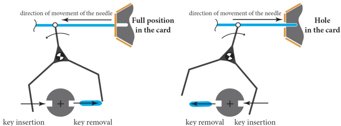
Figure 111: Positions of the triangle lever for the full position in the card and for the hole in the card
