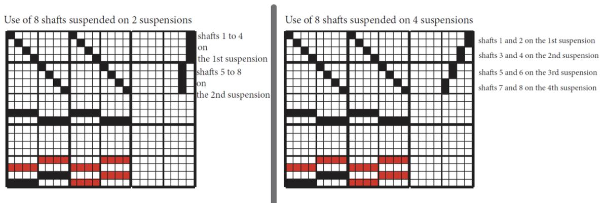
Figure 119: Examples of the suspension of shafts in technical patterns for longitudinal rib
