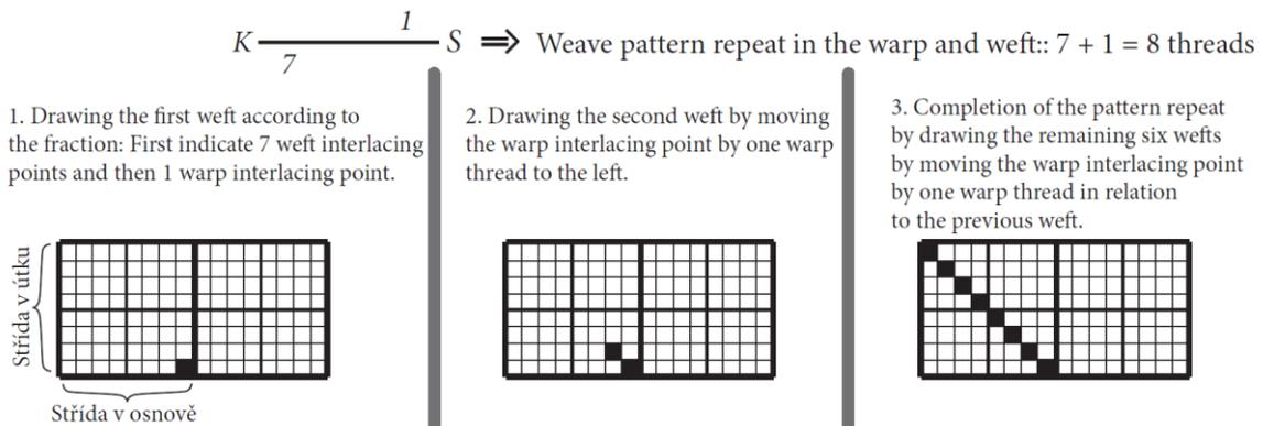
Figure 28: Procedure for writing the pattern according to the given weave (6-harness twill in the Z direction)
