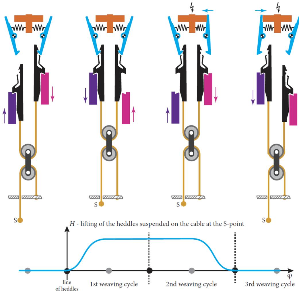
Figure 132: Positions of the hooks and knives of the Stäubli Jacquard mechanism during three weaving cycles as described above
