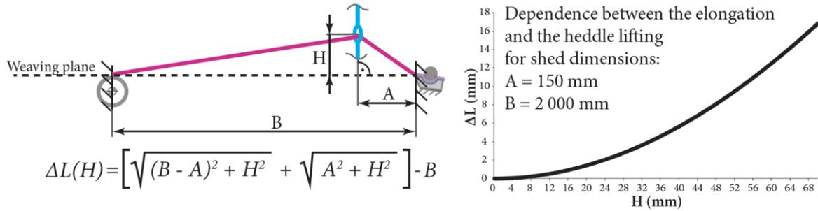
Figure 141: Diagram of the warp thread with the heddle and thread elongation-heddle lifting chart
