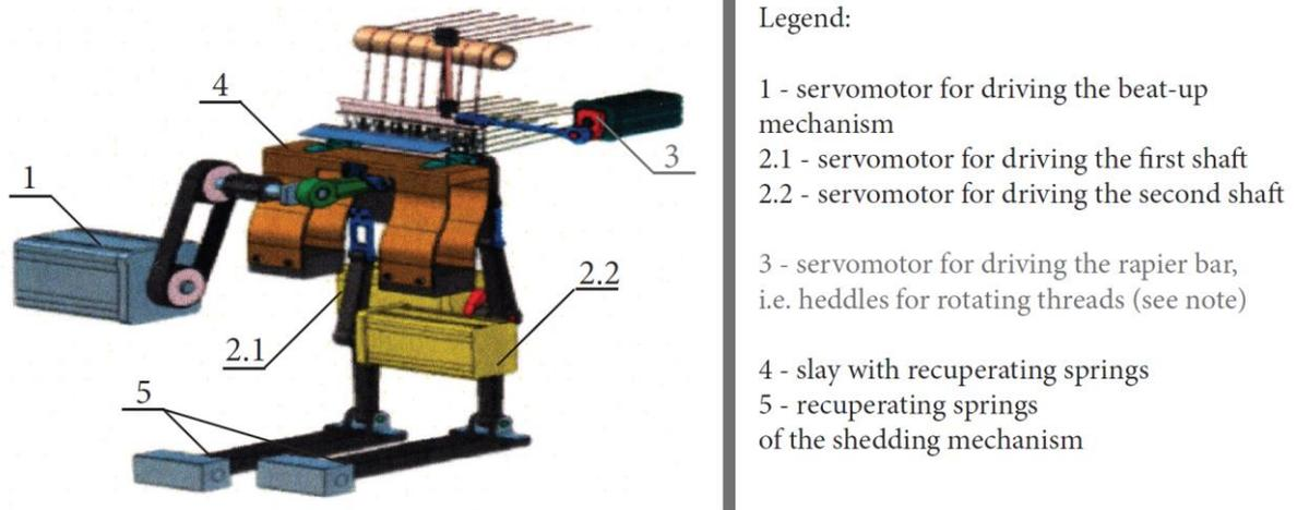
Figure 64: Drive of the Combine weaving machine (source [19])
