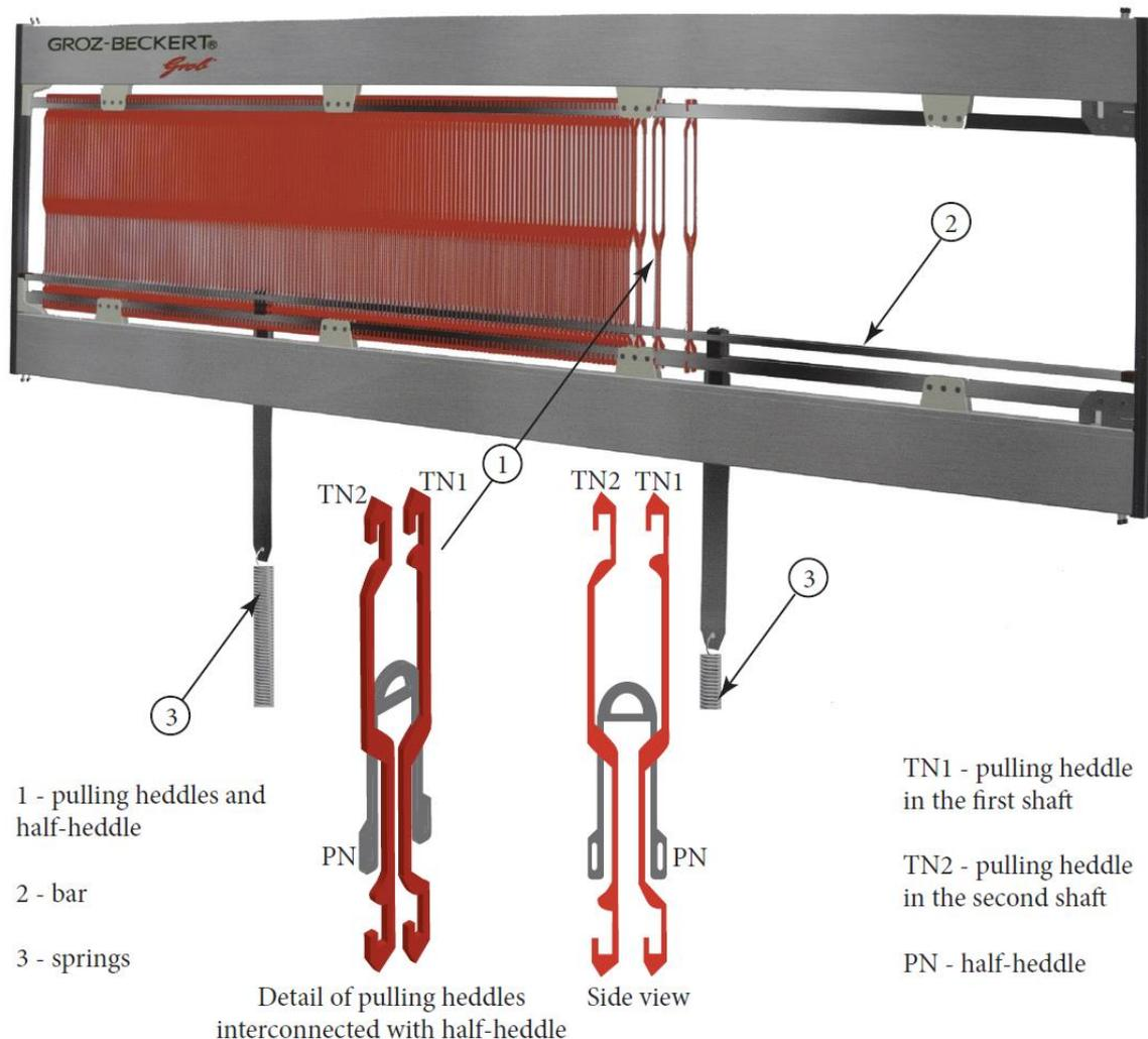
Figure 200: Main parts of the whip heald (whip double shaft)
