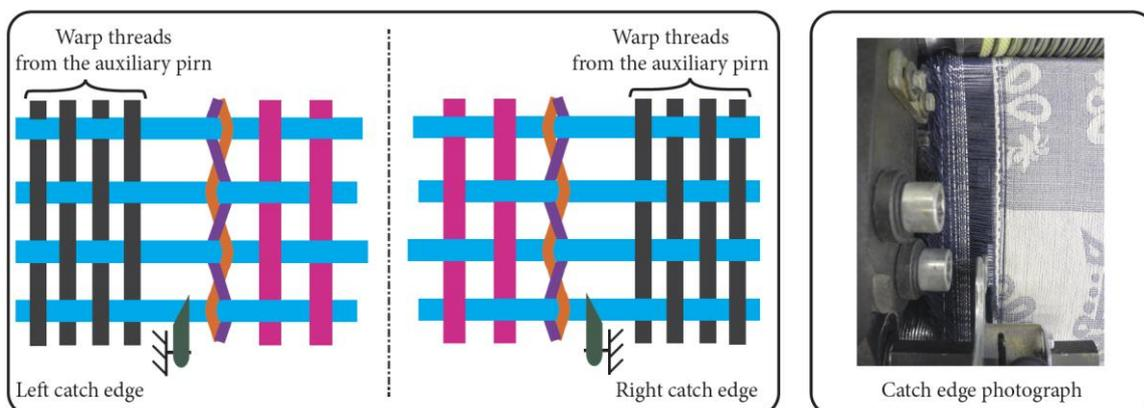
Figure 148: Catch edge of fabric on shuttleless machines
