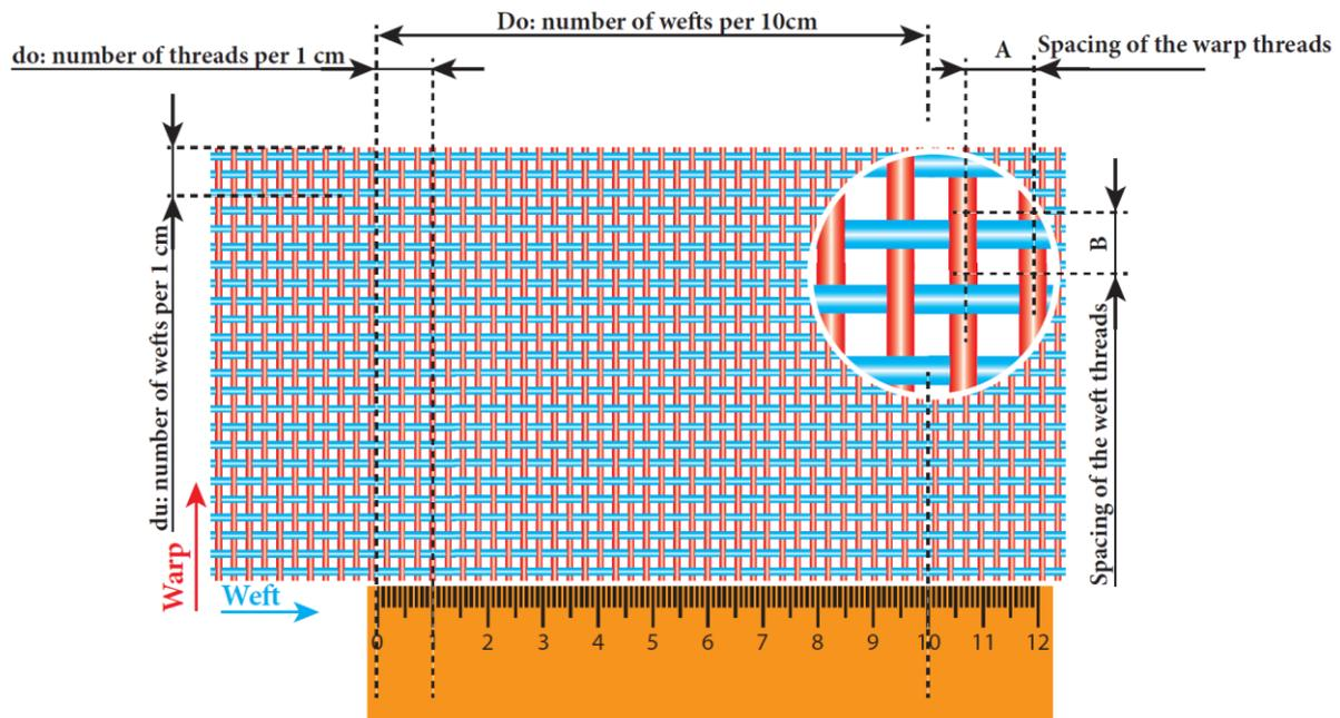
Figure 14: Number of warp and weft threads per unit length
