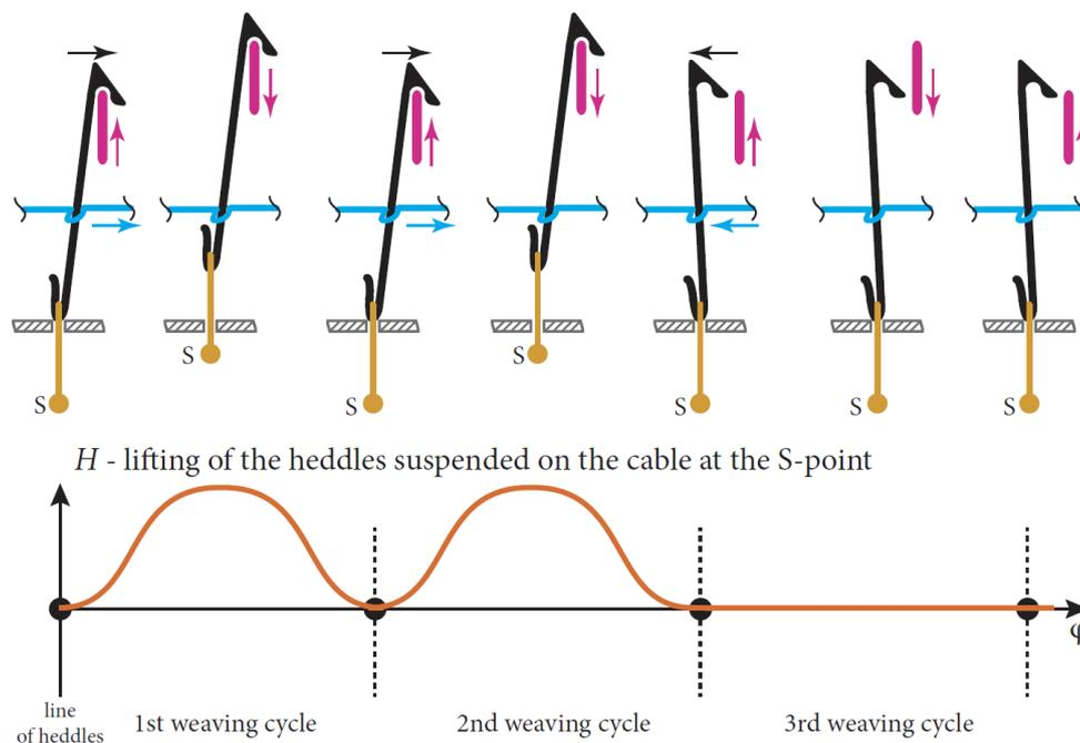
Figure 129: Positions of the hook and knife of the single-lift mechanism during three weaving cycles as described above
