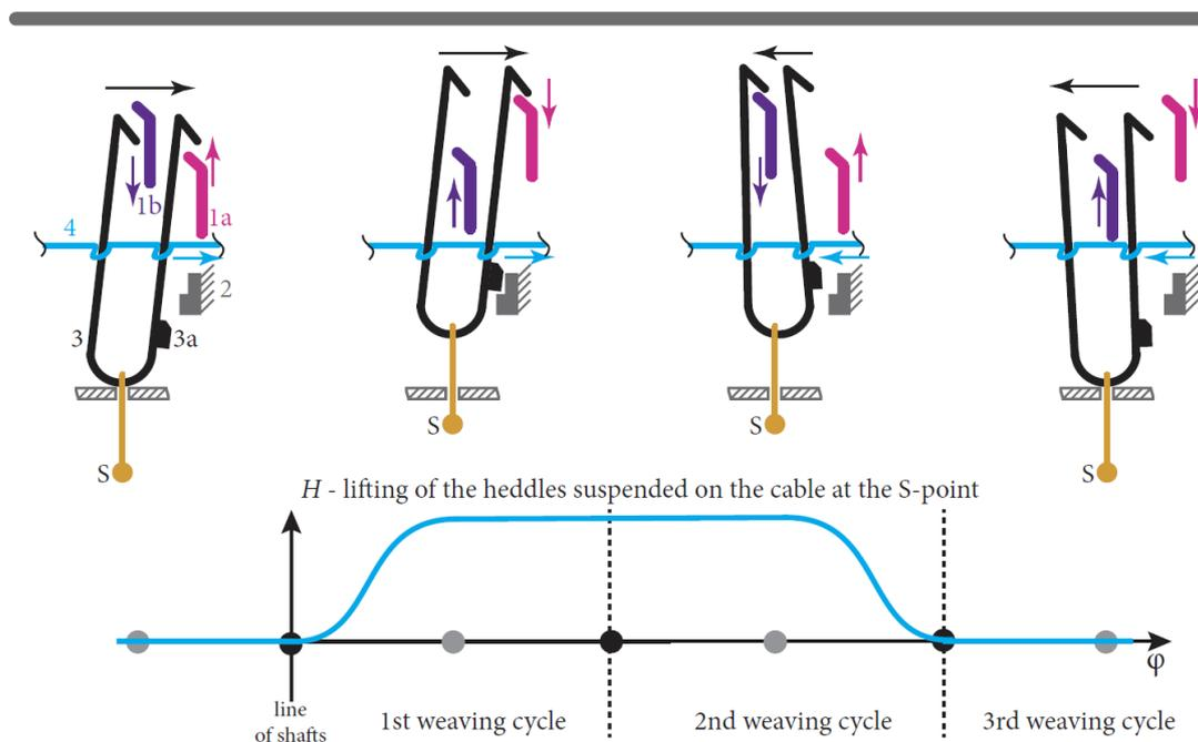
Figure 130: Positions of the hook and knives of the double-lift mechanism during three weaving cycles as described above
