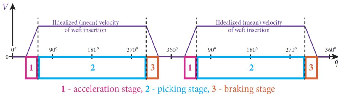
Figure 144: Weft insertion stages depending on the rotation angle of the main shaft
