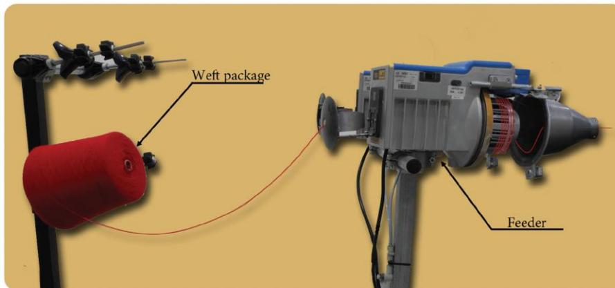
Figure 55: Cone with weft package and feeder
