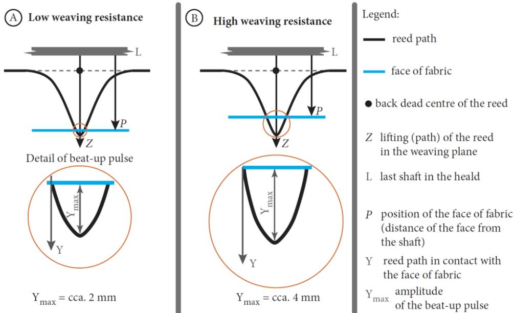
Figure 179: Plan view of the lifting of the reed with the position of the face of fabric for the various numbers of weft threads per unit length
