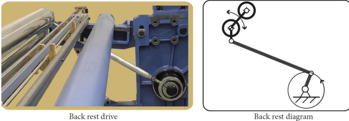
Figure 186: Back rest with forced drive
