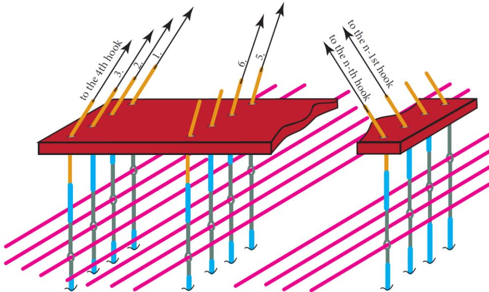
Figure 83: 3D diagram of threading the warp threads in the Jacquard heald
