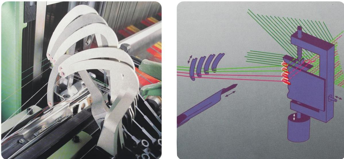
Figure 164: Photographs of the colour change feeders and diagram of four-colour change (source [14])
