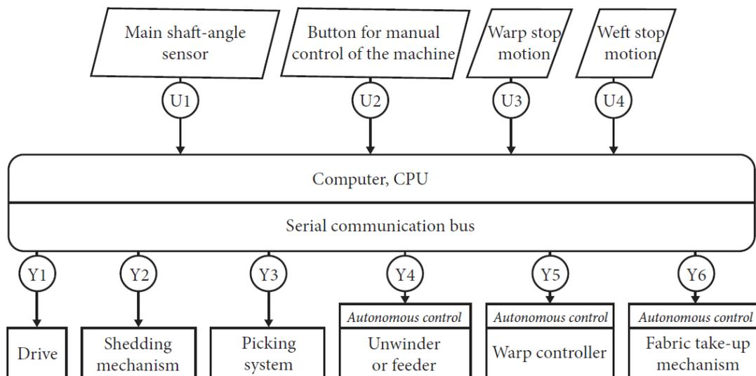
Vstupní signály: U1 - digital signal, which determines the angle of rotation of the main shaft
