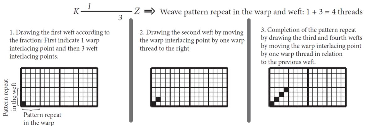
Figure 27: Procedure for drawing 4-harness twill as indicated (according to the pattern)
