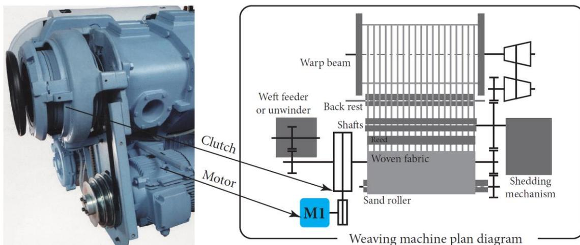
Figure 60: Structure of the drive type A, photographs of the motor and the mechanical clutch on the main shaft (source [14])
