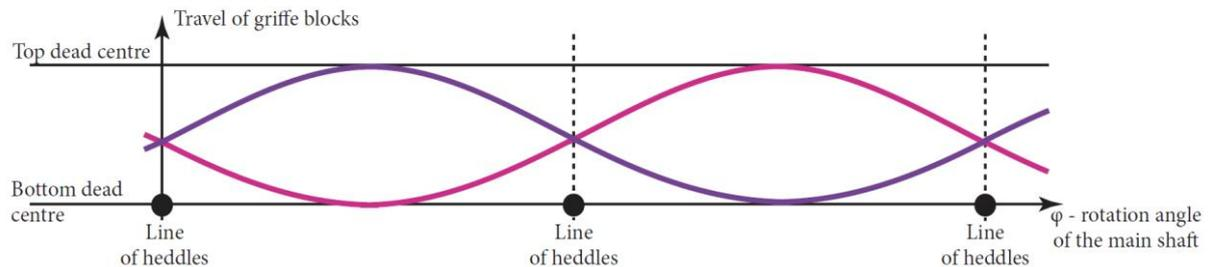
Figure 135: Lifting dependence of the griffe blocks of the double-lift Jacquard mechanism
