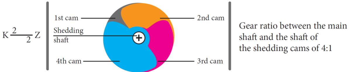
Figure 98: Final assembly of the cams for stitched 4-harness twill
