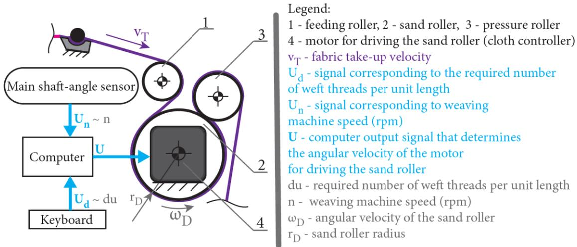
Figure 70: Fabric take-up (cloth controller) diagram
