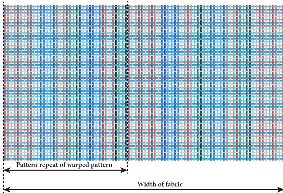
Figure 15: Scheme of fabric with warped pattern
