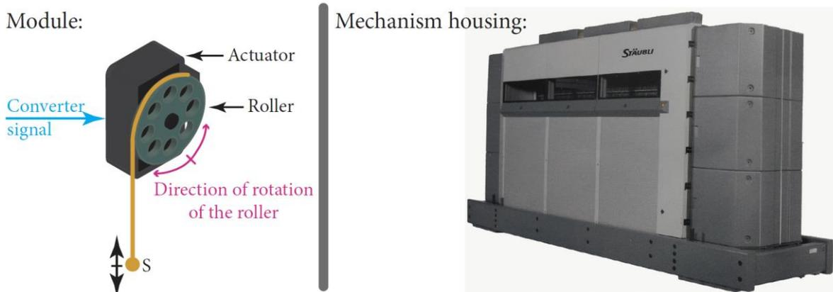
Figure 140: Main parts of the Jacquard mechanism with actuators (source [27])
