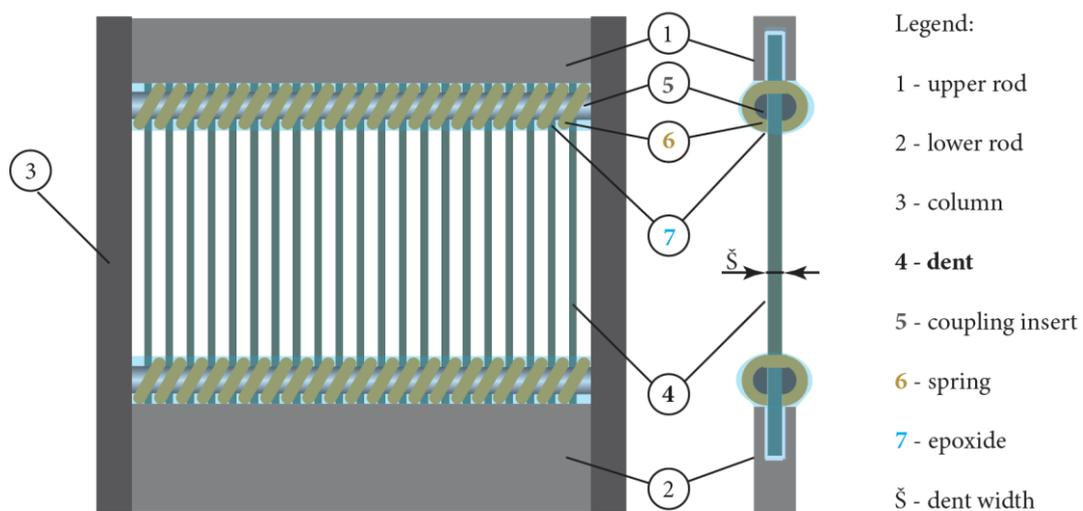
Figure 176: Diagram of the main parts of the reed (front and side views)
