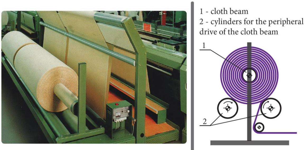
Figure 73: Winding fabric outside the weaving machine (winder)
