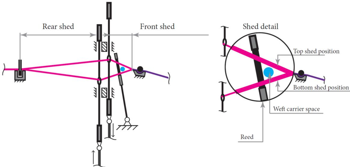
Figure 74: Diagram of the shed with dobbie heald, which consists of two shafts
