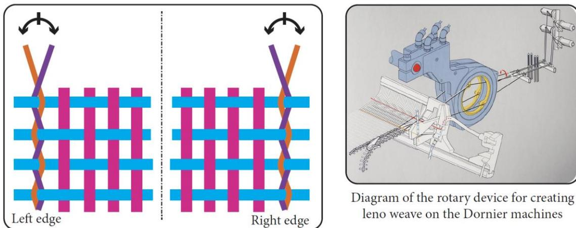
Figure 175: Reinforcing the edges of fabric by leno weave
