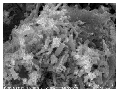
Figure 2: SEM analysis shows the crystalline structure of \text{TiO}_2 fibers annealed at 1000 °C in argon.
