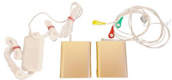
Fig. 1: Two pieces of the Wearable Telehealth Multi-Sensor Monitors. On the left, the monitor with a connected sensor for measuring respiratory activity. In the right, the monitor with cables for ECG chest electrodes.
