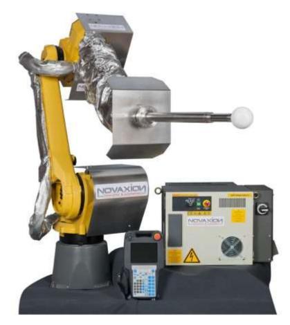
Fig. 8.13 Example of a ball-gatherer feeder (source: NOVAXION)
