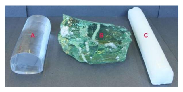
Fig. 3.8 Glass crystallization: A – clear glass pressing rod without visible crystallization, B – fragment of glass from a tank furnace with appreciable crystallization after heterogeneous nucleation, C - opal pressing rod with crystallisation after homogeneous nucleation
