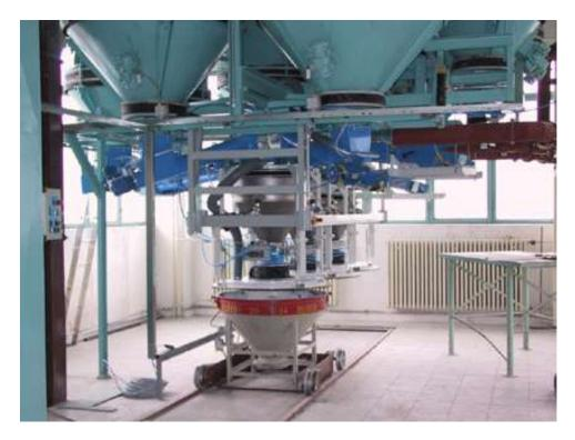
Fig. 5.3 View of the actual part of machinery of the batch house, the lower part of containers, raw material feeders, weigher, container (source: Dites spol. s r.o.)
