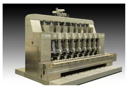
Fig. 9.24 Container glass forming machine type ISS (source: Sklostroj Turnov CZ, s.r.o.)
