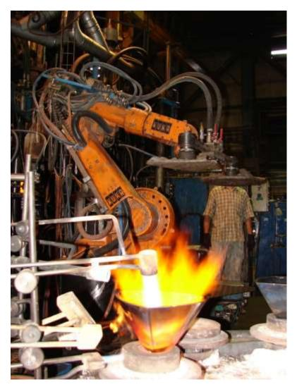
Fig. 11.29 Angular Kuka robot for handling in vase polishing
