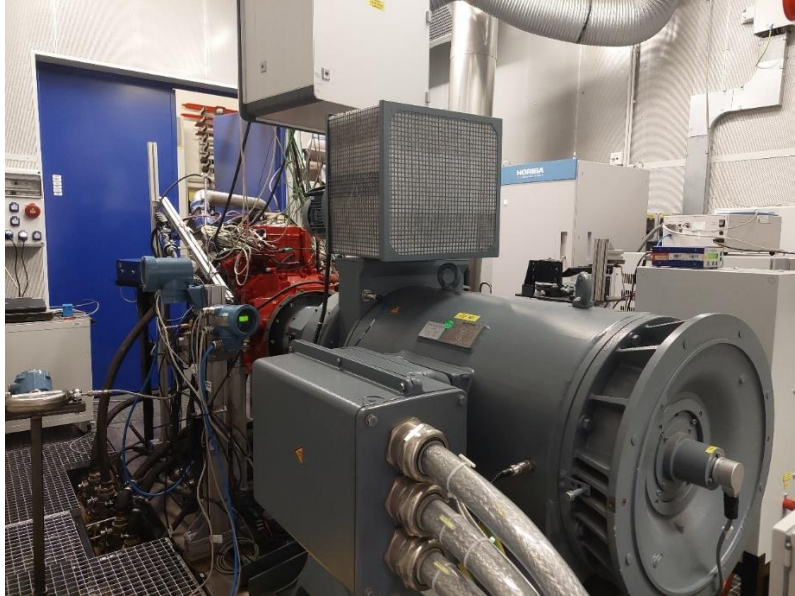
Figure 2: Functional sample of a dual-fuel engine in the laboratory
