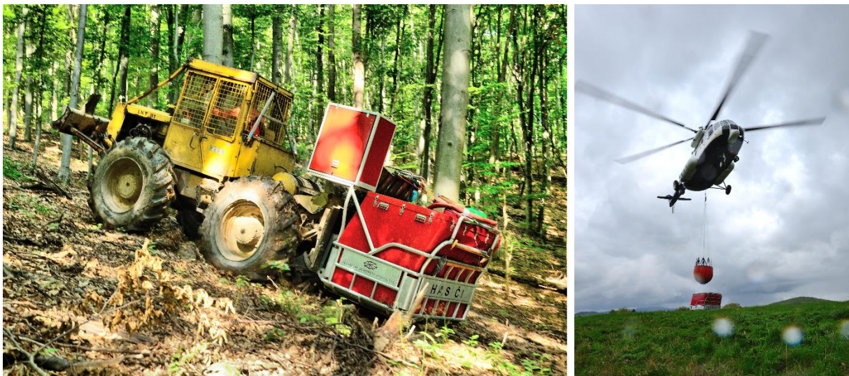
Figure 1: The firefighting adapter based on skidder with front axle oscillation. Filling the water tank with Bambi bucket.
