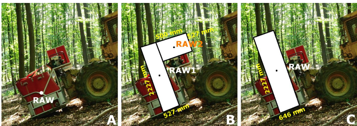
Figure 6: Original water tank and its simplified possible shape modifications. RAW, RAW1, RAW2 – Centers of gravities, and dimensions for 2000 l water tanks (see also Tab.1). Width is 1390 mm for all the tanks.
