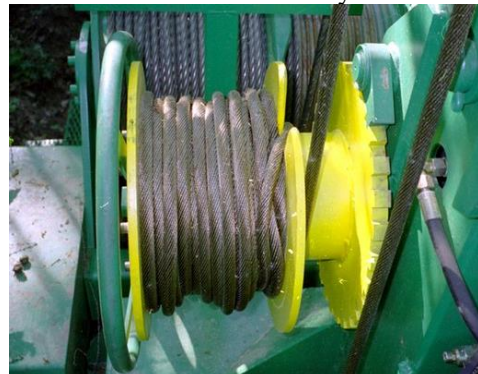
motor driven cable tightening
