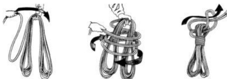
Fig. 73. Procedure of folding textile cables to scrolls
