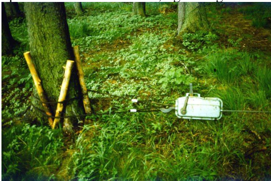
skyline tightening by manual winch
