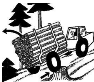
Fig. 113. Hitting a stump can result in machine overturning or damage to trees next to the line
