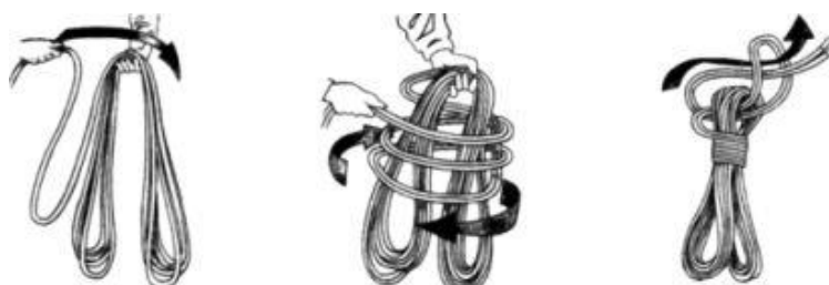
Fig. 65. Procedure of plaiting the textile rope into the scroll
