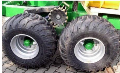
Fig. 104. Non-driven and pinion-driven bogie axle
