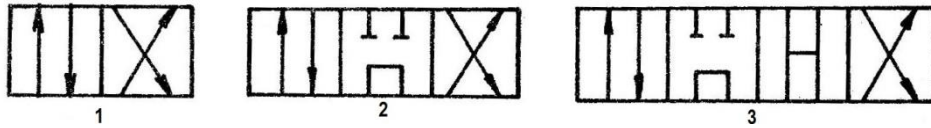
1 – two-position, 2 – three-position, 3 – four-position Fig. 41. Examples of four-way distributor schematics
