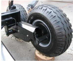
Fig. 104. Non-driven and pinion-driven bogie axle
