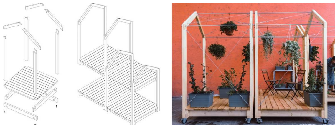
Fig. 1: Technical details of the structure and a photo from the opening day
