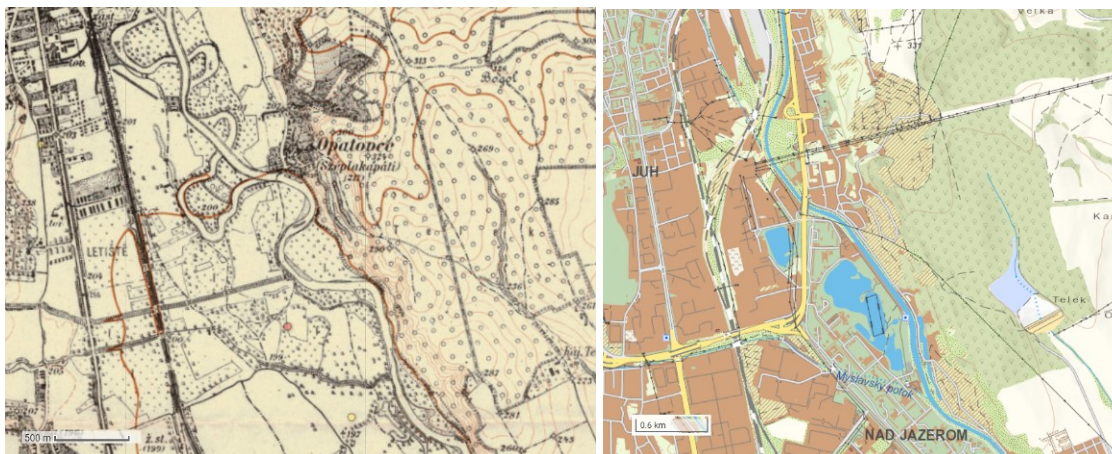
Fig. 1: Comparison of stream-channel regulation of the Hornád river in the Košice. (Left map: The military mapping in 1920 – 1950. Right map: ZBGis map 2023)
