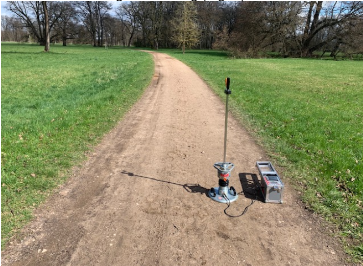
Fig. 3: View of the impact load test measurements on the pavement surface.
