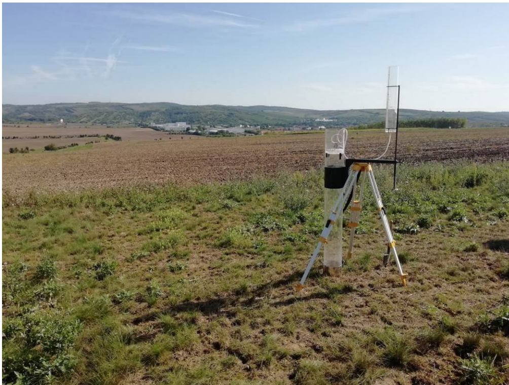
Fig. 5: Measurement of infiltration properties on the anti-erosion grass strip
