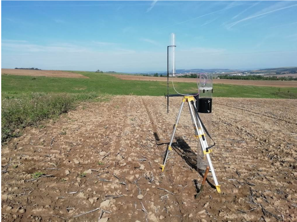
Fig. 4: Measurement of infiltration characteristics on arable land in the vicinity of an anti-erosion grass strip
