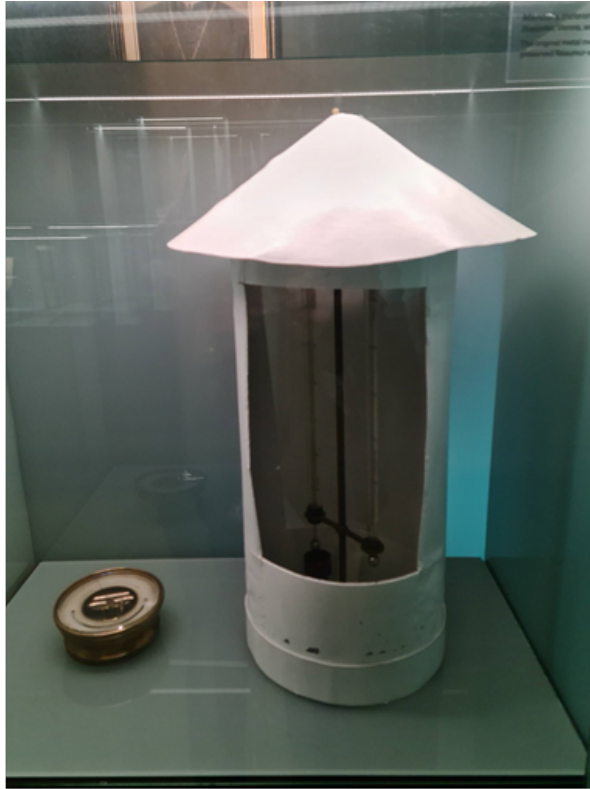
Fig. 2: A replica of the tin meteorological booth in the Mendel Museum exposition
