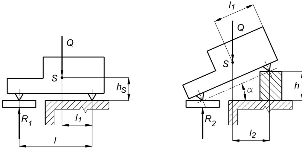
Fig. 1.1 Determining the centre of gravity
