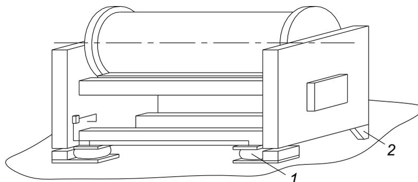
*Fig. 3.6 Flexible mounting of the loom: 1-pneumatic spring, 2-rubber spring*
