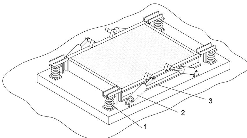
*Fig. 3.3 Flexible machine base: 1-springs, 2-dampers, 3-frame.*
