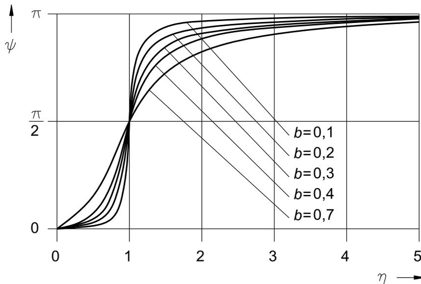
Fig. 1.15 Phase characteristics
