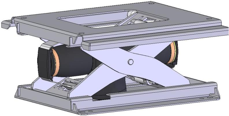
*Fig. 3.10 Pneumatic pedestal of driver's seat with adjustable natural frequency*
