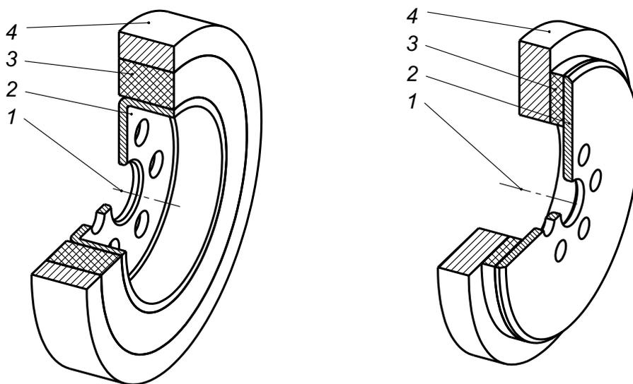
Fig. 2.11 Rotary damper: 1-axis of rotation, 2-disk, 3-rubber spring, 4-damping mass
