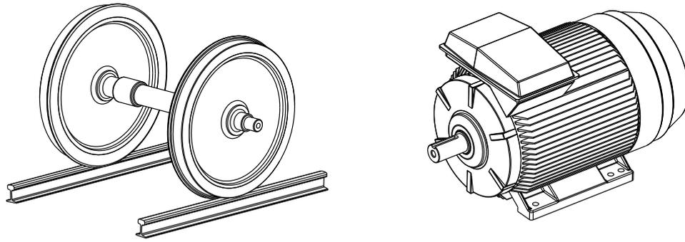
Fig. 2.1 Examples of rigid rotors
