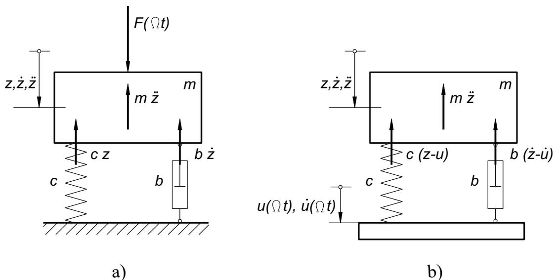
*Fig. 1.12 Oscillatory system with translational movement and one degree of freedom:
