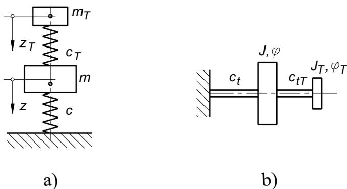
Fig. 2.6 Principle of the absorption of vibrations
