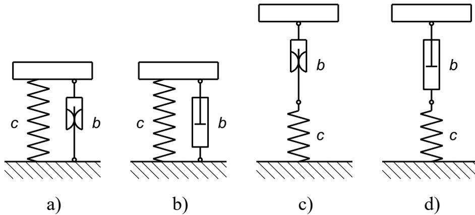
Fig. 1.7 Mechanical models with dampers:
