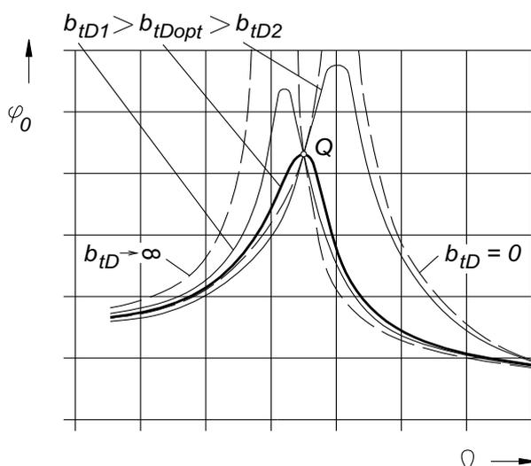
Fig. 2.12 Amplitude of oscillations of a damped rotor with a damper without elastic coupling
