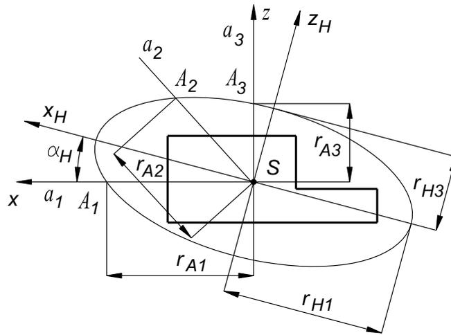
*Fig. 1.2 Determination of the main moments of inertia and their axes*
