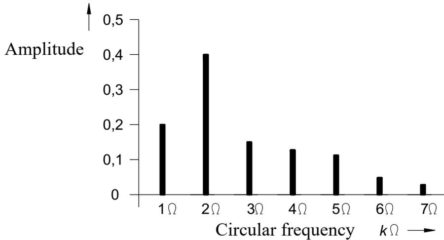
Fig. 1.10 Frequency spectrum of the periodic excitation
