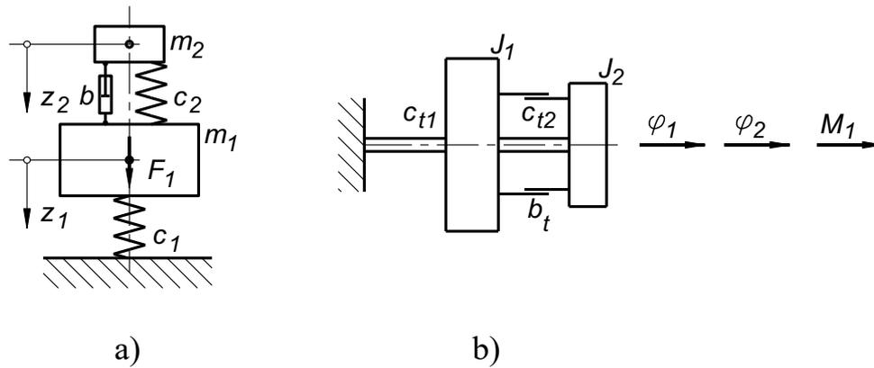
*Fig. 1.19* Partially damped dual-mass dynamic systems:
