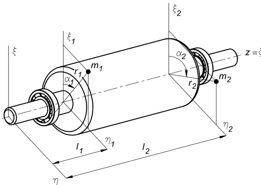
Fig. 2.4 Balancing in two planes
