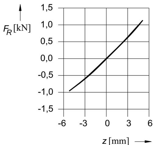
Fig. 1.4 Characteristics of air springs at an amplitude of 5 mm and  $\Omega = 10\text{Hz}$
