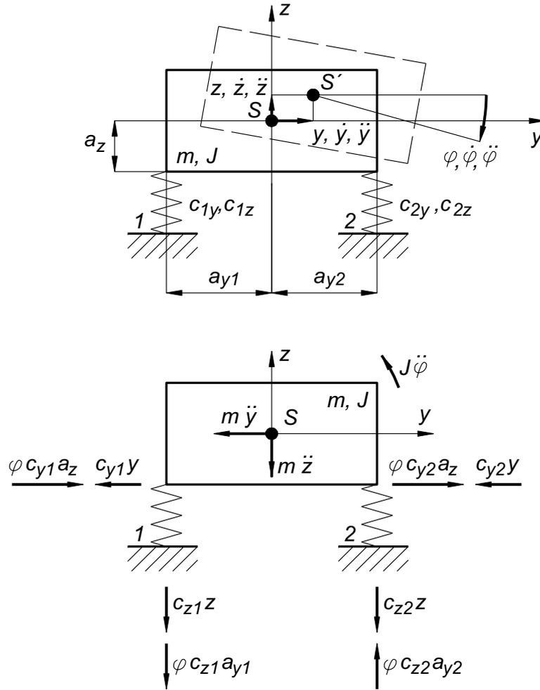
Fig. 1.17 Single-mass model with three degrees of freedom
