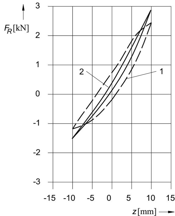
Fig. 1.3 Characteristics of air springs at an amplitude of 10 mm:
