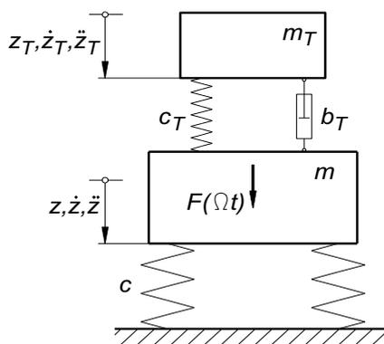
Fig. 2.7 Vibration absorber with a low damping
