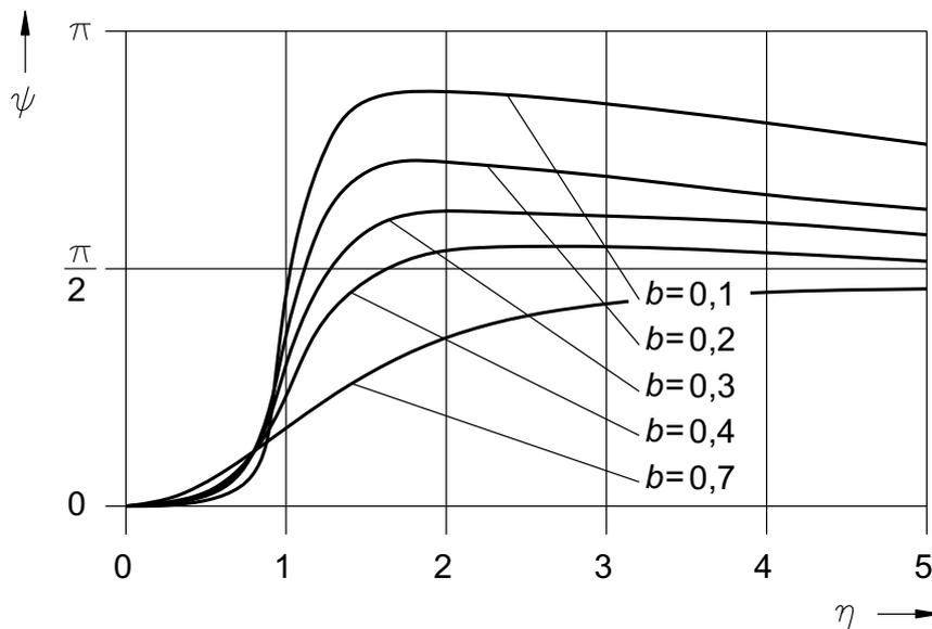
Fig. 1.16 Phase characteristic in kinematic excitation
