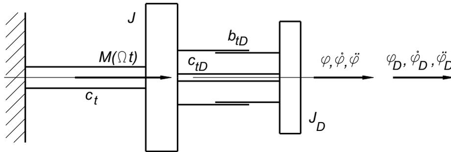
Fig. 2.9 Torsional vibration damper
