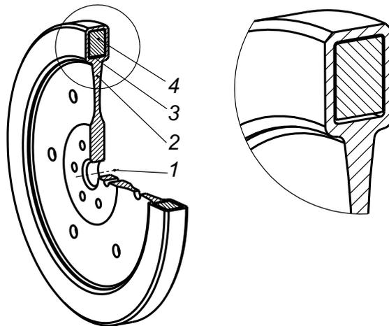
*Fig.2.13 Design of damped rotor with a damper without elastic coupling:
