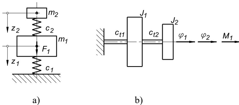
*Fig. 1.18 Undamped dual-mass dynamic system:
