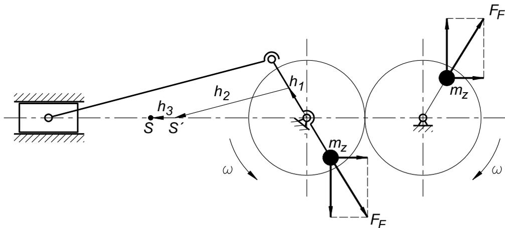
Fig. 2.5 Balancing by means of an additional shaft
