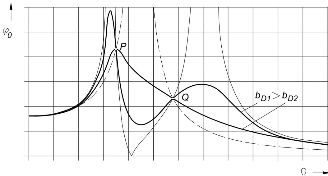
Fig. 2.10 Amplitude characteristic of a damped rotor
