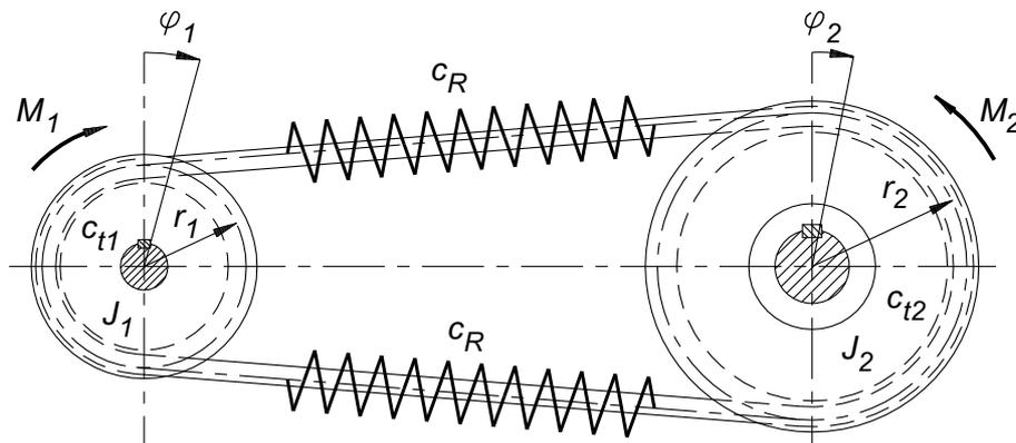
Fig. 1.6 Torsional rigidity of pulleys
