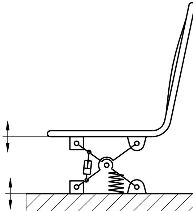
*Fig. 3.4* Suspension driver's seat with a guide mechanism
