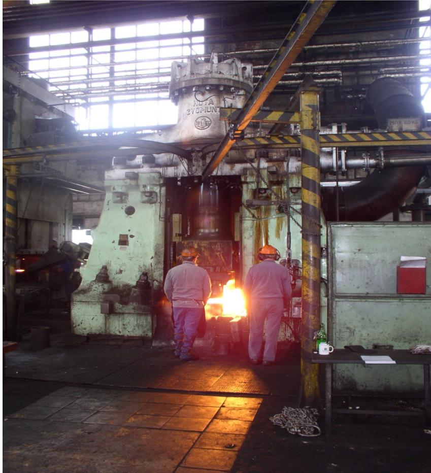
Fig. 3.7 Forging hammer
