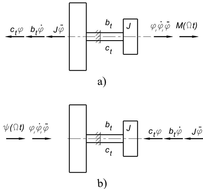
*Fig. 1.13 Oscillatory system with rotational movement and one degree of freedom:
