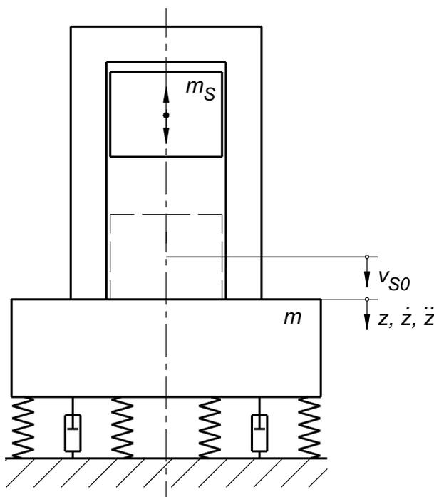
*Fig. 3.8 Mechanical model of the spring-mounted forging hammer*
