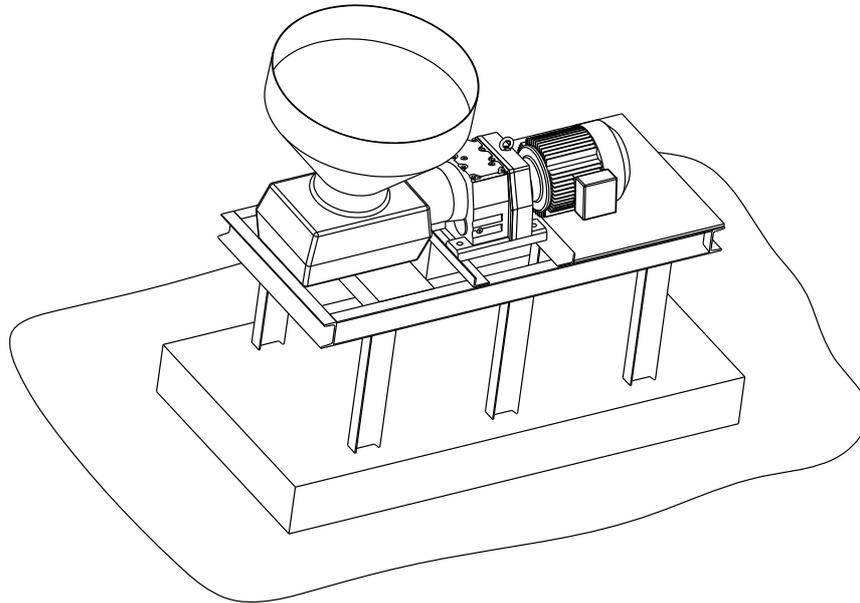
*Fig. 3.2 Setting of machine onto a frame structure*
