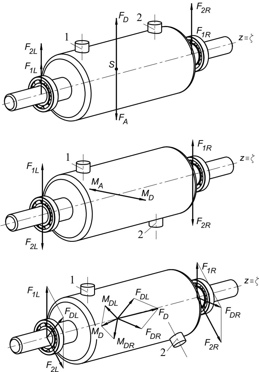
*Fig. 2.3 Rotor balancing*
