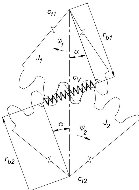
Fig. 1.5 Elastic coupling of gears
