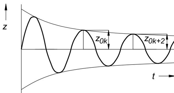
Fig. 1.8 Determination of the damping coefficient using the logarithmic decrement
