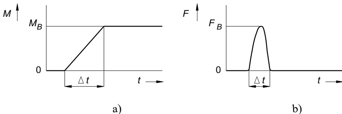
Fig. 1.11 Non-periodic excitation: a) ramp function, b) impact function
