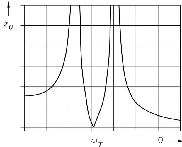
Fig. 2.8 *Waveform of the amplitude of oscillations of an object with a vibration absorber*
