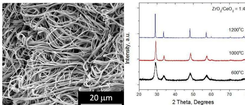
Figure 1. SEM image (left) and XRD patterns at different temperatures (right) of  $ZrO_2/CeO_2$  composite nanofibers with 1:4 molar ratio.
