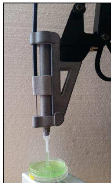
Figure 1. The pipette end effector
