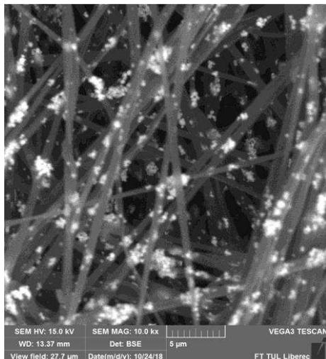
**Figure 1:** SEM image of electrospun PVB/ Bi<sub>2</sub>O<sub>3</sub> in ratio 1:1 (material contrast).
