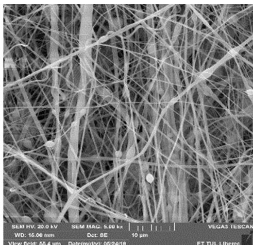
**Figure 1:** A sample of PVA nanofibers prepared from 12 wt.% precursor solution.
