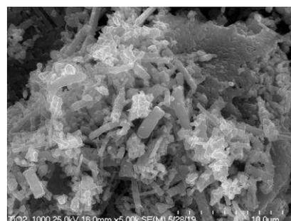
Figure 2: SEM analysis shows the crystalline structure of TiO<sub>2</sub> fibers annealed at 1000 °C in argon.
