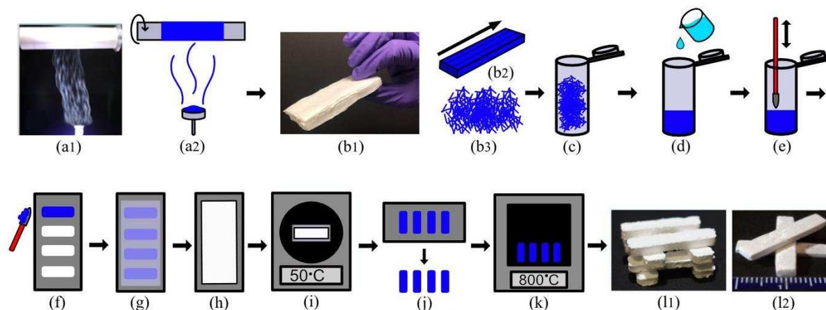
Figure 1: Process of making (3-D) glass-ceramic fibrous structures.
