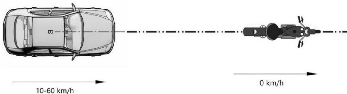
Obr. 46 Test nárazu do stojaceho motocykla (Car-to-Motorbike stationary – CMBs) [35]
