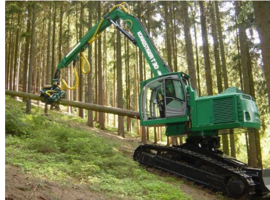
Fig. 4. Tracked harvester in main felling
