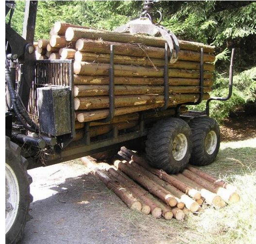
Fig. 63. By temporarily filling the ditch with logs, the harmless passage of machines into and out of the forest is enabled
