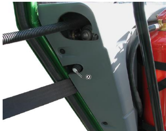
Fig. 67. Door safety switch (A)
