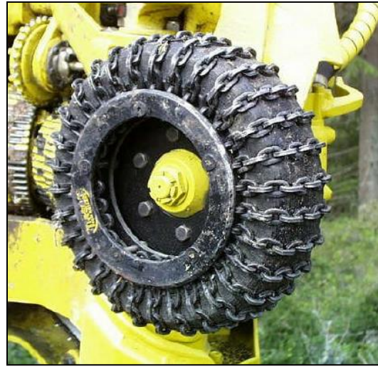
Fig. 32. Tyreco feed rollers with anti-slip chains
