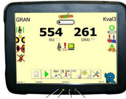
Fig. 50. Working mode of the touch display of Rottne D5 measuring and control system
