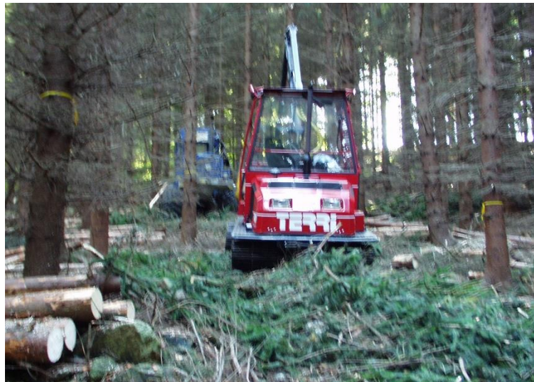
Fig. 64. Marking the marginal trees of the line with a tape is properly visible, the layer of logging residues on the line is sufficient to prevent disturbance of root system in marginal trees
