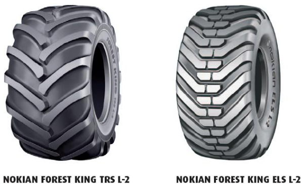
Fig. 16. Tyres with arrow pattern (TRS) and bent segments (ELS)
