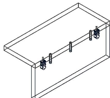
Fig. 1: 3D model of Cabineo with dowels
