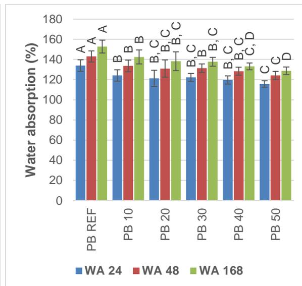
Fig. 2: Water absorption – same letter do not differ statistically by the Tukey's test ( $\alpha = 0.05$ ). Error bars represent standard deviation.
